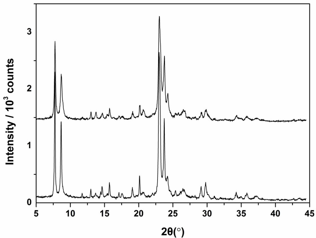
Figure S2. XRD patterns of as-made 8BI-MFI (bottom) and 10BI-MFI (top) zeolites synthesized at 175 °C and 150 °C with synthesis time of 9 and 10 days and water/silica ratio of 2.6 and 3.0, respectively.
