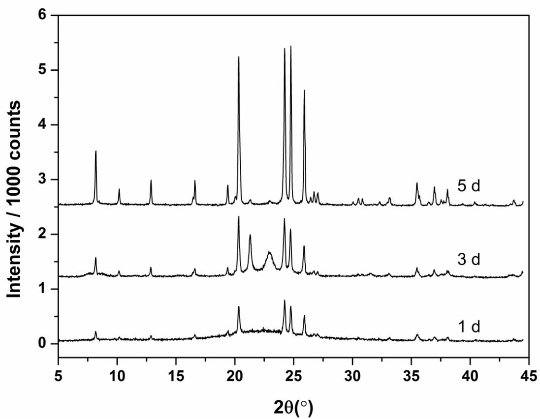
Figure S3. XRD patterns of as-made materials synthesized at different times with 8BI at 175 °C and a water/silica ratio of 8. The main phase obtained at 5 days is zeolite TON.
