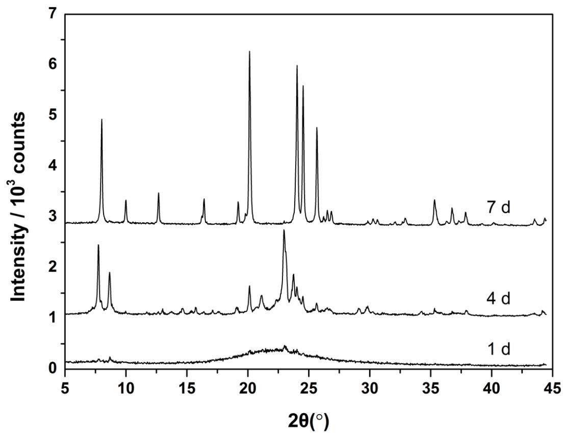
Figure S4. XRD patterns of as-made materials synthesized at different times with 10BI at 175 °C and a water/silica ratio of 8. The phase obtained at 7 days is zeolite TON.
