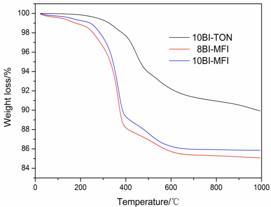
Figure S6. Thermogravimetric analysis of the as-made zeolites obtained in this work.
