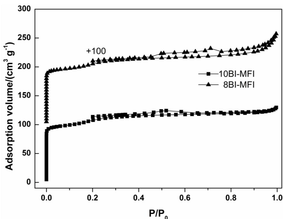
Figure S7. N<sub>2</sub> sorption isotherms of the calcined MFI zeolites.
