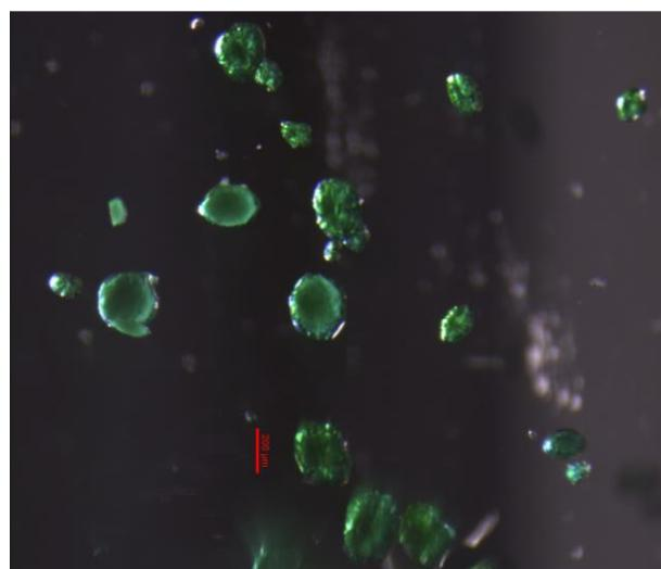
Figure S1. Light microscope image of **Cu-Sp5-EtOH** single crystals. Scale bar (in red): 200 μm
