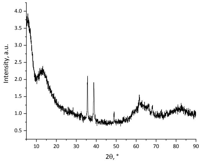
Figure S7. Powder pattern of the final product after **Cu-Sp5-EtOH** thermal decomposition in air. The broad peaks arise from the sample holder, while all the narrow peaks correspond to the copper (II) oxide.
