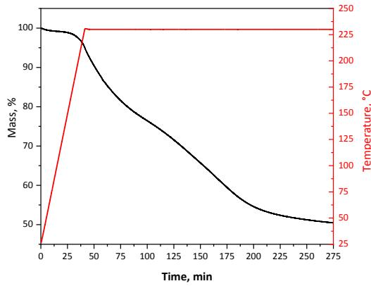
Figure S5. TGA curve for **Cu-Sp5-EtOH** in nitrogen atmosphere with the following program: 5°C/min until 230 °C, hold at 230 C. *The abscissa represents time in minutes.*
