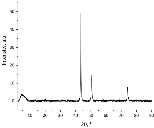
Figure S6. Powder pattern of the final product after **Cu-Sp5-EtOH** treatment at 230 °C in nitrogen atmosphere. The feature below 10 ° is due to the sample holder specifics.
