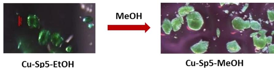
Figure S8. Light microscope images indicating the change in crystal size during transformation of **Cu-Sp5-EtOH** to **Cu-Sp5-MeOH** upon methanol soaking
