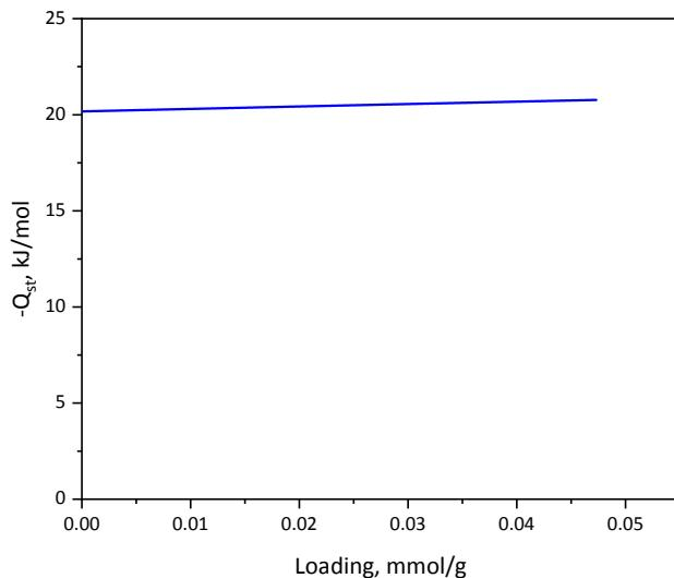
Figure S11. Isosteric heat of N<sub>2</sub> adsorption for Cu-Sp5.
