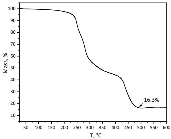
Figure S4. TGA curve for **Cu-Sp5-EtOH** in air. Heating rate: 5 °C/min.
