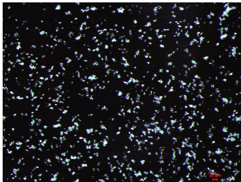
Figure S9. Light microscope image of **Cu-Sp5-MeOH**. Scale bar (in red): 20  $\mu\text{m}$
