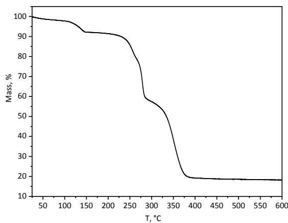
Figure S10. TGA curve for **Cu-Sp5-MeOH** in air. Heating rate: 5  $^{\circ}\text{C}/\text{min}$ .
