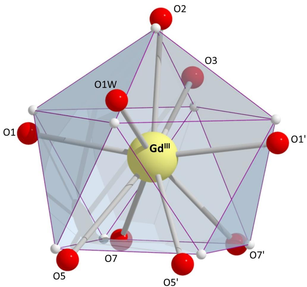
**Fig. S9** The spherical capped square antiprismatic coordination polyhedron of Gd<sup>III</sup> in complex **5**·MeCN. The smaller cream spheres define the vertices of the ideal polyhedron. Symmetry operation used to generate equivalent atoms: (')  $x, -y+1/2, z$ .
