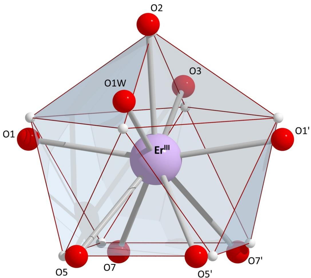
**Fig. S10** The spherical capped square antiprismatic coordination polyhedron of  $\text{Er}^{\text{III}}$  in complex  $9 \cdot \text{MeCN}$ . The smaller cream spheres define the vertices of the ideal polyhedron. Symmetry operation used to generate equivalent atoms: ( $'$ )  $x, -y+1/2, z$ .
