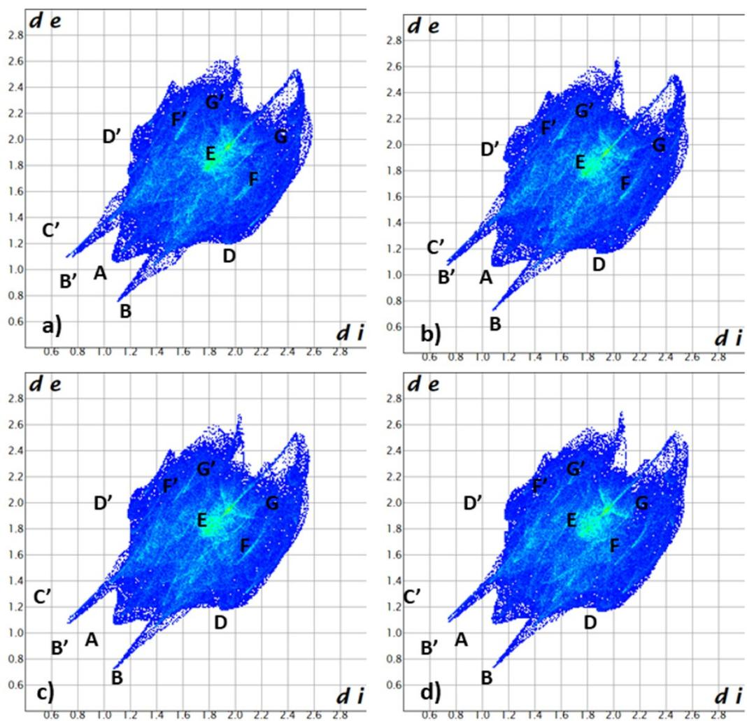
**Fig. S12** FP plots for all types of interactions in the crystal structures of (a) 1·MeCN, (b) 3·MeCN, (c) 5·MeCN and (d) 9·MeCN. Symbols B, D, F and G indicate acceptor point contributions for the O···H, Br···H, N···O and Br···O interactions, respectively, while B', D', F' and G' stand for the corresponding donor points. C', A and E correspond to the H···N, H···H and C···C interactions, respectively.
