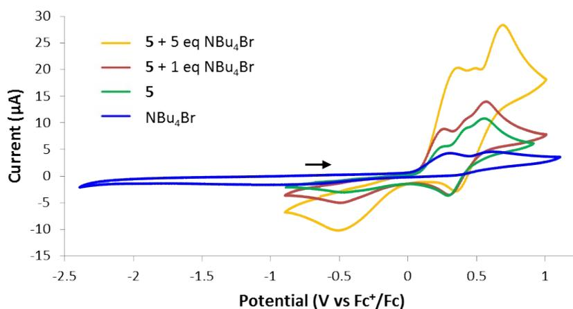
**Figure S16.** Cyclic voltammogram of compound **5**<sup>1</sup> with additional  $\text{NBu}_4\text{Br}$  (ca. 1.50 mM solution of complex in 1,2-dichloroethane; 0.1 M  $[\text{Bu}_4\text{N}][\text{PF}_6]$  electrolyte; scan rate  $0.1 \text{ V}\cdot\text{s}^{-1}$ ).
