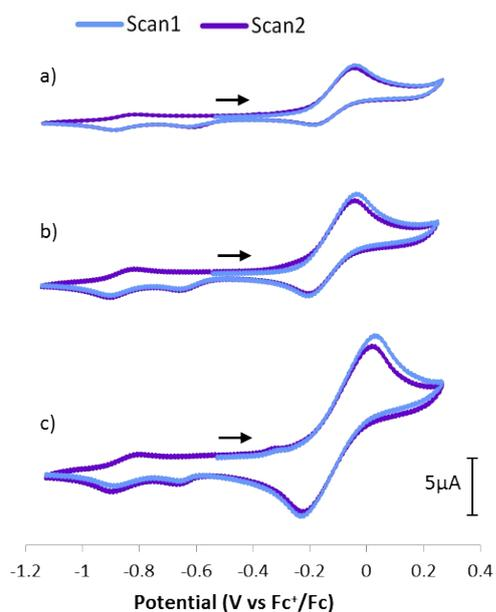
**Figure S12.** Cyclic voltammogram of compounds **4** (ca. 1.50 mM solution of complex in THF; 0.1 M  $[\text{Bu}_4\text{N}][\text{PF}_6]$  electrolyte, scan rate: a)  $0.05 \text{ V}\cdot\text{s}^{-1}$ , b)  $0.1 \text{ V}\cdot\text{s}^{-1}$ , c)  $0.3 \text{ V}\cdot\text{s}^{-1}$ ).
