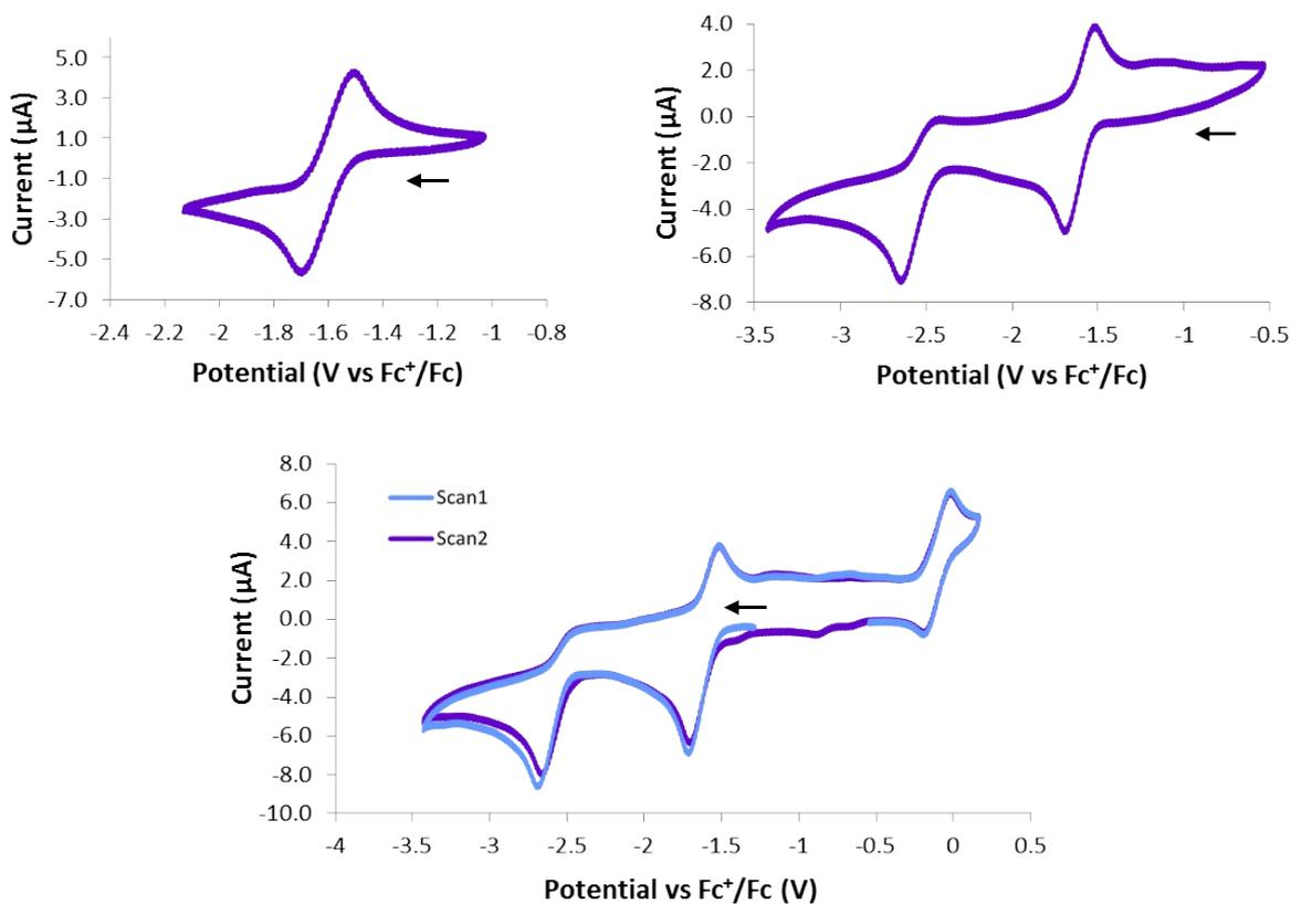
**Figure S11.** Cyclic voltammograms of compounds **4** (ca. 1.50 mM solution of complex in THF; 0.1 M  $[\text{Bu}_4\text{N}][\text{PF}_6]$  electrolyte; scan rate =  $0.1 \text{ V}\cdot\text{s}^{-1}$ ).
