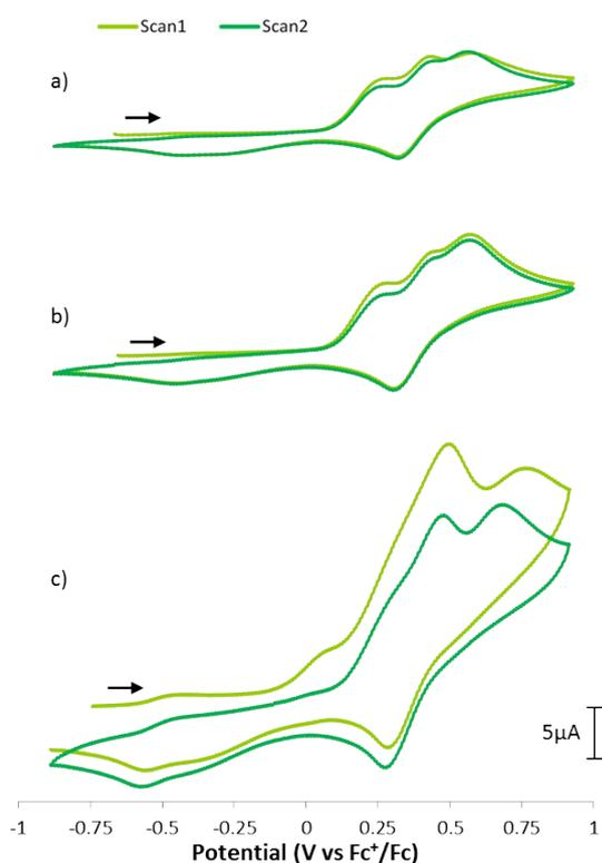
**Figure S15.** Cyclic voltammogram of compound **5** (ca. 1.50 mM solution of complex in 1,2-dichloroethane; 0.1 M  $[\text{Bu}_4\text{N}][\text{PF}_6]$  electrolyte; scan rate: a)  $0.05 \text{ V}\cdot\text{s}^{-1}$ , b)  $0.1 \text{ V}\cdot\text{s}^{-1}$ , c)  $0.5 \text{ V}\cdot\text{s}^{-1}$ ).
