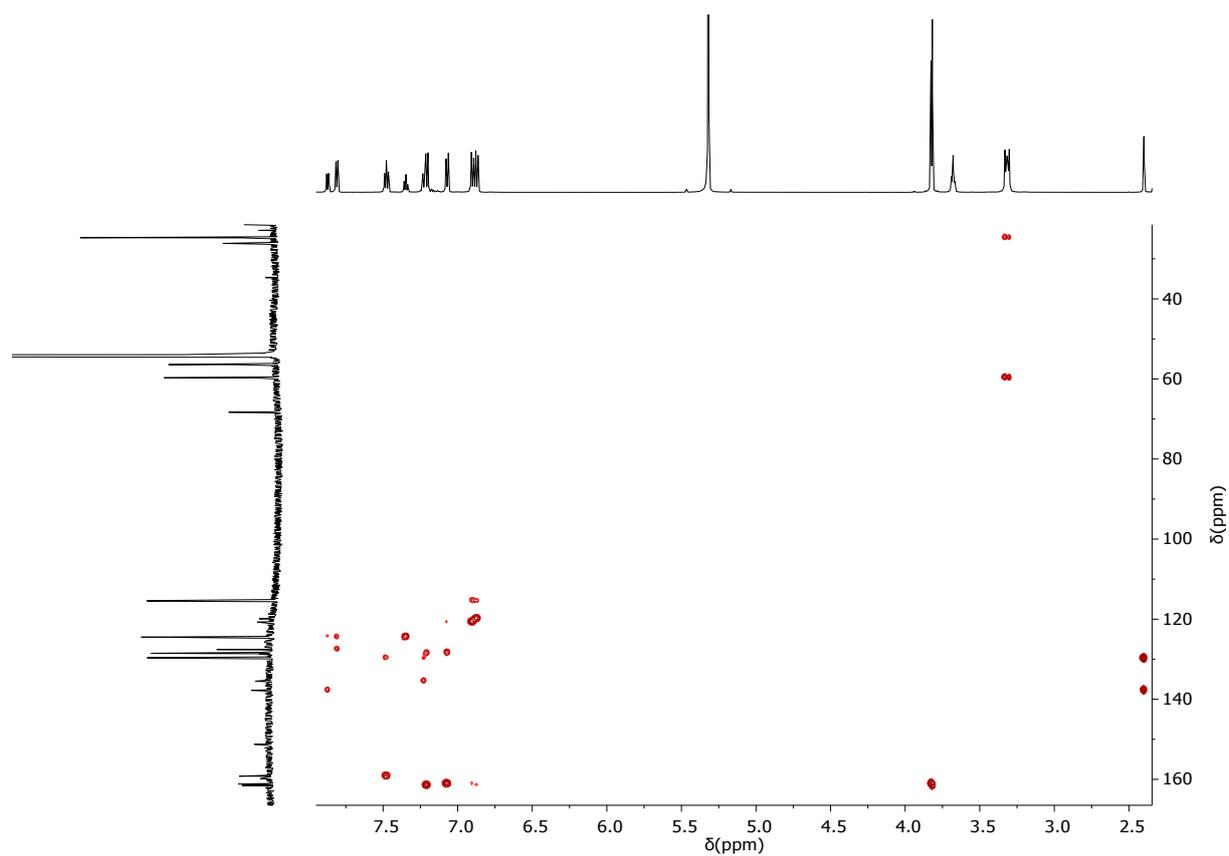
**Figure S6e.**  $^1\text{H}$ - $^{13}\text{C}$  gHMBC spectrum of **5** +  $\text{NBu}_4\text{Br}$  ( $\text{CD}_2\text{Cl}_2$ , 600 MHz, 25 °C).
