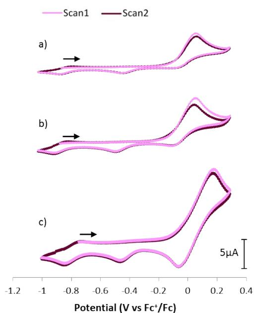
**Figure S10.** Cyclic voltammogram of compound **3** (ca. 1.50 mM solution of complex in THF; 0.1 M [Bu<sub>4</sub>N][PF<sub>6</sub>] electrolyte, scan rate: a) 0.05 V·s<sup>-1</sup>, b) 0.1 V·s<sup>-1</sup>, c) 0.5 V·s<sup>-1</sup>).
