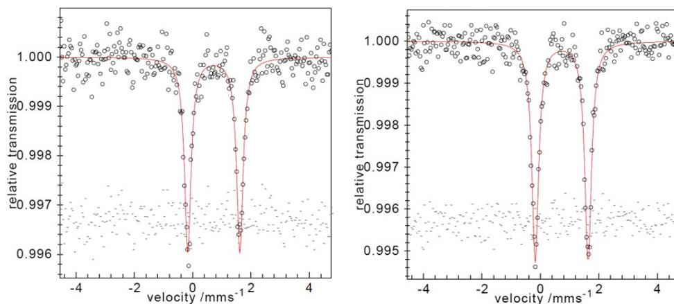
**Figure S2.** Zero-field Mössbauer spectra of solid **3** at 80 K (left; fit parameters are  $\delta = 0.73$   $\text{mm}\cdot\text{s}^{-1}$  and  $\Delta E_Q = 1.79$   $\text{mm}\cdot\text{s}^{-1}$ ) and at 7 K (right; fit parameters are  $\delta = 0.73$   $\text{mm}\cdot\text{s}^{-1}$  and  $\Delta E_Q = 1.81$   $\text{mm}\cdot\text{s}^{-1}$ ).
