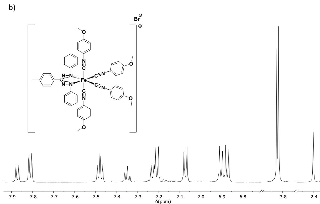
**Figure S6a.**  $^1\text{H}$  NMR spectrum of **5** +  $\text{NBu}_4\text{Br}$  ( $\text{CD}_2\text{Cl}_2$ , 600 MHz, 25 °C): a) full spectrum, b) selected peaks of **5**.
