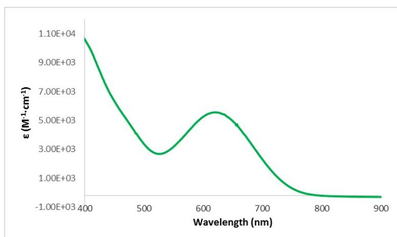
**Figure S18.** UV-Vis absorption spectrum of compound **5** in  $\text{CH}_2\text{Cl}_2$ .
