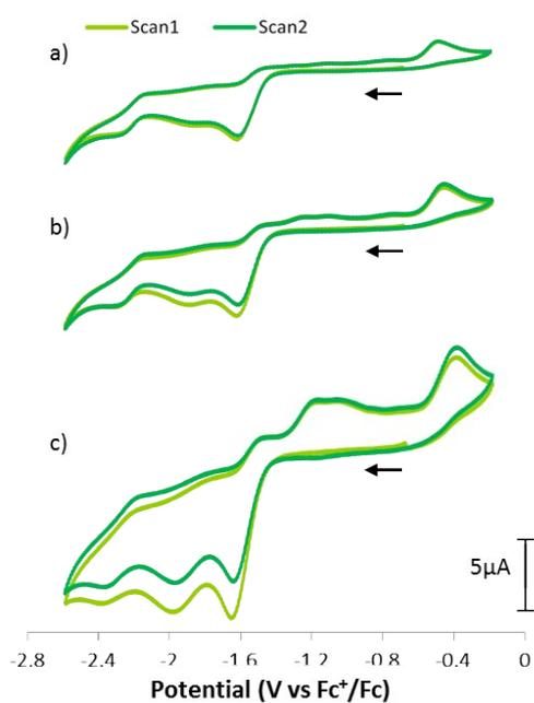
**Figure S13.** Cyclic voltammogram of compound **5** (ca. 1.50 mM solution of complex in 1,2-dichloroethane; 0.1 M  $[\text{Bu}_4\text{N}][\text{PF}_6]$  electrolyte; scan rate: a)  $0.05 \text{ V}\cdot\text{s}^{-1}$ , b)  $0.1 \text{ V}\cdot\text{s}^{-1}$ , c)  $0.5 \text{ V}\cdot\text{s}^{-1}$ ).
