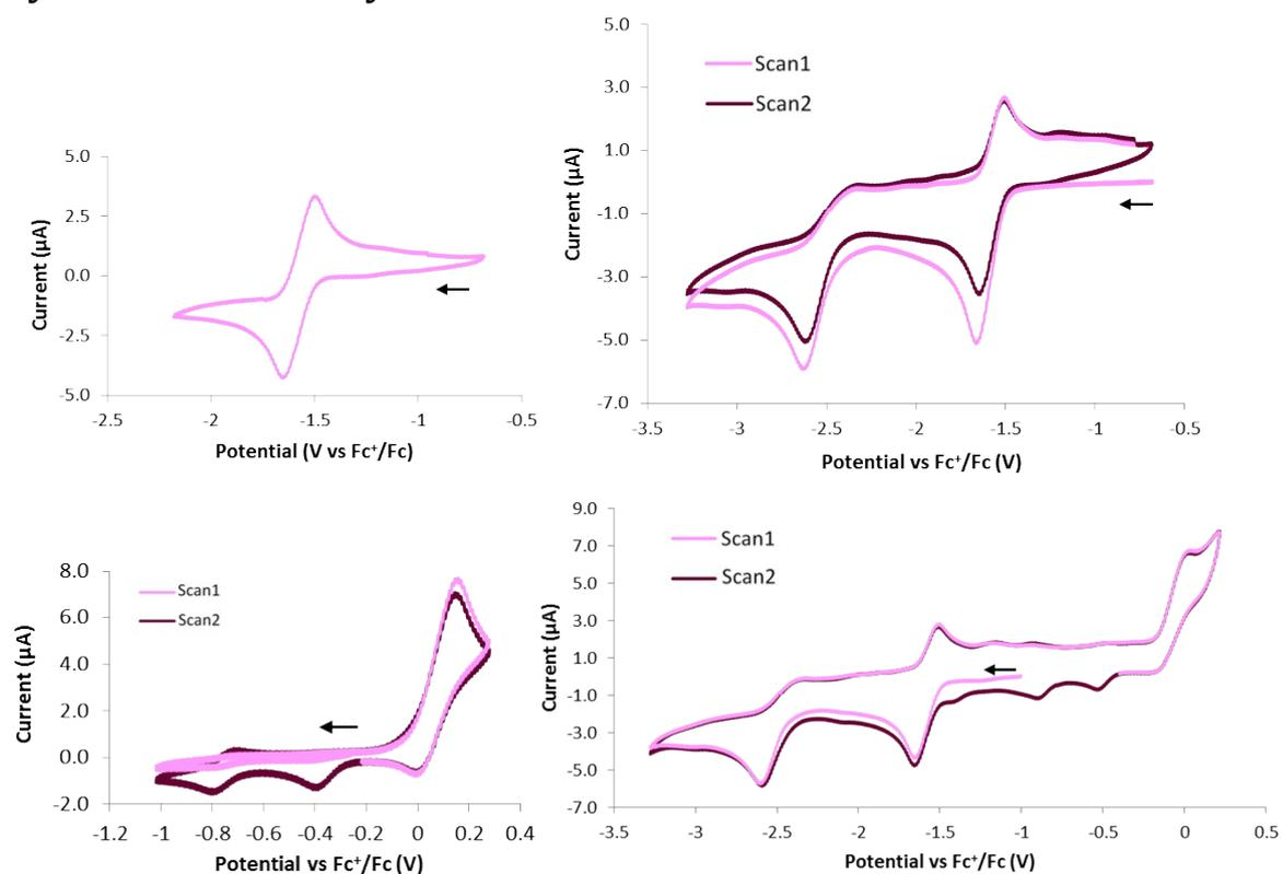
**Figure S9.** Cyclic voltammograms of compound **3** (ca. 1.50 mM solution of complex in THF; 0.1 M [Bu<sub>4</sub>N][PF<sub>6</sub>] electrolyte; scan rate = 0.1 V·s<sup>-1</sup>).
