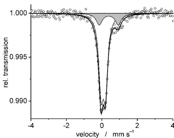
**Figure S3.** Zero-field Mössbauer spectrum of solid **5** at 80 K. Data is fit with two contributions: parameters for the major fraction (82%) are  $\delta = 0.08$   $\text{mm}\cdot\text{s}^{-1}$  and  $\Delta E_Q = 0.25$   $\text{mm}\cdot\text{s}^{-1}$ ; parameters for the minor fraction (18%) are  $\delta = 0.39$   $\text{mm}\cdot\text{s}^{-1}$  and  $\Delta E_Q = 1.07$   $\text{mm}\cdot\text{s}^{-1}$ .
