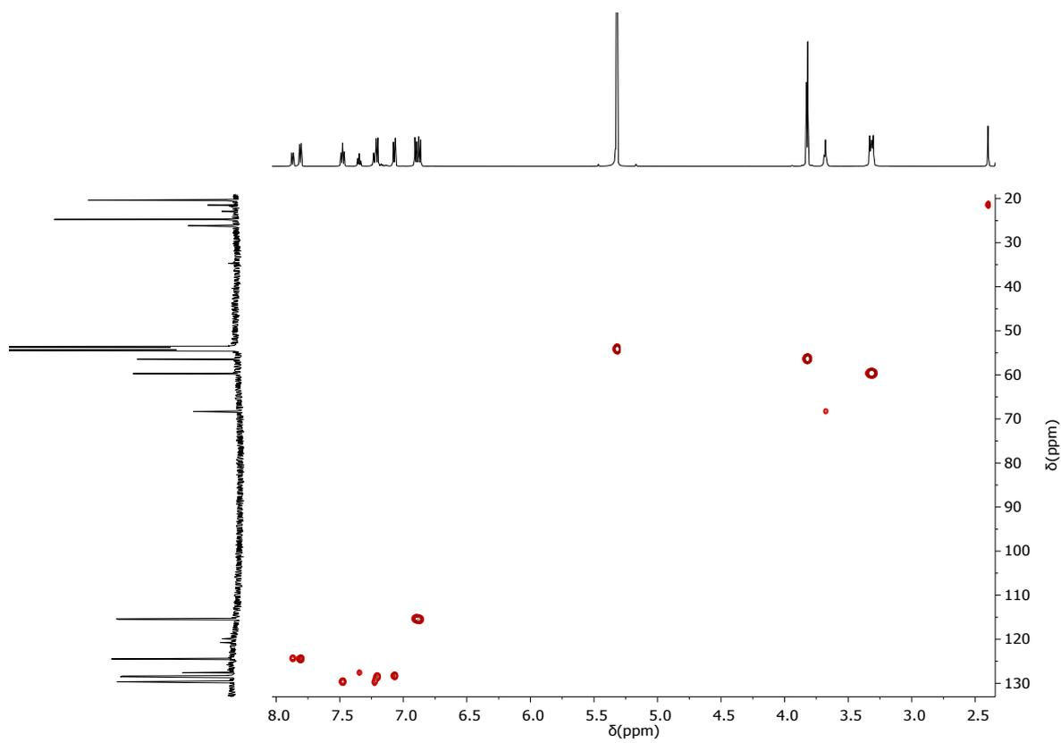
**Figure S6d.** <sup>1</sup>H-<sup>13</sup>C gHSQC spectrum of **5** + NBu<sub>4</sub>Br (CD<sub>2</sub>Cl<sub>2</sub>, 600 MHz, 25 °C).
