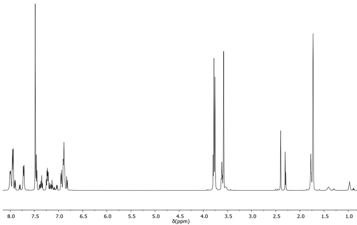
**Figure S6g.**  $^1\text{H}$  NMR spectrum of **5** +  $\text{NBu}_4\text{Br}$  ( $\text{THF-}d_8$ , 500 MHz, 25 °C).
