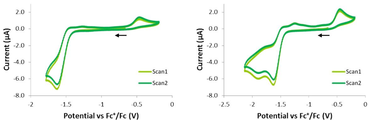
**Figure S14.** Cyclic voltammograms of compounds **5** (ca. 1.50 mM solution of complex in THF; 0.1 M  $[\text{Bu}_4\text{N}][\text{PF}_6]$  electrolyte; scan rate =  $0.1 \text{ V}\cdot\text{s}^{-1}$ ).
