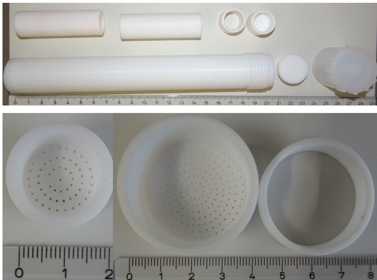
Figure S1 Top: Full autoclave set for MW-DGC with microwave tube, lid and screw-cap, three ring inlays for height-adjustment of sieve and DGC sieve, given also at bottom left in close-up view. Bottom right: Close-up view of a CE-DGC sieve with inlay ring for height adjustment.
