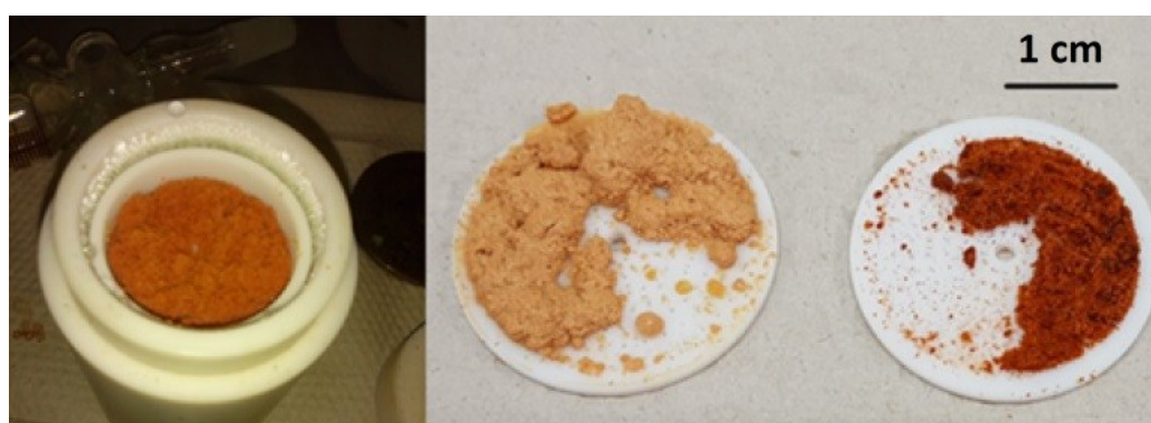
Figure S3 Left: Autoclave with DGC sieve, with MIL-100(Fe) product on top. Right: Products obtained from \text{Fe}(\text{NO}_3)_3 \cdot 9\text{H}_2\text{O} (left), \text{FeCl}_3 \cdot 6\text{H}_2\text{O} (right).
