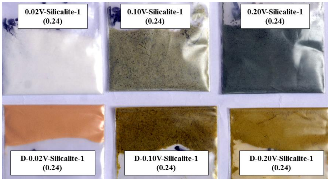
Fig. S5. Colors of the samples (before and after calcination) with different vanadium content in the system of 0.24 g NaOH.
