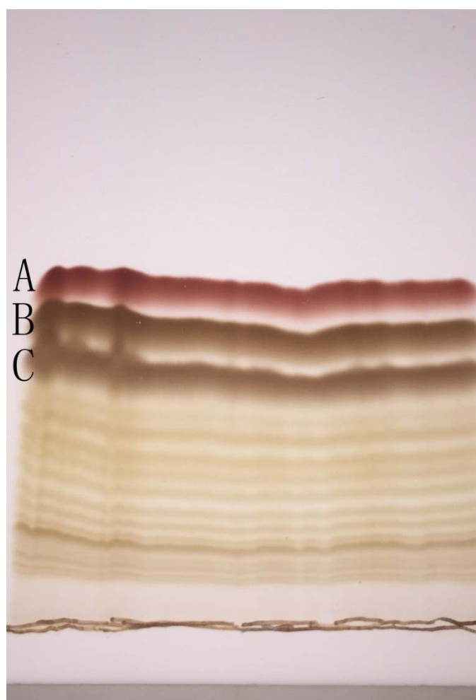
Fig. S1 PTLC of product A, B and C synthesized by one-pot method with n -propanol as solvent.
