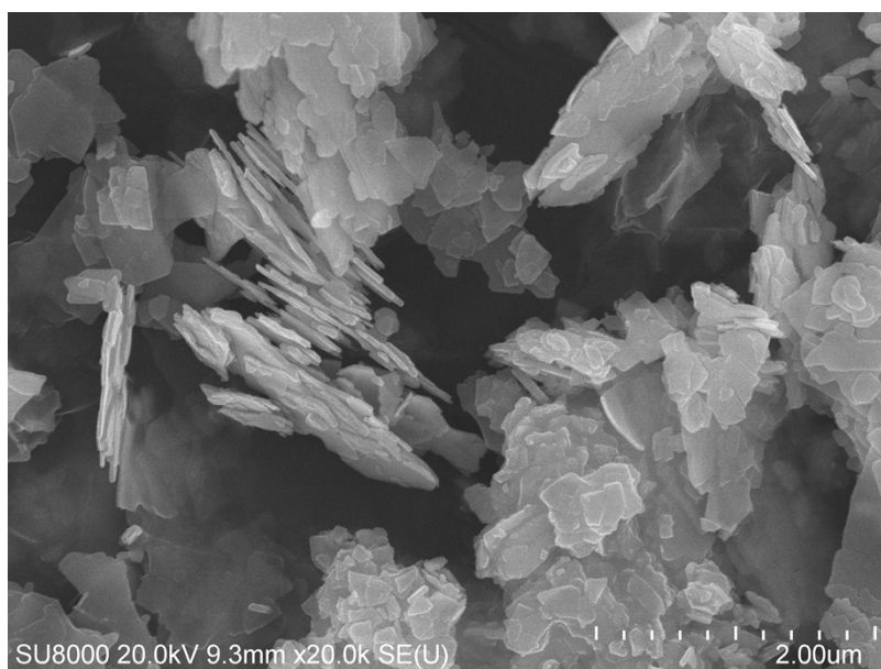
Fig. S9 The SEM micrograph of the hierarchical \text{WS}_2/\text{Bi}_2\text{MoO}_6 composite (5 wt% of \text{WS}_2 ) after the recycle experiments.
