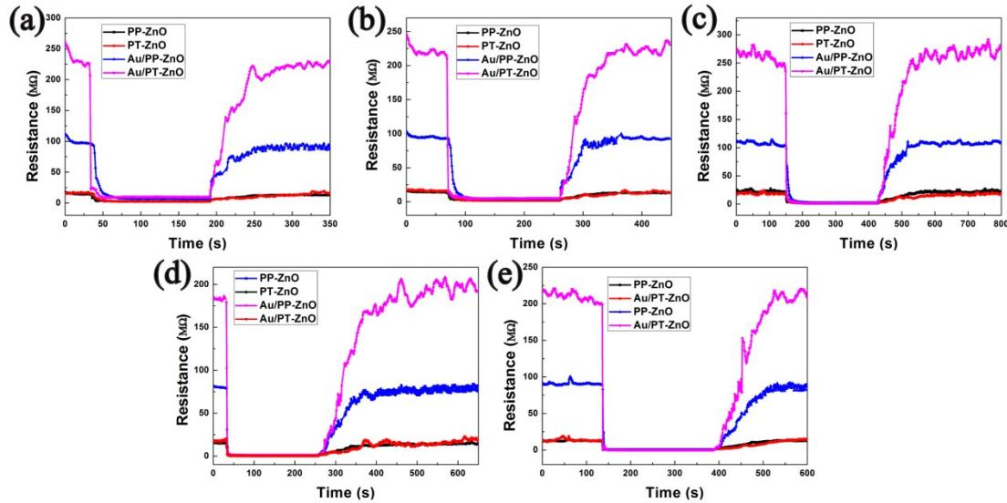
Fig. S2 Response-recovery curves to different acetone of these samples: (a) 12.5 ppm, (b) 25 ppm, (c) 50 ppm, (d) 100 ppm and (e) 200 ppm
