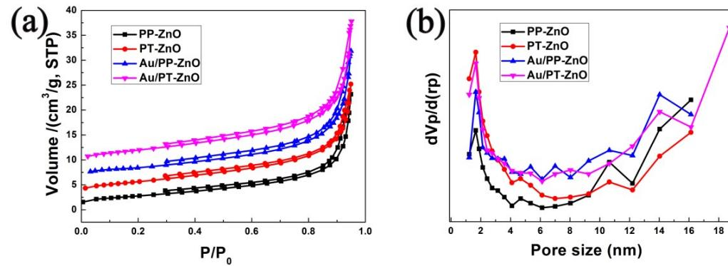
Fig. S1 (a) Nitrogen adsorption-desorption isotherms and (b) pore size distributions of PP-ZnO and PT-ZnO
