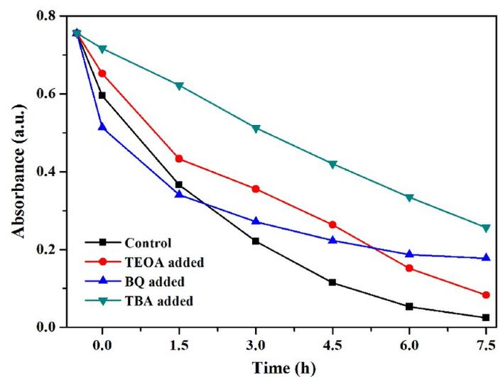
**Fig. S11** Effect of different trapping agents on degradation efficiencies of RhB aqueous solution ( $10 \text{ mg}\cdot\text{L}^{-1}$ ). Conditions: Tris (2-Hydroxyethyl) Amine (TEOA,  $0.5 \text{ mM}$ ), benzoquinone (BQ,  $0.5 \text{ mM}$ ) and tert-Butanol (TBA,  $0.5 \text{ mM}$ ).
