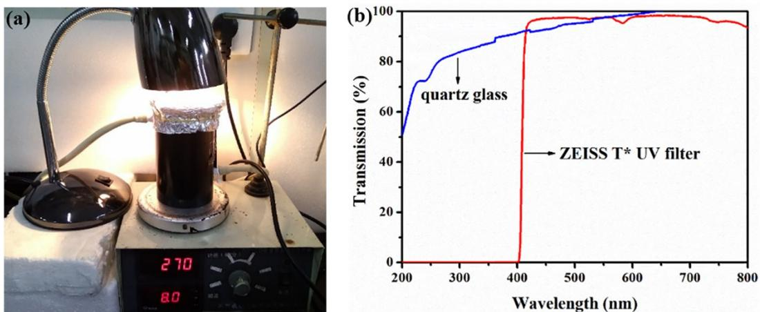
**Fig.S3** The photocatalytic reaction device under 40 W incandescent lamp (a), the transmittance test of quartz glass and ZEISS T\* UV filter under 200-800 wavelength (b).
