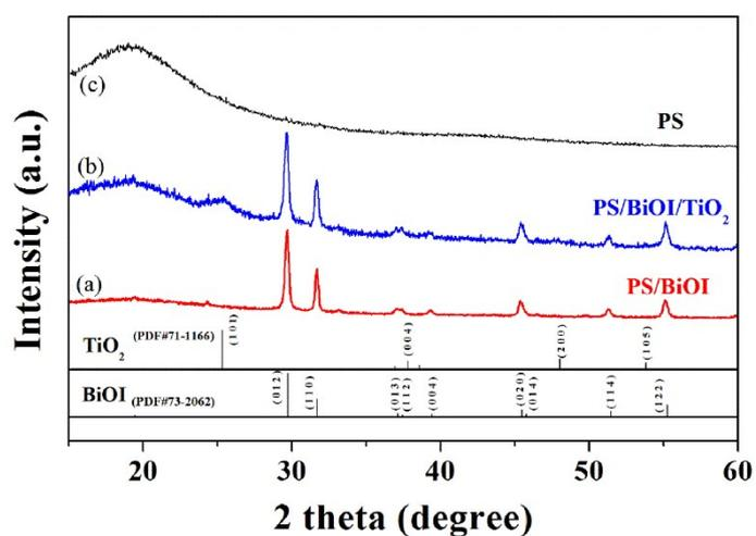
**Fig.S4** XRD patterns of PS/BiOI (a), PS/BiOI/TiO<sub>2</sub> (b) and PS (c).
