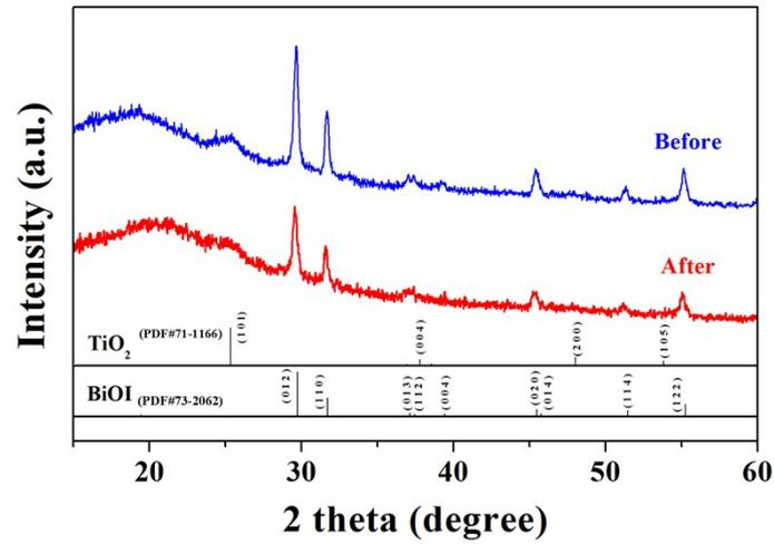
**Fig.S6** XRD patterns of the PS/BiOI/TiO<sub>2</sub> composite photocatalyst before and after the three cycles of photo-degradation.
