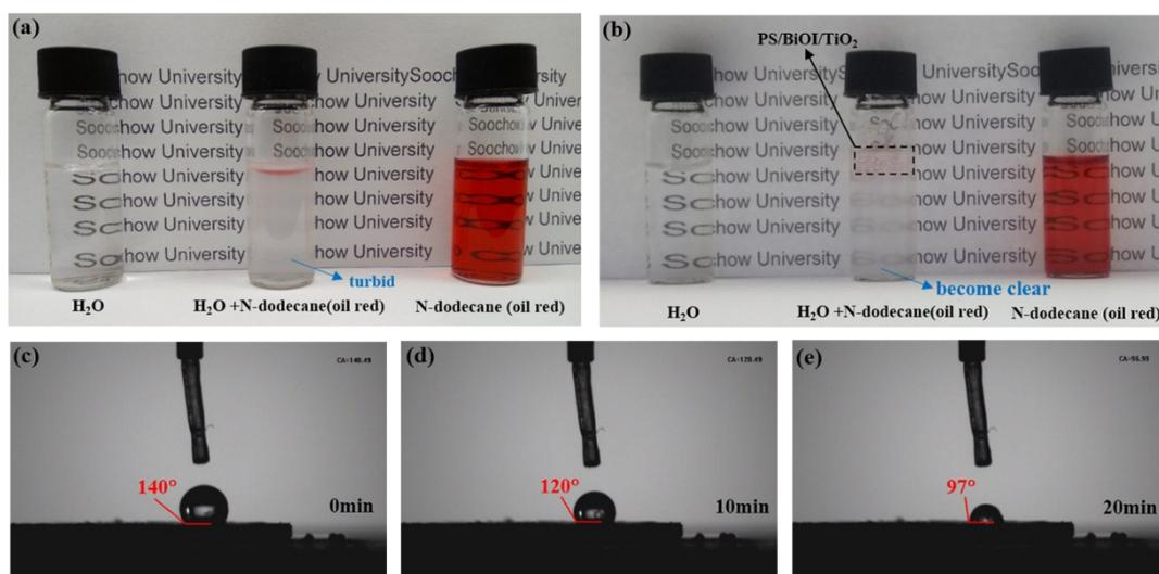
**Fig.S5** The experiment of oil-soluble dyes adsorption of PS/BiOI/TiO<sub>2</sub> (a-b), time-evolution of images for a water droplet absorbed by PS/BiOI/TiO<sub>2</sub> (c-e).
