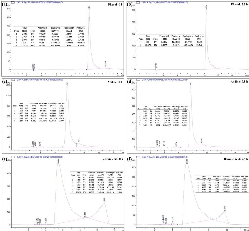
**Fig.S9** HPLC chromatograms recorded (a,c,e) before and (b,d,f) after a 7.5 h visible-light irradiation for the decomposition of several organic pollutants in presence of PS/BiOI/TiO<sub>2</sub> composite photocatalyst. (a,b) phenol, (c,d) aniline and (e,f) benzoic acid.
