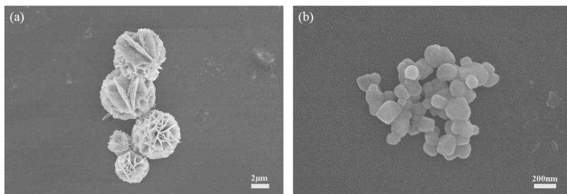
**Fig.S2** SEM images of BiOI (R1) (a) and TiO<sub>2</sub> (R2) (b).
