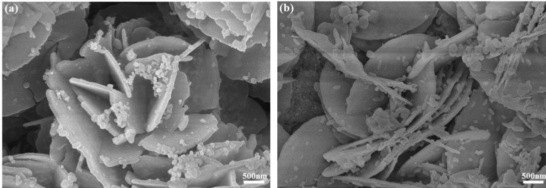
**Fig.S7** SEM images of the PS/BiOI/TiO<sub>2</sub> composite photocatalyst before (a) and after (b) the three cycles of photo-degradation.
