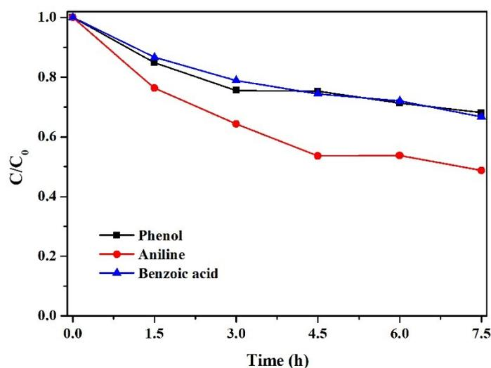
**Fig.S8** Concentration variation of several organic pollutants under visible-light irradiation in presence of PS/BiOI/TiO<sub>2</sub> composite photocatalyst.
