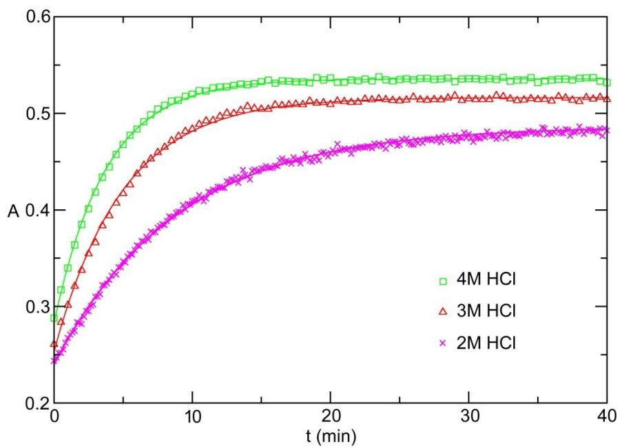
**Figure S8.** Kinetic traces ( $37\text{ }^{\circ}\text{C}$ ) obtained for the dissociation of the  $[\text{Bi}(\text{DO3A})]$  complex ( $5\text{ }10^{-5}\text{ M}$ ) by recording the absorption at 308 nm at different proton concentrations.
