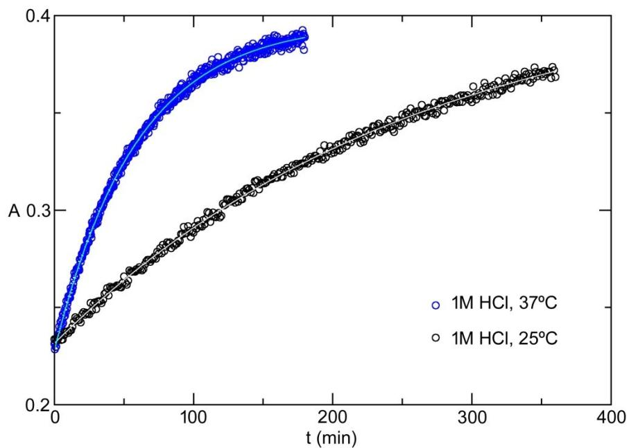
**Figure S9.** Kinetic traces obtained for the dissociation of the  $[\text{Bi}(\text{DO3A})]$  complex ( $5 \times 10^{-5}$  M) in 1 M HCl by recording the absorption at 308 nm at different temperatures.
