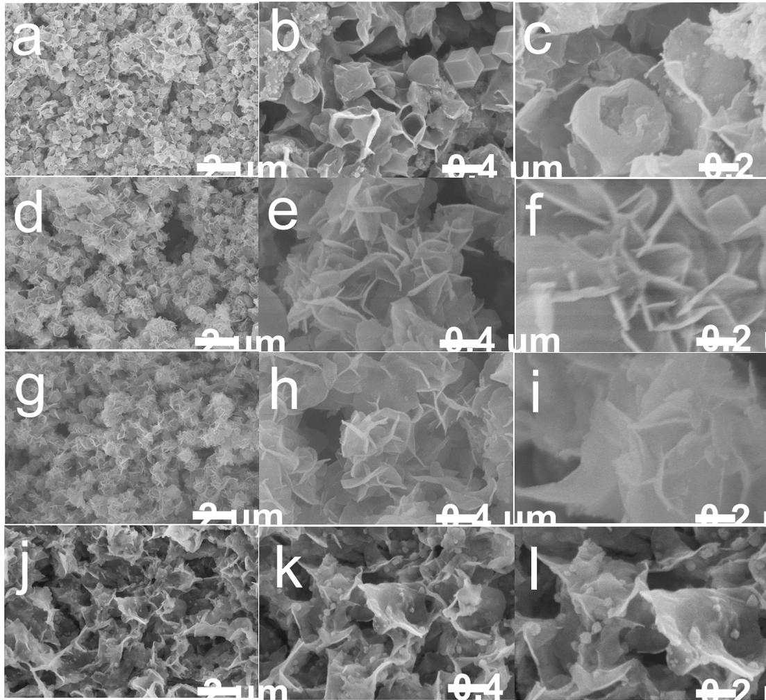
Figure S3 the SEM images of (a, b, c) obtained materials after etching 5 min; (d, e, f) etching 10 min; (g, h, i) etching 15 min; (j, k, l) etching 20 min;
