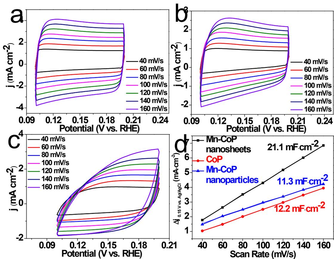
Figure S10 Voltammograms of the (a) Mn-CoP nanosheets; (b) hollow CoP, (c) Mn-CoP nanoparticles at various scan rates (40-160  $\text{mV s}^{-1}$ ); (d) Current difference ( $\Delta j$ ) plotted against the scan rate.
