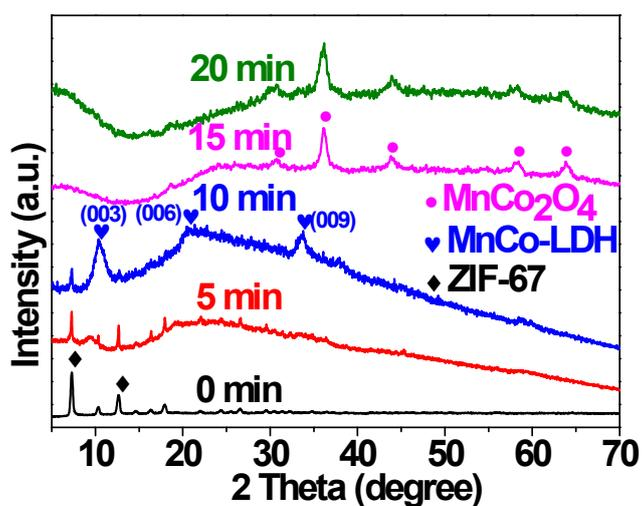
Figure S2. (a) XRD patterns of different etching time.
