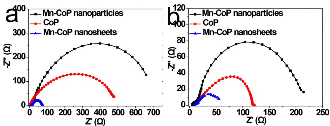
Figure S9 Nyquist plots of the as-synthesized Mn-CoP nanosheets, hollow CoP and Mn-CoP nanoparticles catalysts in (a) 0.5 M H<sub>2</sub>SO<sub>4</sub> with an overpotential of 165 mV vs. RHE and (b) 1 M KOH with an overpotential of 200 mV vs. RHE for HER.
