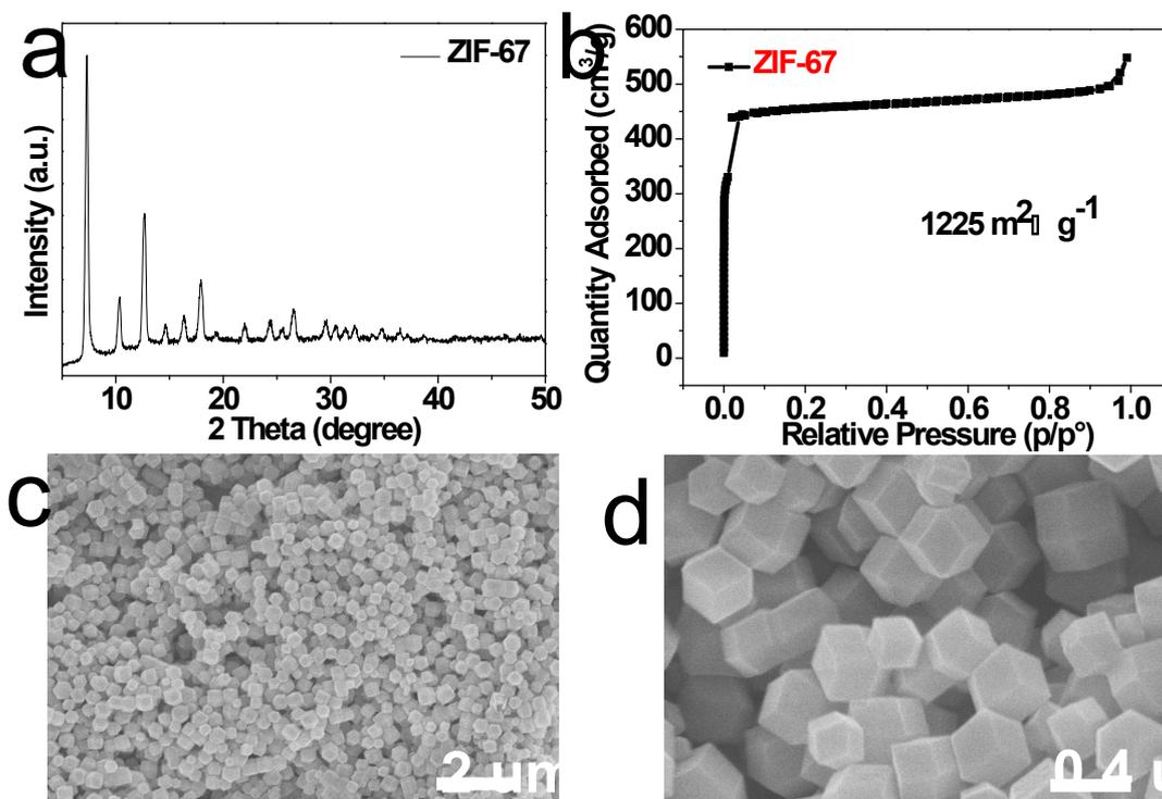
Figure S1. (a) XRD patterns of the as-synthesized ZIF-67; (b) N<sub>2</sub> adsorption-desorption isotherm of ZIF-67; (c and d) the SEM images of precursor ZIF-67
