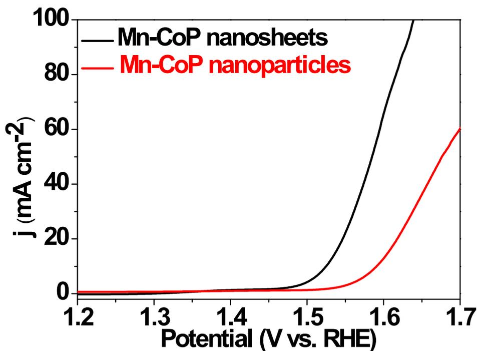
Figure S13 the LSV curves of the Mn-CoP nanosheets and Mn-CoP nanoparticles catalyst in 1 M KOH for OER.
