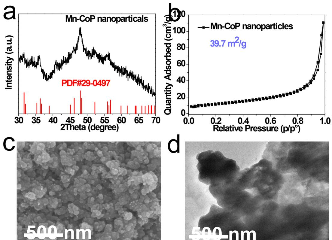
Figure S7 (a) The XRD of Mn-CoP nanoparticles; (b) N<sub>2</sub> sorption of Mn-CoP nanoparticles; (c-d) SEM of Mn-CoP nanoparticles
