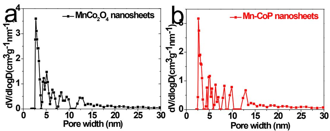
Figure S5 the pore size distributions of  $\text{MnCo}_2\text{O}_4$  and Mn-CoP nanosheets calculated by using NLDFT method.
