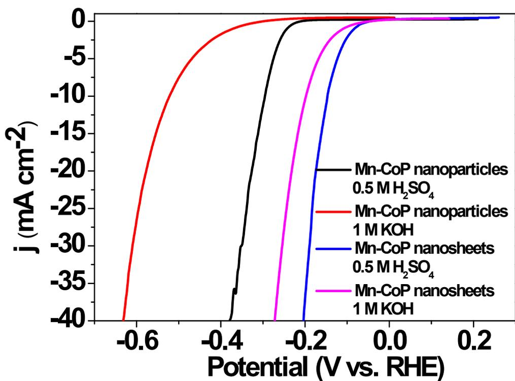
Figure S8 the HER performance of Mn-CoP nanoparticles and Mn-CoP nanosheets in 0.5 M H<sub>2</sub>SO<sub>4</sub> and 1 M KOH
