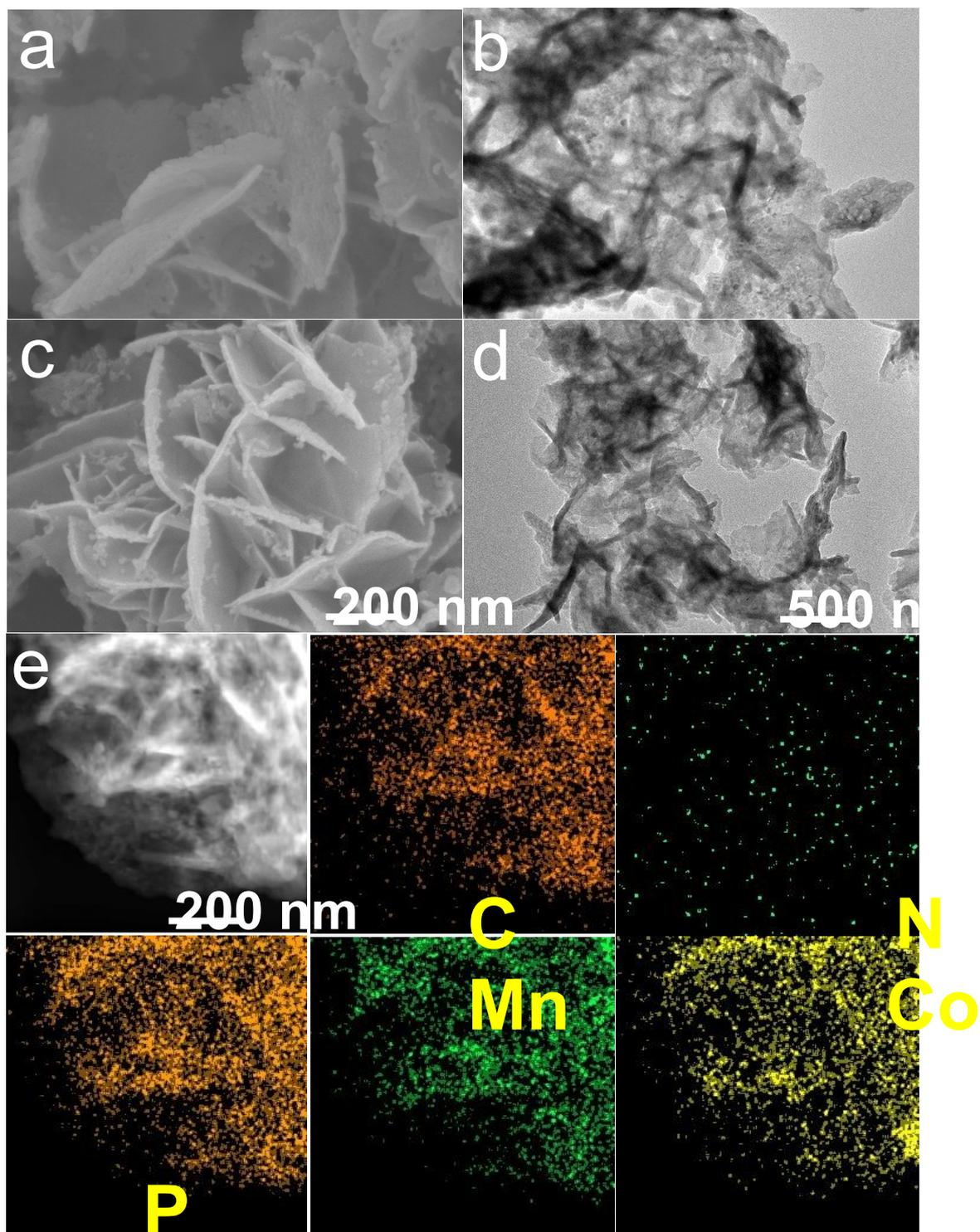
Figure S11 the SEM and TEM image of the Mn-CoP nanosheets catalyst after long term test in (a and b) 0.5 M H<sub>2</sub>SO<sub>4</sub> and (c and d) 1 M KOH for HER. (e) HAADF-STEM elemental mapping of the Mn-CoP nanosheets catalyst after long term test 0.5 M H<sub>2</sub>SO<sub>4</sub> solution .
