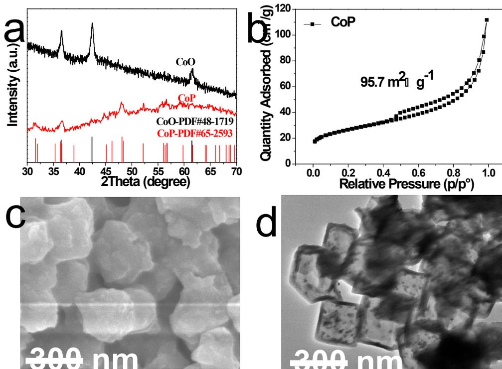
Figure S6 (a) The XRD of CoO and CoP nanoparticles; (b) N<sub>2</sub> sorption of hollow CoP; (c-d) SEM and TEM of hollow CoP nanoparticles
