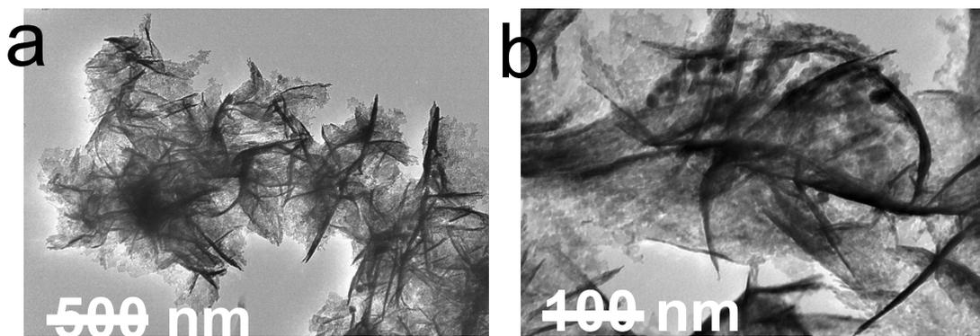
Figure S4 TEM images of  $\text{MnCo}_2\text{O}_4$  nanosheets
