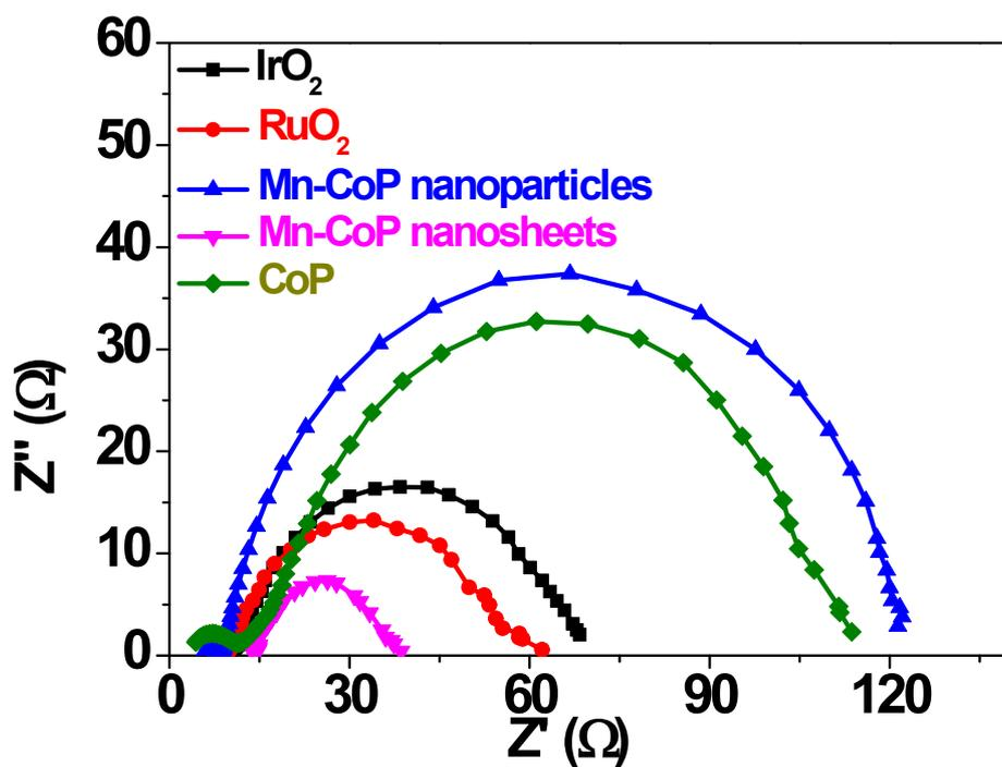
Figure S14 Nyquist plots of the as-synthesized catalysts in 1 M KOH with an overpotential of 320 mV vs. RHE for OER.
