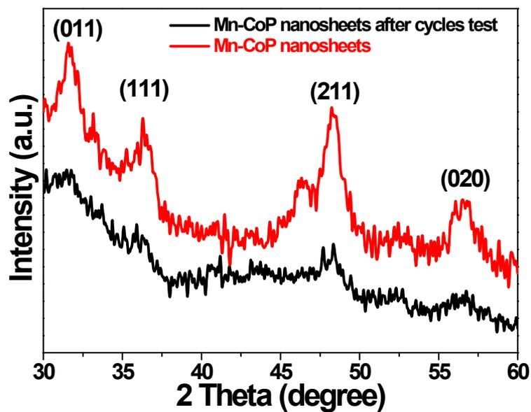
Figure S12 the XRD of Mn-CoP nanosheets before and after cycles tests
