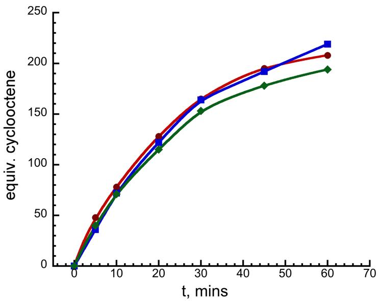
**Figure S12.** Comparative catalyst activity plot for  $(^{t\text{Bu},\text{CF}_3}\text{PCP})\text{Ru}(\text{nbd})\text{H}$  under 590 Torr of  $\text{N}_2$  (■), under vacuum (●), and with 100 equiv of added  $\text{H}_2\text{O}$  (◆) in 1:1 cyclooctane/*tert*-butylethylene at 200 °C (0.033 mol % catalyst loading).
