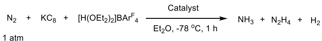
Catalytic reduction of dinitrogen into ammonia and hydrazine was carried out according to a method similar to the Peters' procedure.<sup>S11</sup> A typical experimental procedure using **2c** is described below.
