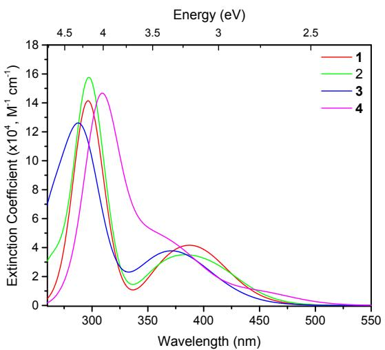
Fig. S4 Simulated UV-vis spectra for iridium complexes **1**, **2**, **3** and **4** at B3LYP/6-31g(d)/LANL2DZ level of theory with PCM in  $CH_2Cl_2$  medium. The curves are plotted using Gaussian broadening function with a full width at half-maximum of 0.4 eV.
