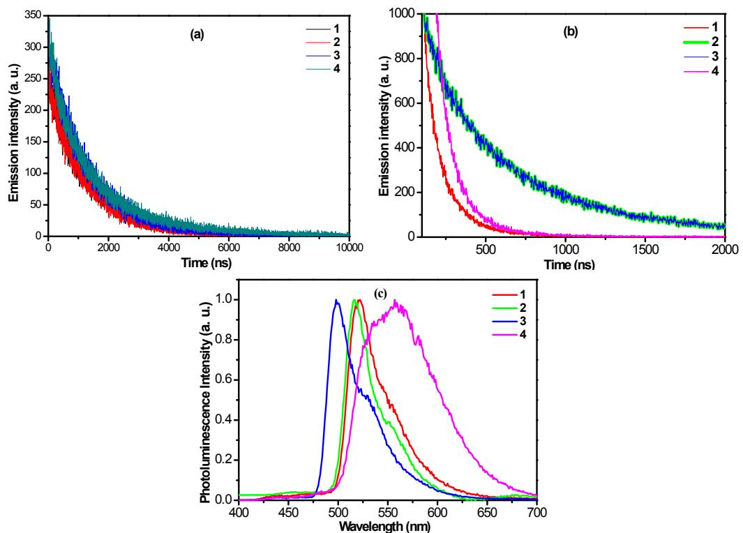
**Fig. S2.** Emission decay curves of iridium(III) complexes in PMMA (0.01 wt%) (a) and neat power (b). PL spectra of iridium complexes in PMMA (0.01 wt%) at temperatures of 77 K (c).
