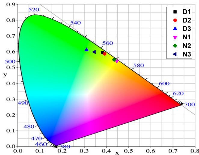
Fig. S6. CIE coordinates of EL devices **D1, D2, D3, N1, N2** and **N3**.
