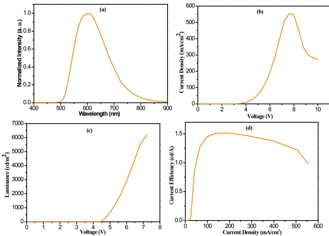
**Fig. S7.** The performance of non-doped OLEDs device based on complex 4. (a) EL spectra of device. (b) Current density-voltage characteristics. (c) Luminance-voltage characteristics. (d) Luminance efficiencies vs. current density.
