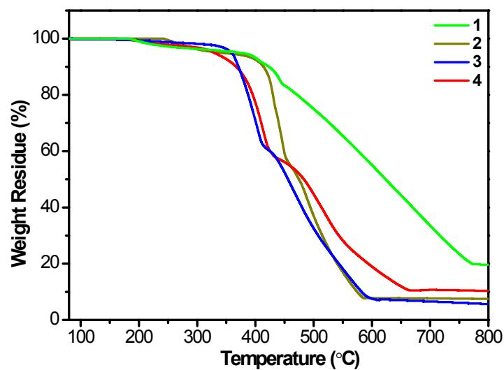
**Fig S1.** Thermal gravimetric spectra of iridium (III) complexes.
