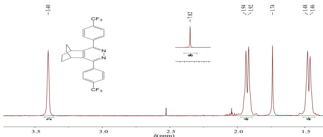
$^{19}\text{F}$ -NMR Spectrum of **L2** in  $\text{CDCl}_3$  (376 MHz):
