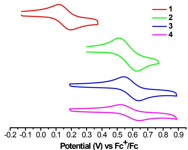
**Fig S3.** Cyclic voltammetry curves of iridium (III) complexes in  $\text{CH}_2\text{Cl}_2$ .
