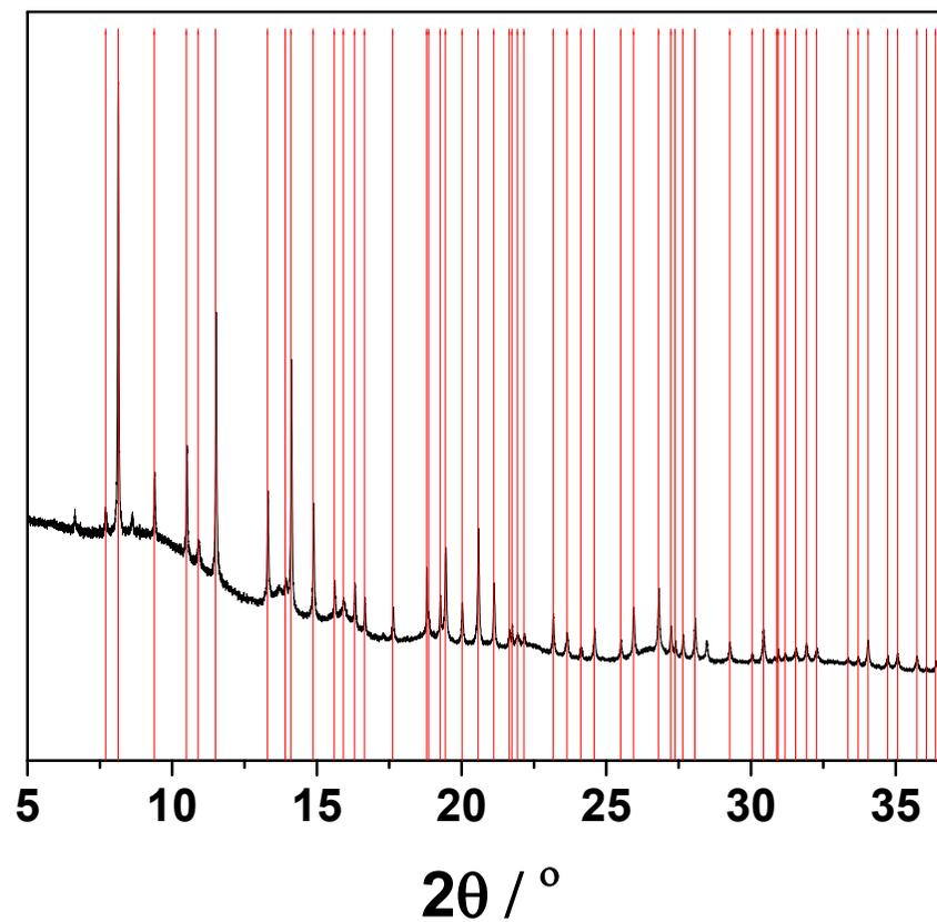
Figure S13 50% Li discharged  $\text{Sc}_2\text{W}_3\text{O}_{12}$  electrode at  $550^\circ\text{C}$  XRD pattern and extraction of peak positions.
