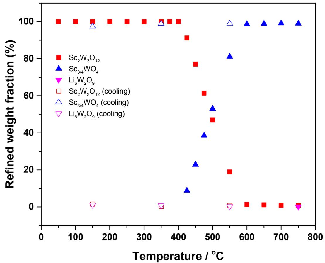
Figure S6 Refined weight fraction of phases during heating and cooling process for the thermal treatment of the 12.5% Li discharged  $\text{Sc}_2\text{W}_3\text{O}_{12}$  electrode
