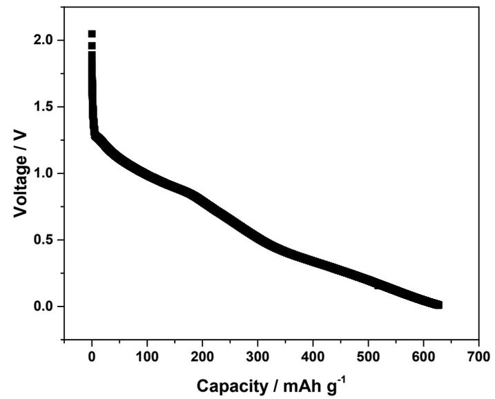
Figure S1 The full discharge curve of 100% Li discharged  $\text{Sc}_2\text{W}_3\text{O}_{12}$ . The recorded capacity was 627(1) mAh g<sup>-1</sup>.
