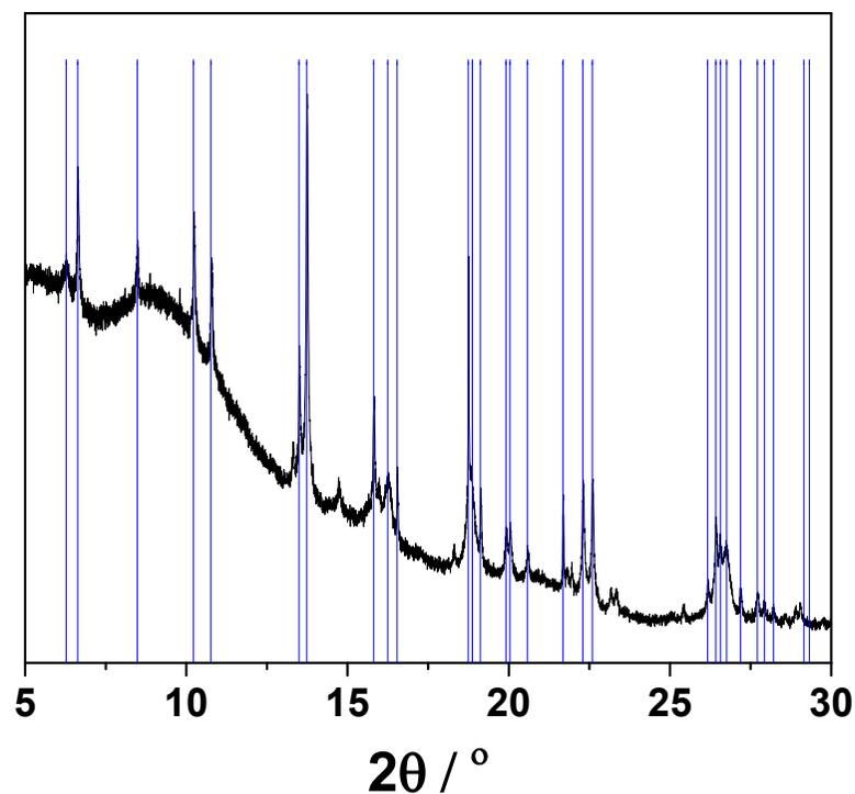
Figure S14 50% Li discharged  $Sc_2W_3O_{12}$  electrode at 700°C with extracted peak positions indicated.
