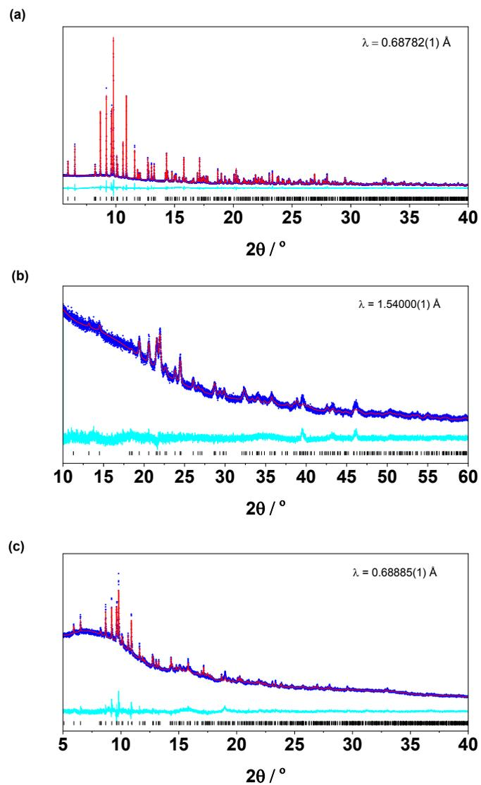
Figure S2 (a) 12.5% discharged Rietveld-refined  $\text{Sc}_2\text{W}_3\text{O}_{12}$  model with XRD data,  $wR=4.280\%$ . (b) 25% discharged Rietveld-refined model with XRD data,  $wR=4.034\%$ . (c) 50% discharged Rietveld-refined model with XRD data,  $wR=2.622\%$ . In (b-d) the data are represented as blue, the calculated model as red line and the difference between the data and model as the cyan curve below, the black points are  $\text{Sc}_2\text{W}_3\text{O}_{12}$  peak markers.
