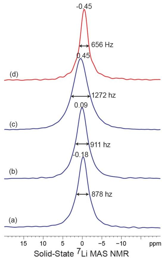
Figure S4 Solid-state  ${}^7\text{Li}$  MAS NMR of  $\text{Sc}_2\text{W}_3\text{O}_{12}$  electrodes discharged to (a) 12.5 %, (b) 25 % and (c) 50% of the full Li discharge capacity and (d) is the 25 % discharged  $\text{Sc}_2\text{W}_3\text{O}_{12}$  heat treated to 700 °C. The chemical shifts of the peak maxima in ppm and the peak full width at half maximum (FWHM) in Hz are indicated.
