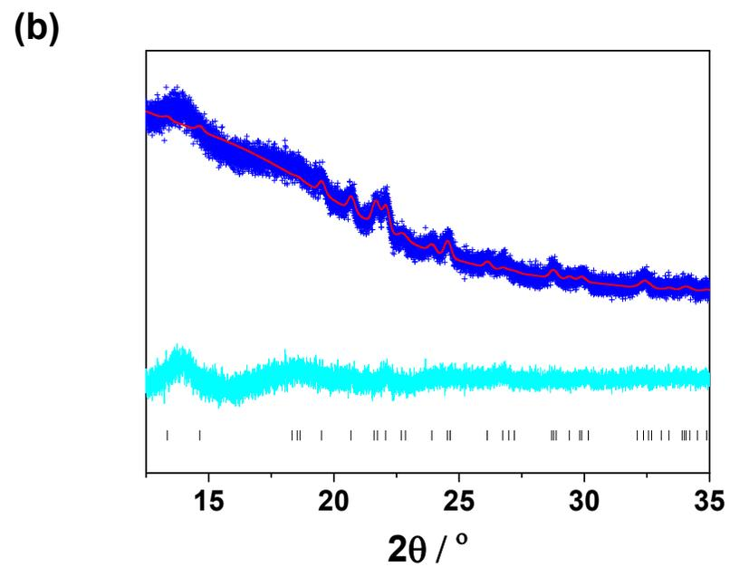
Figure S10 Thermal evolution of 25% discharged  $Sc_2W_3O_{12}$  electrode in PC-electrolyte without binder. (b) Rietveld refined fit of the  $Sc_2W_3O_{12}$  model with XRD data at 50°C,  $wR=4.081\%$ . In b, the data are represented as blue, the calculated model as red and the difference between the data and model as the cyan curve below, black are  $Sc_2W_3O_{12}$  peak markers. Please note these data were collected on the laboratory XRD.
