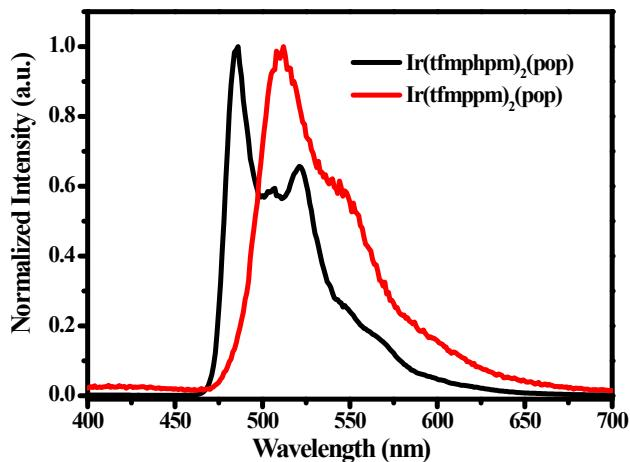
**Fig. S1.** Emission spectra of  $\text{Ir}(\text{tfmphpm})_2(\text{pop})$  and  $\text{Ir}(\text{tfmppm})_2(\text{pop})$  complexes in degassed  $\text{CH}_2\text{Cl}_2$  solutions ( $5.0 \times 10^{-5}$  mol L $^{-1}$ ) at 77 K.
