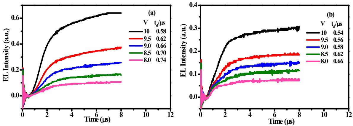
**Fig. S3** the transient EL signals for the device structure of ITO/TAPC (50nm)/Ir complexes (60nm)/ LiF (1 nm)/ Al (100 nm) under different applied fields of Ir(tfmphpm)<sub>2</sub>(pop) and Ir(tfmppm)<sub>2</sub>(pop).
