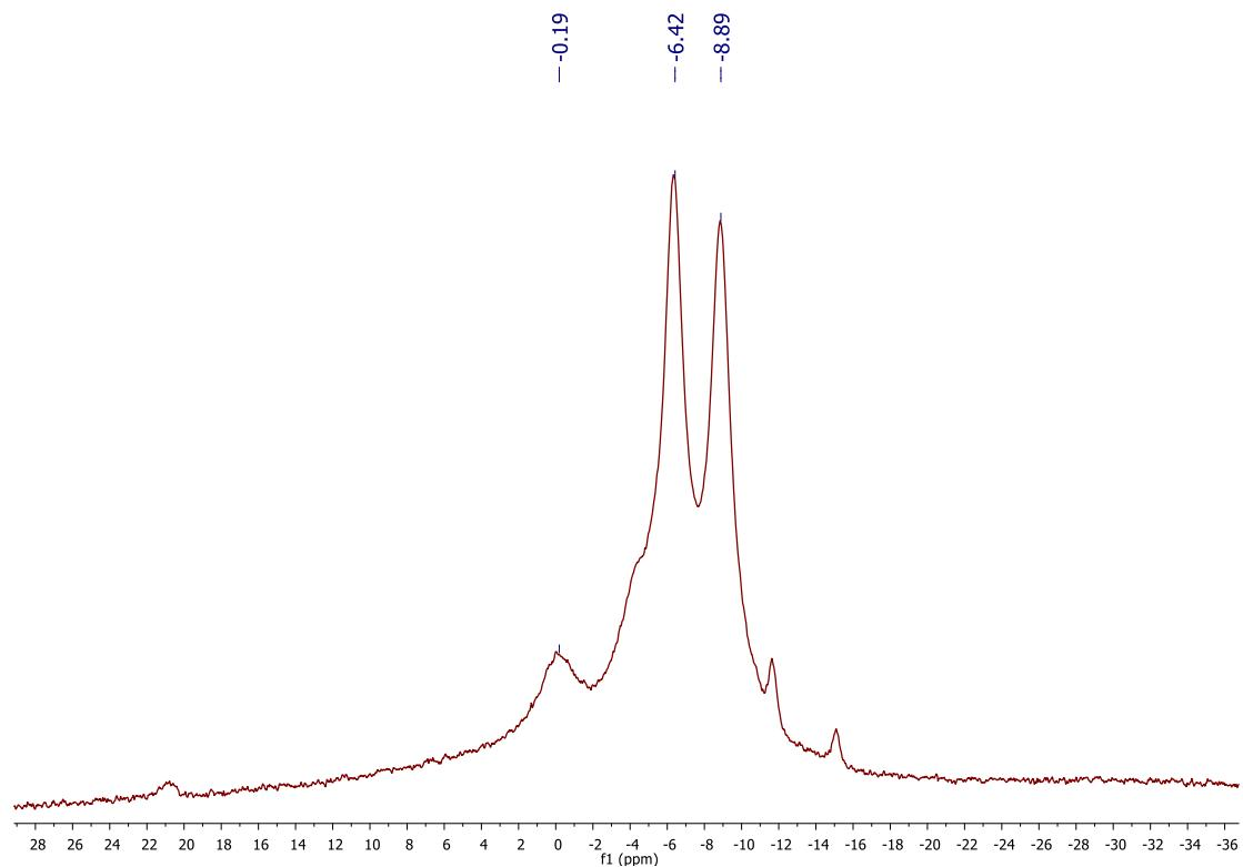
**Figure S7.** Evolution of the  $^{11}\text{B}\{^1\text{H}\}$ -NMR spectrum of compound **3** in MeOH/H<sub>2</sub>O to produce lower nuclearity species as compound **2**.
