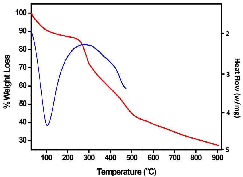
Figure S4. Thermal Gravimetric Analysis (TGA, red trace) and Differential Scanning Calorimetric (DSC, blue trace) plots for **2-Cu**.
