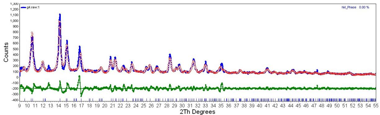
Figure S7B. Le Bail refinement of X-ray powder diffraction (XRPD) pattern of **1-Cu**. The observed, calculated (profile matching) and difference profiles are given in blue, red, and olive lines, respectively. Generated Bragg positions are provided as blue vertical lines.
