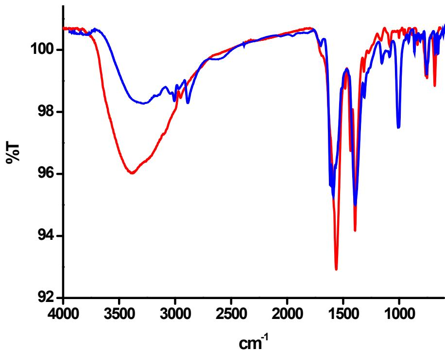
Figure S10. FTIR spectra of as synthesized **1-Cu** (red trace) and after methanol exchange experiment (blue trace).
