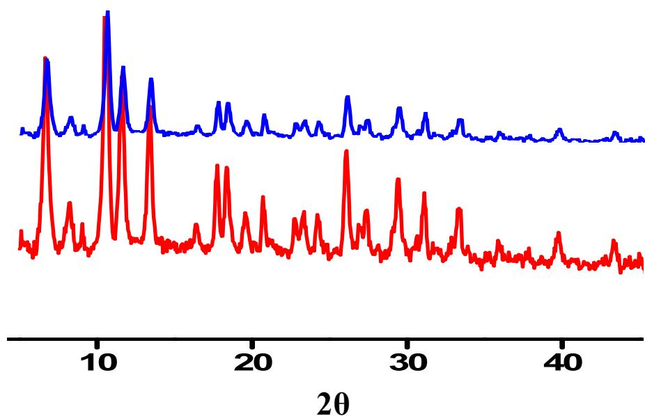
Figure S17. X-ray Powder Diffraction (XRPD) patterns for as-synthesized **1-Cu** (red trace) and the one recovered after oxidation of benzyl alcohol using TBHP (blue trace).
