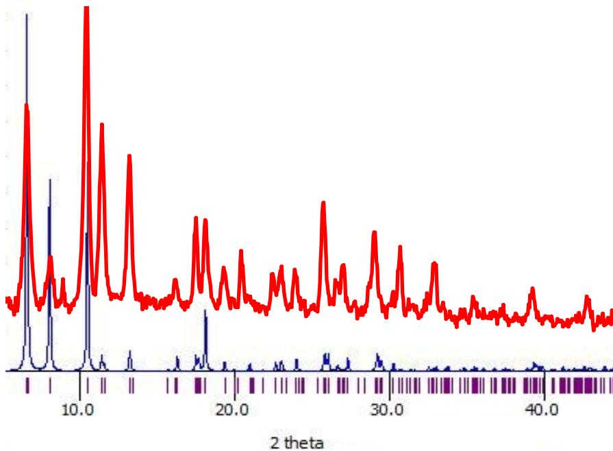
Figure S7A. X-ray Powder Diffraction (XRPD) patterns for as-synthesized **1-Cu** (red trace) and the one simulated from mercury 3.8 using single crystal diffraction data.
