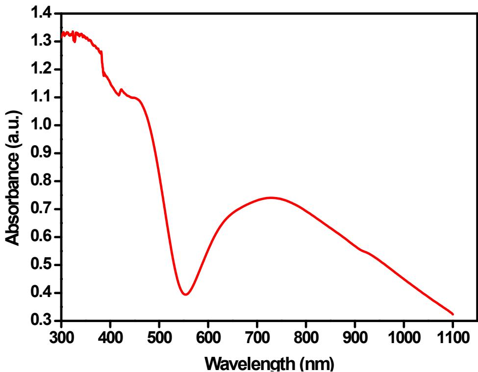
Figure S6. Diffuse reflectance UV-Vis spectrum of **2-Cu**.
