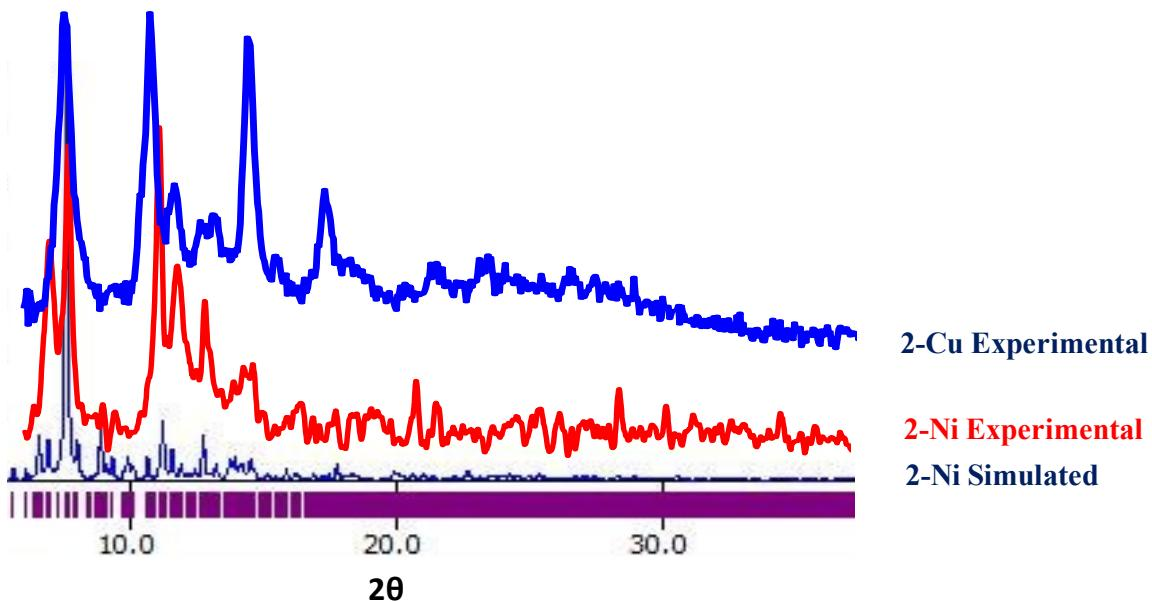
Figure S8A. X-ray Powder Diffraction (XRPD) patterns for as-synthesized **2-Cu** (blue trace) and its comparison with our earlier reported coordination polymer, **2-Ni** (red trace).
