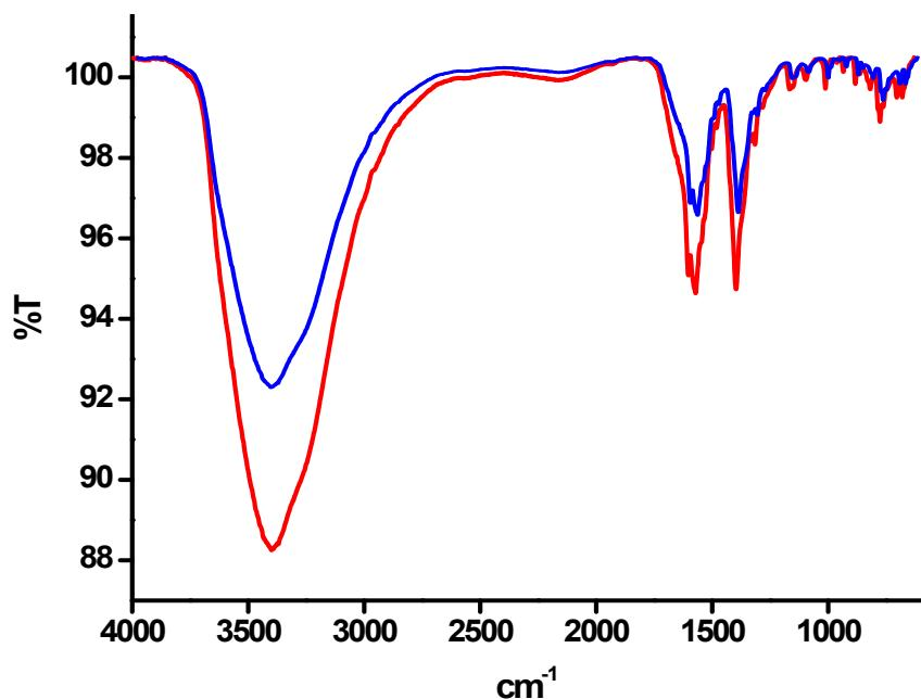
Figure S16. FTIR spectra of as-synthesized **1-Cu** (red trace) and the one recovered after oxidation of benzyl alcohol using TBHP (blue trace).
