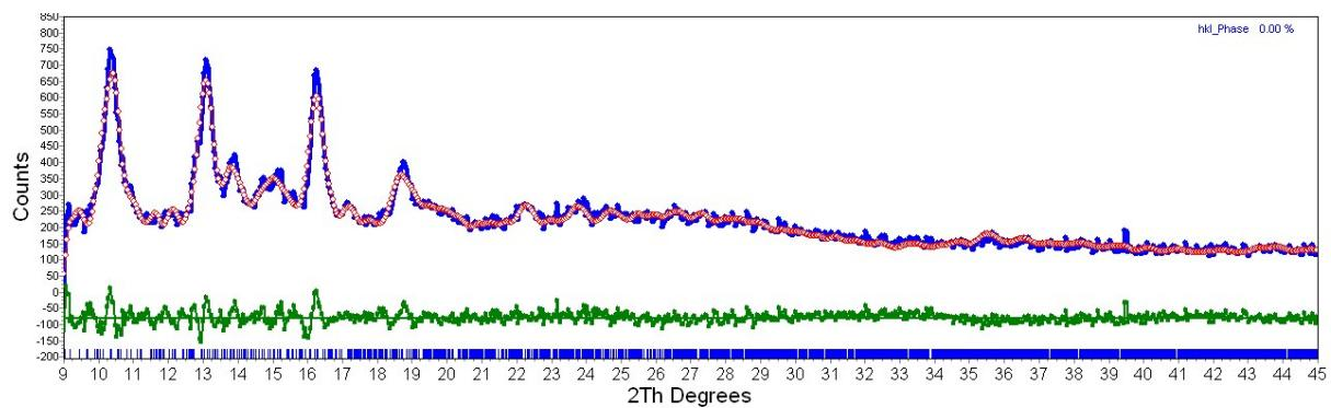
Figure S8B. Le Bail refinement of X-ray powder diffraction (XRPD) pattern of **2-Cu** using single crystal diffraction data for our earlier reported coordination polymer, **2-Ni**. The observed, calculated (profile matching) and difference profiles are given in blue, red, and olive lines, respectively. Generated Bragg positions are provided as blue vertical lines.
