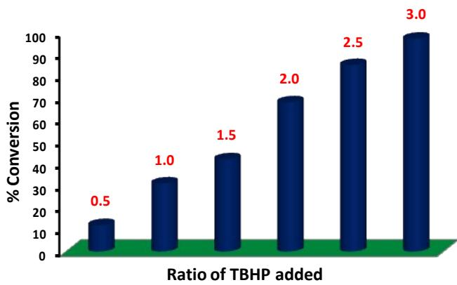
Figure S15. Effect of ratio of TBHP on the oxidation of benzyl alcohol using **1-Cu** as a catalyst.
