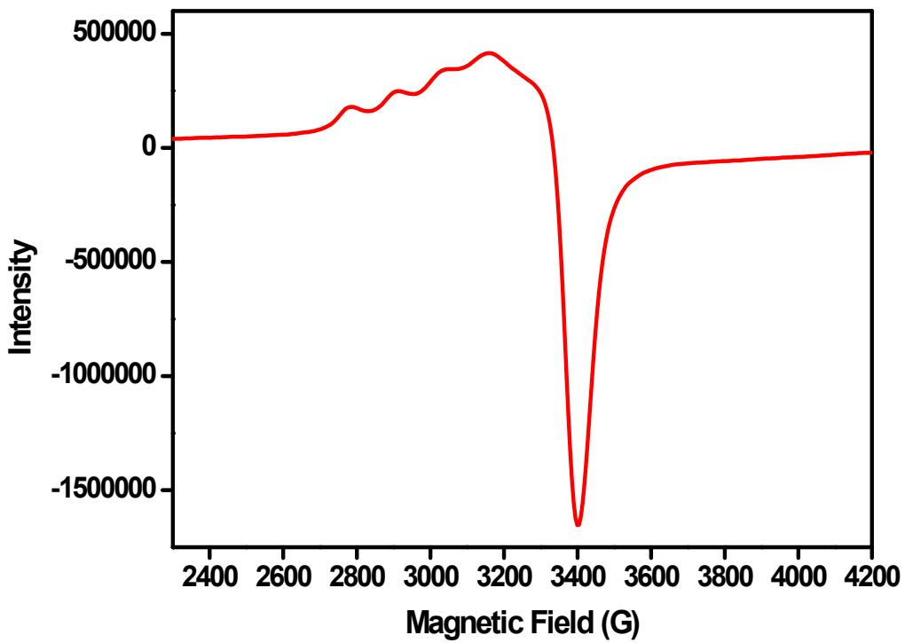
Figure S13. Solid-state EPR spectrum of powdered **1-Cu**.
