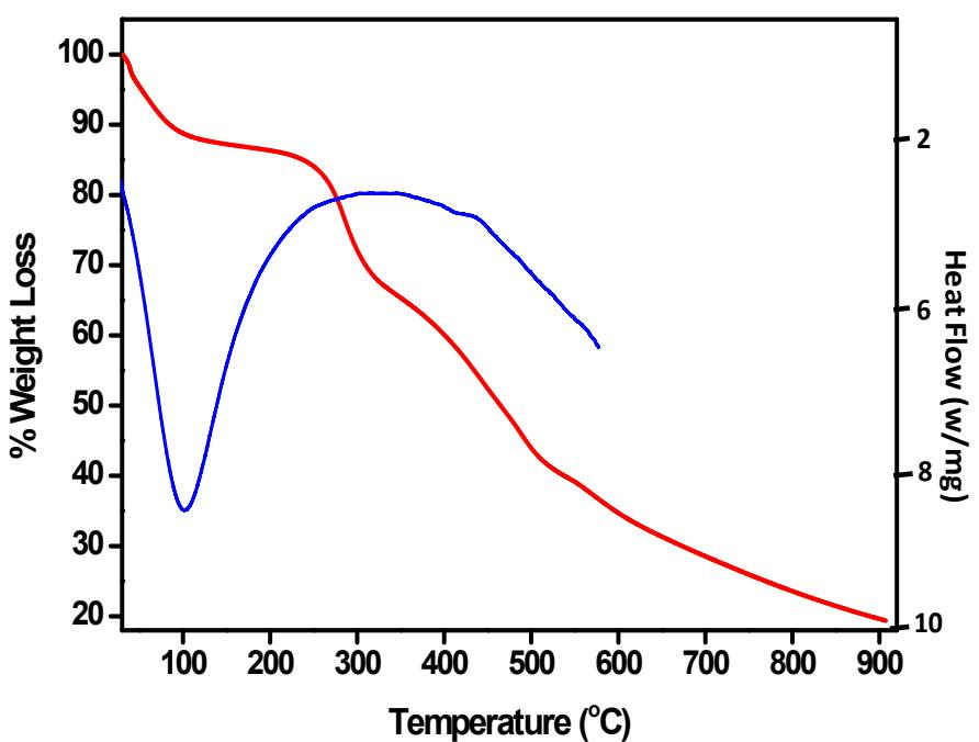
Figure S3. Thermal Gravimetric Analysis (TGA, red trace) and Differential Scanning Calorimetric (DSC, blue trace) plots for **1-Cu**.
