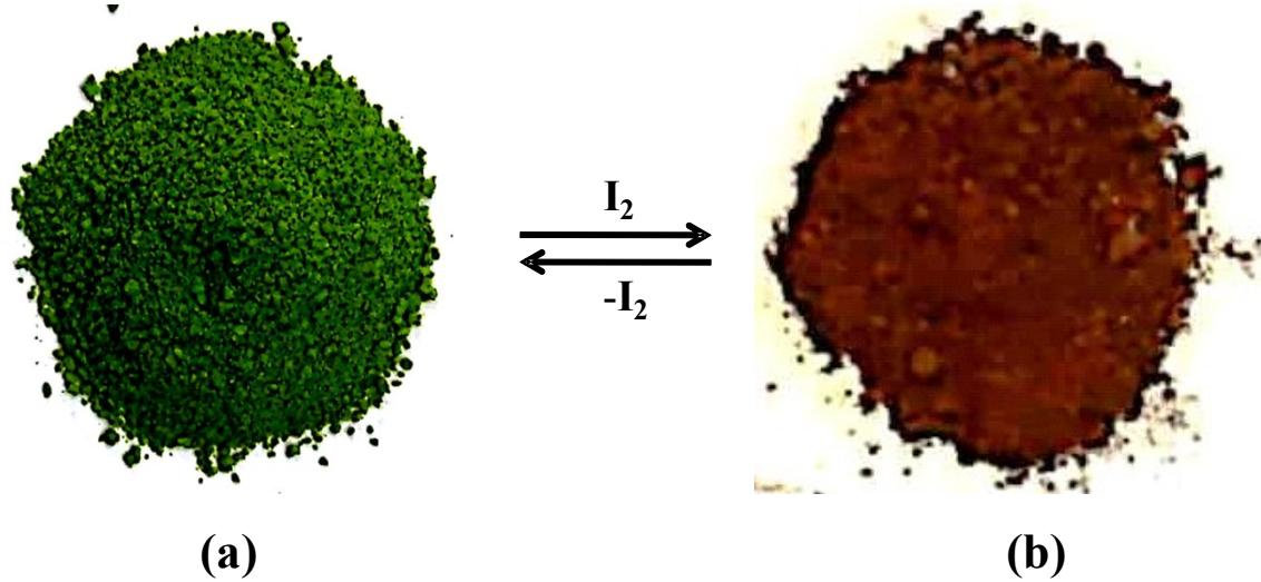
Figure S11. Optical images of a solid sample of (a) as synthesized **1-Cu** and (b) after molecular iodine adsorption experiment.
