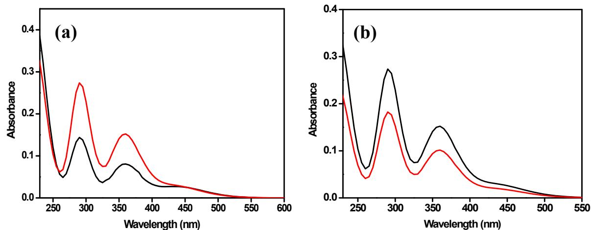
Figure S12. (a) UV-Vis spectrum of standard triiodide ion (red trace) and triiodide ion generated by **1-Cu** in MeOH solution of KI (black trace). (b) UV-Vis spectrum of standard triiodide ion (black trace) and triiodide ion generated by **2-Cu** in MeOH solution of KI (red trace).
