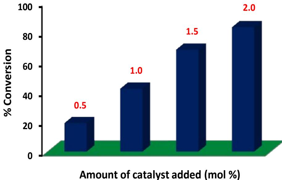
Figure S14. Effect of catalyst loading (**1-Cu**) on the epoxidation of styrene using molecular oxygen and isobutyraldehyde.
