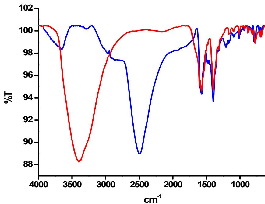
Figure S9. FTIR spectra of as synthesized **1-Cu** (red trace) and after  $\text{D}_2\text{O}$  exchange experiment (blue trace).
