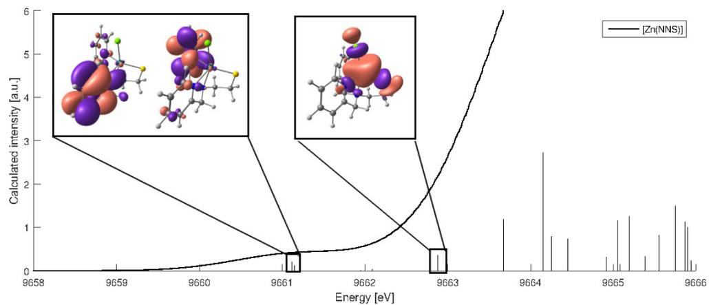
Figure S13: TDDFT spectra of [Zn(N-NNS)] focusing in the pre-edge absorption and highlighting molecular orbitals involved in these transitions. Nitrogen atoms are colored in blue, oxygen in red, sulfur in yellow, chlorine atoms in green, zinc in grey and carbon in light grey.
