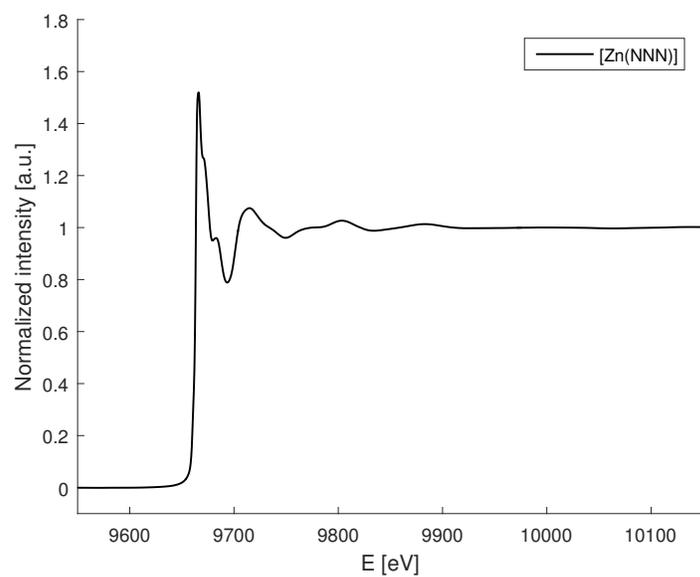
Figure S8: Zn K-edge X-ray absorption spectrum of the  $[\text{Zn}(\text{N}-\text{NNN})\text{Cl}](\text{PF}_6)$  complex in solid state.
