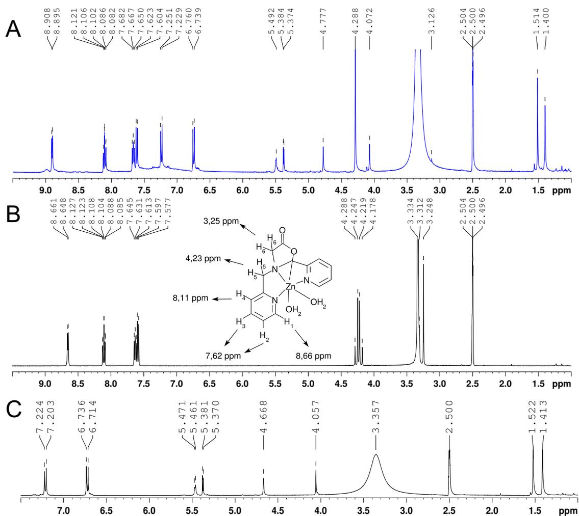
Figure S7:  $^1\text{H}$  NMR spectra of the complex  $[\text{Zn}(\text{N-NNO})(\text{H}_2\text{O})_2](\text{NO}_3)$  (A) and amoxicillin with  $[\text{Zn}(\text{N-NNO})(\text{H}_2\text{O})_2](\text{NO}_3)$  (B) in  $d_6$ -DMSO. The spectrum of amoxicillin in  $d_6$ -DMSO is shown for reference (C)
