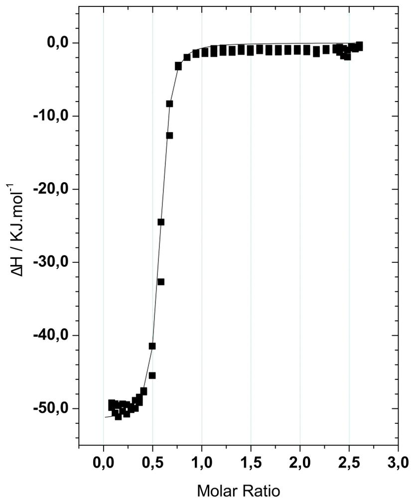
Figure S15: Enthalpy variation by molar ratio of amoxicillin titrated to a solution of  $[\text{Zn}(\text{NNN})\text{Cl}](\text{PF}_6)$  complex and the curve resultant of the one-site fitting analysis.
