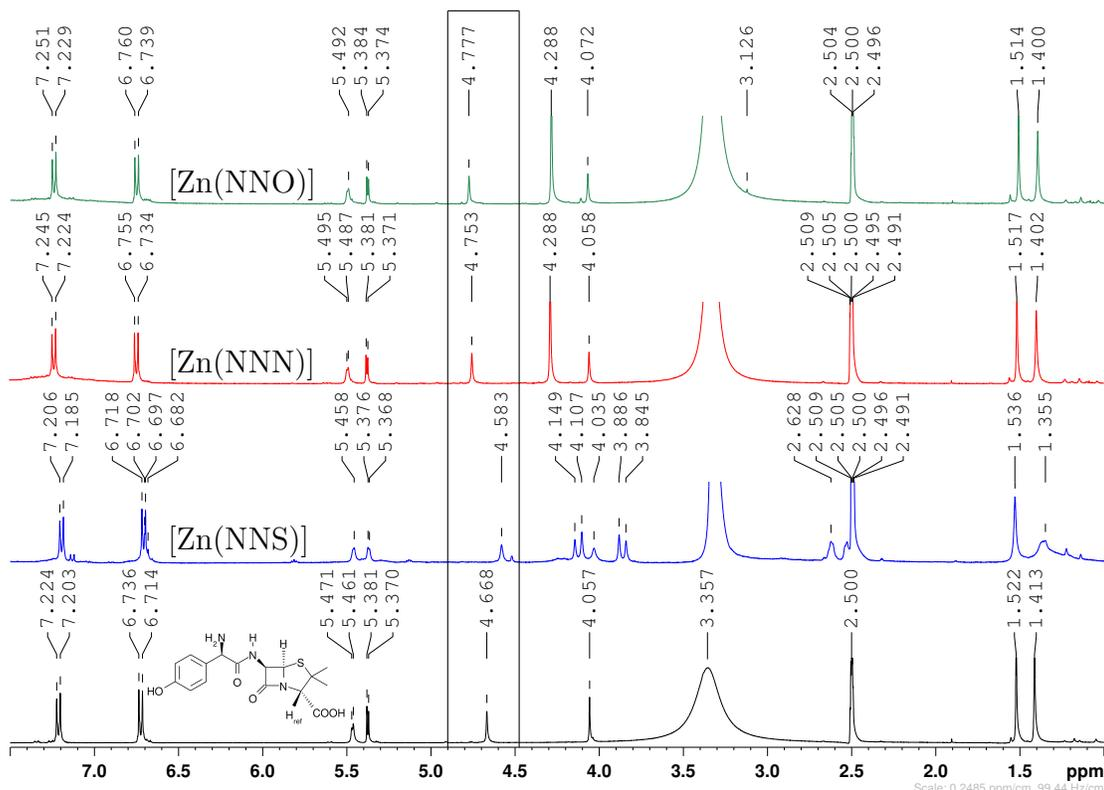
Figure S4:  $^1\text{H}$  NMR spectra of the amoxicillin interaction with our mimetics in  $d_6$ -DMSO, highlighting the geminal hydrogen used as probe.  $[\text{Zn}(\text{N}-\text{NNO})] + \text{Am}$  (green),  $[\text{Zn}(\text{N}-\text{NNN})] + \text{Am}$  (red),  $[\text{Zn}(\text{N}-\text{NNS})] + \text{Am}$  (blue) and Amoxicillin (Am) (black).
