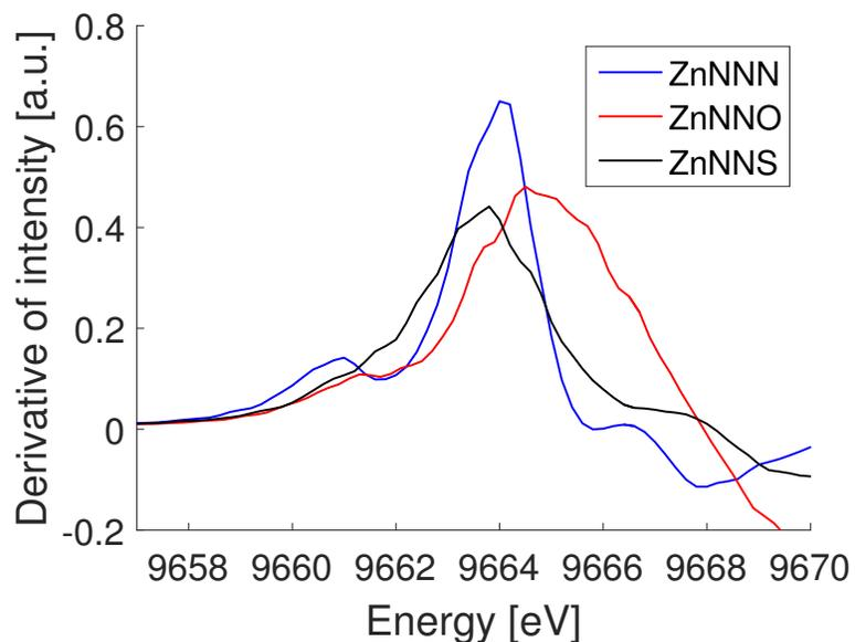
Figure S11: First derivative of Zn K-edge XAS spectra of solid model complexes [Zn(N-NNX)], with X = O, N or S, ([Zn(N-NNN)] in blue, [Zn(N-NNO)] in red, and [Zn(N-NNS)] in black). The rising edge energies were taken as the maximum of the edge (9663-4 eV). It is possible to see the variation between its position for each complex and also highlighting the pre-edge absorption around 9661 eV.
