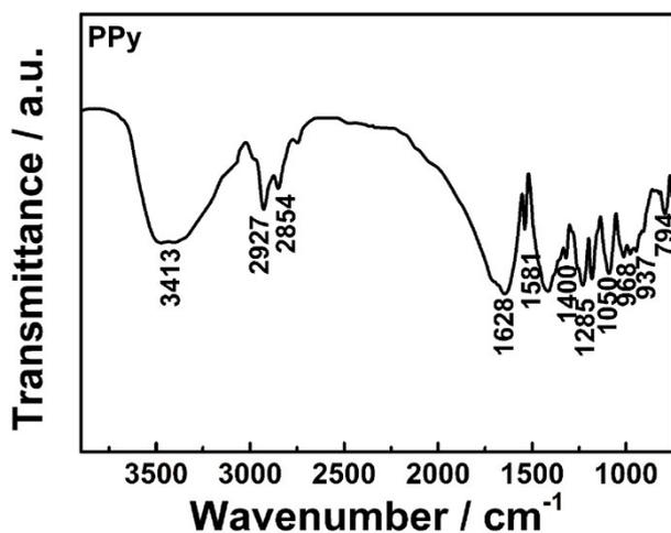
**Fig. S2.** FTIR spectra of the as-prepared CNT@PPy-500.
