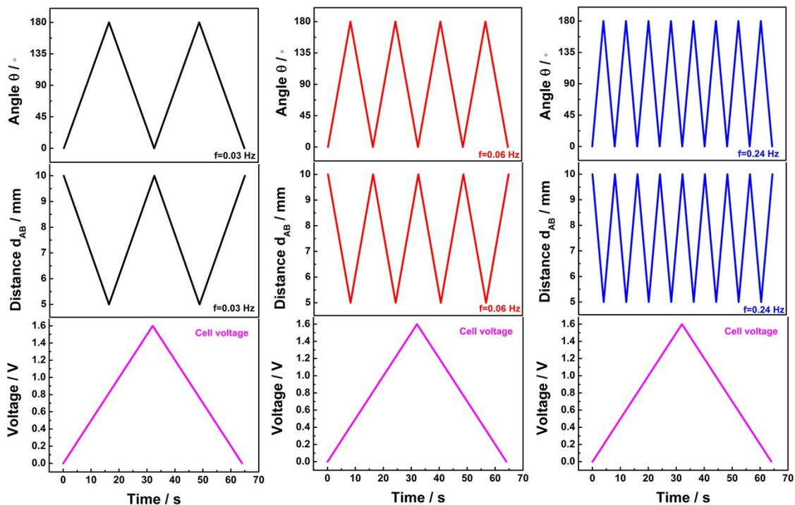
**Fig. S10.** Electrochemical properties of  $\text{CuCo}_2\text{O}_4//\text{PPy}$  under different frequencies of dynamic bending conditions. The changes of bending angle  $\theta$ , distance  $d_{AB}$  and cell voltage versus time at low and high frequencies during one scan of CV at  $50 \text{ mV s}^{-1}$ .
