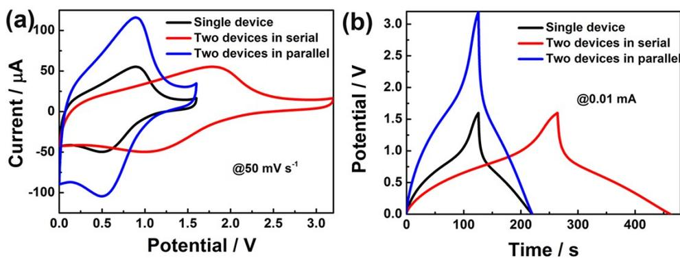
Fig. S9. (a) CV curves of two devices connected in series and parallel, (b) GCD of two devices connected in series and parallel.
