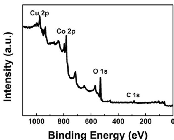
**Fig. S1.** XPS spectra of  $\text{CuCo}_2\text{O}_4$ .
