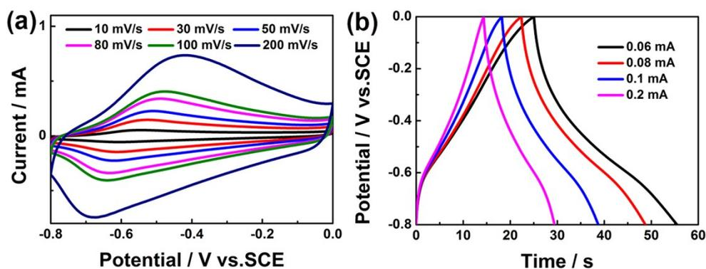
Fig. S4. Electrochemical properties of CNT@PPy-100 electrode.
