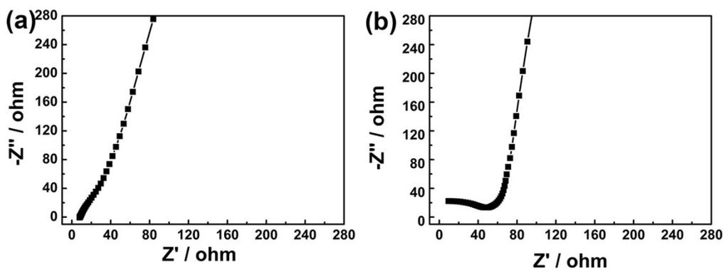
Fig. S3. (a-b) EIS curves of CNT@CuCo<sub>2</sub>O<sub>4</sub> and CNT@PPy-500 electrode.
