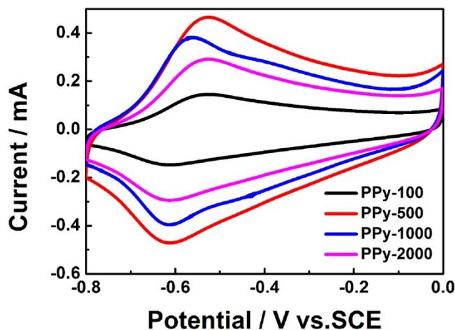
Fig. S7. CV curves at  $30 \text{ mV s}^{-1}$  for different CNT@PPy electrodes.
