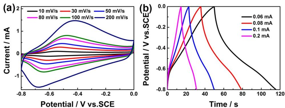
Fig. S6. Electrochemical properties of CNT@PPy-2000 electrode.
