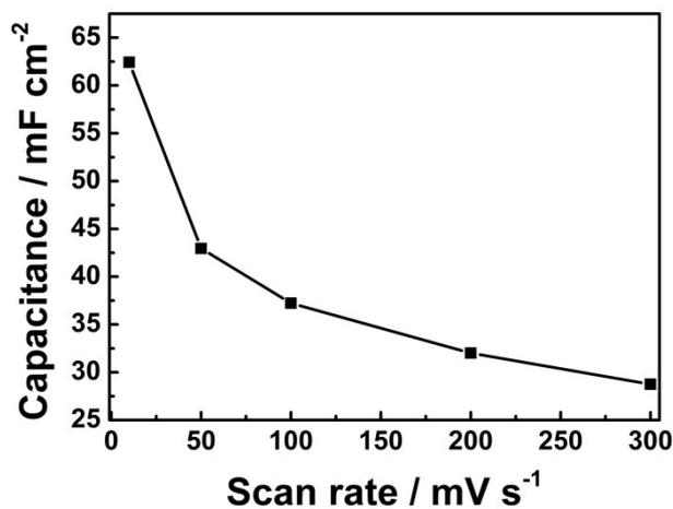
Fig. S8. Areal capacitance of ACS at different scan rate.
