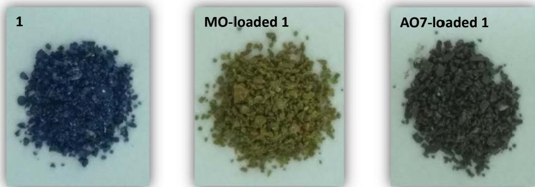
**Fig. S7** Photographs of crystalline materials of **1** before and after immersion of MO and AO7.
