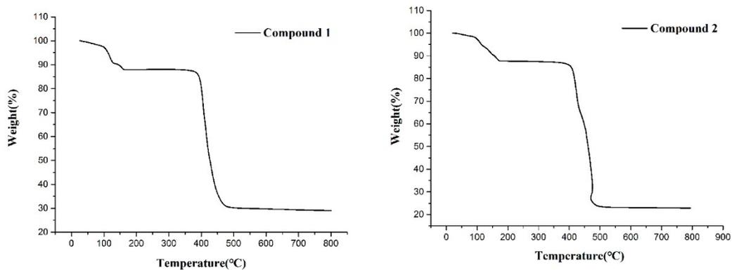
Fig. S3 Thermogravimetric analyses (TGA) profiles of **1** and **2**.
