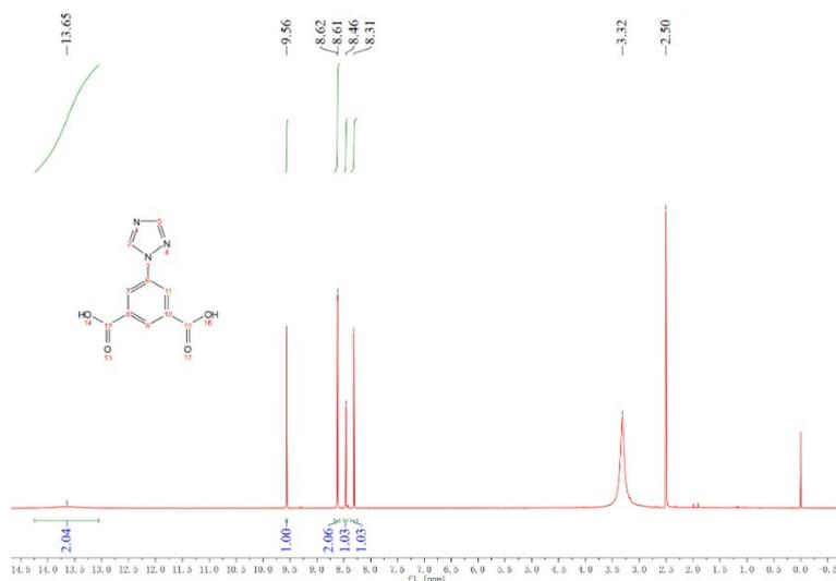
Fig. S1 <sup>1</sup>H-NMR spectrum of ligand H<sub>2</sub>L (DMSO-d<sub>6</sub>).
