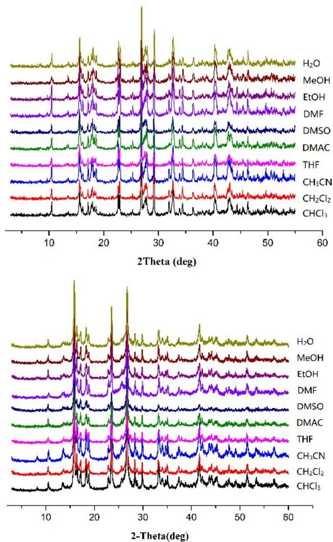
Fig. S4 PXRD patterns of **1** and **2** immersed in various solvents after 60 h.
