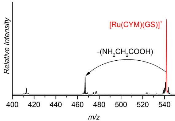
**Figure S13.** MS/MS/MS experiment of mass-selected ion  $[\text{Ru}(\text{CYM})(\text{GS})]^+$ .
