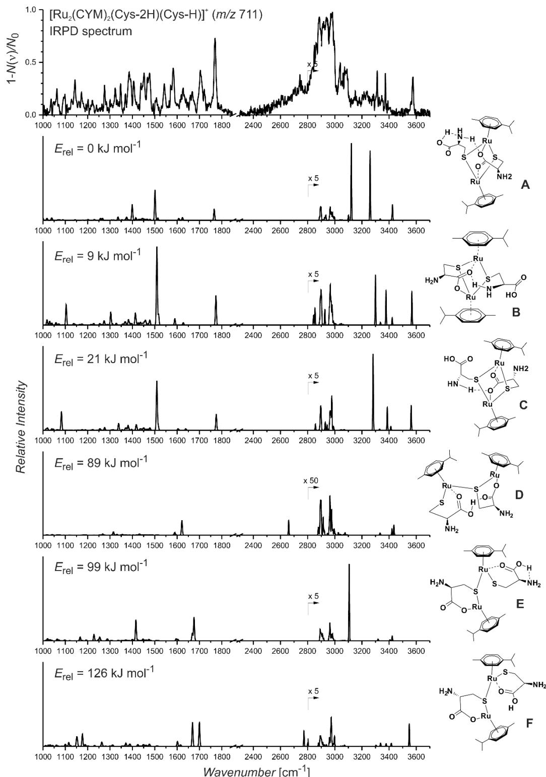
**Figure S14.** a) Helium tagging IRPD spectrum of mass-selected ion  $[\text{Ru}_2(\text{CYM})_2(\text{Cys-2H})(\text{Cys-H})]^+$  ( $m/z$  711). b) Theoretical IR spectra (B3LYP-D3/6-31G\*\*;SDD(Ru)) of possible isomers of  $[\text{Ru}_2(\text{CYM})_2(\text{Cys-2H})(\text{Cys-H})]^+$ . The relative energies refer to energies at 0 K. The geometries and energetics of the optimised structures can be found in Table S3.
