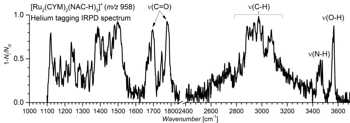
**Figure S16.** Helium tagging IRPD spectrum of mass-selected ions  $[\text{Ru}_2(\text{CYM})_2(\text{NAC-H})_3]^+$  ( $m/z$  958).
