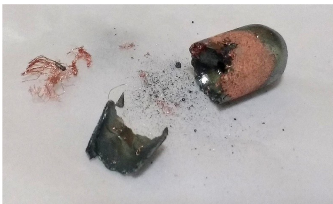
Figure S1: The ingot after annealing showing the copper precipitates
