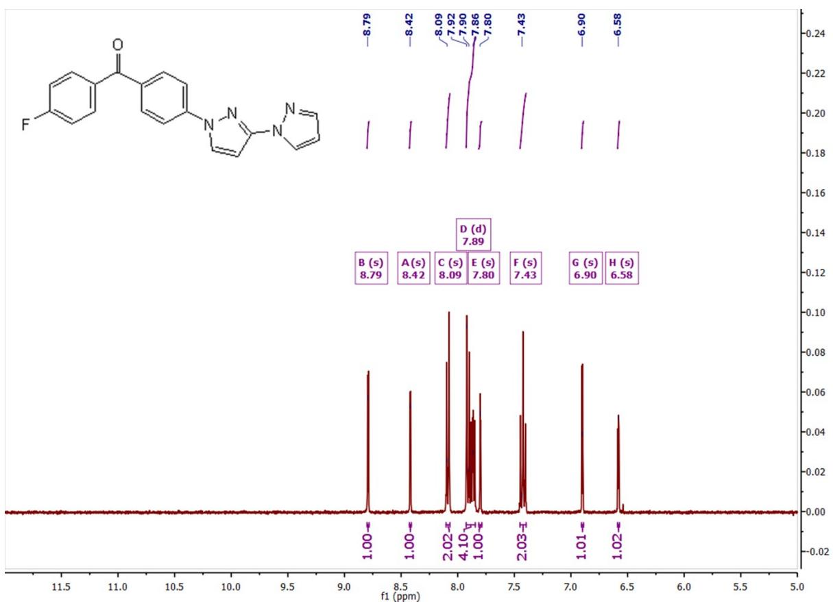
Fig. S4  $^1\text{H}$  NMR spectra of FOB ( $d^6\text{-DMSO}$  as solvent)
