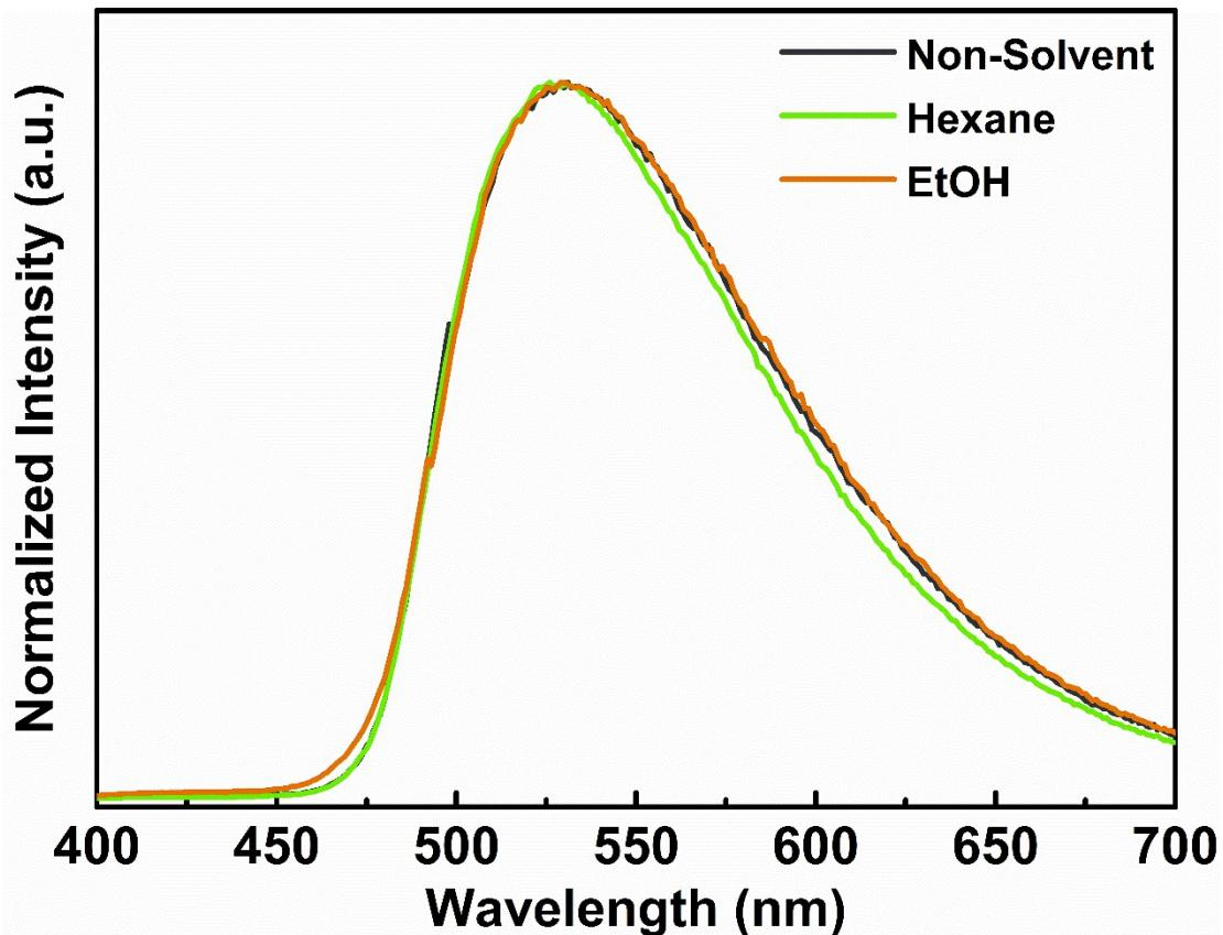
Fig. S13 Photoluminescence spectra of POB crystal without fumed and after fumed by hexane and ethanol.
