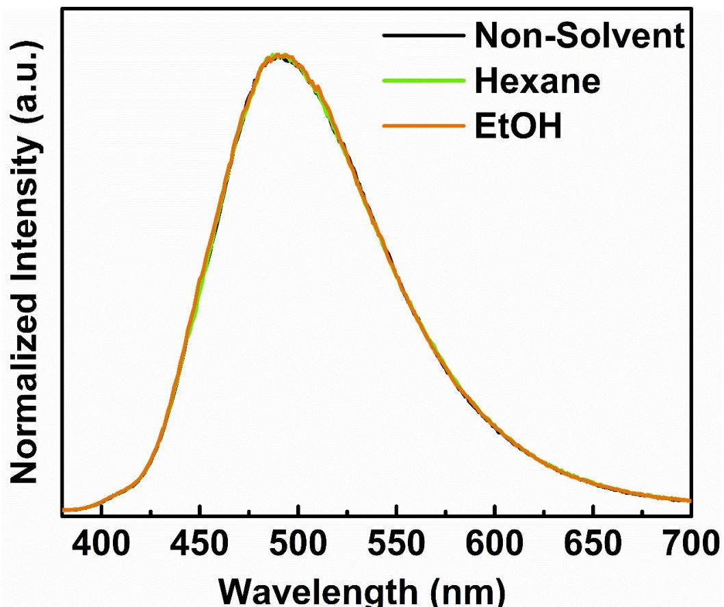
Fig. S12 Photoluminescence spectra of OBC crystal without fumed and after fumed by hexane and ethanol.
