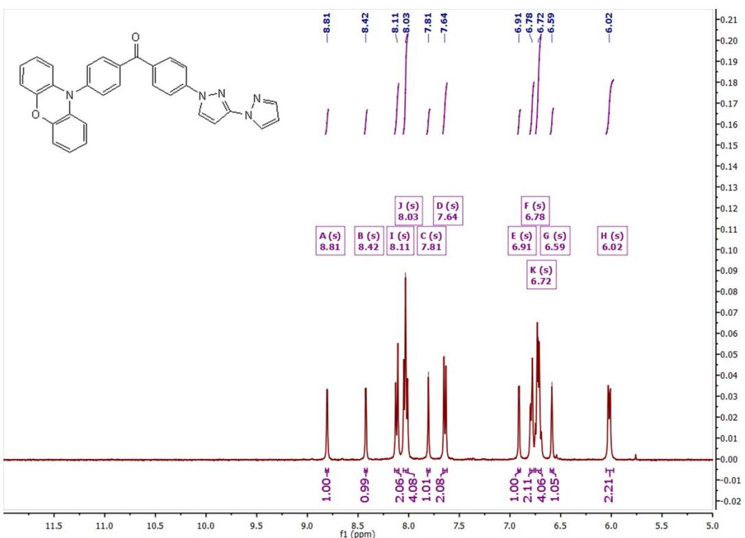
**Fig. S5** <sup>1</sup>H NMR spectra of POB ( $d^6$ -DMSO as solvent)
