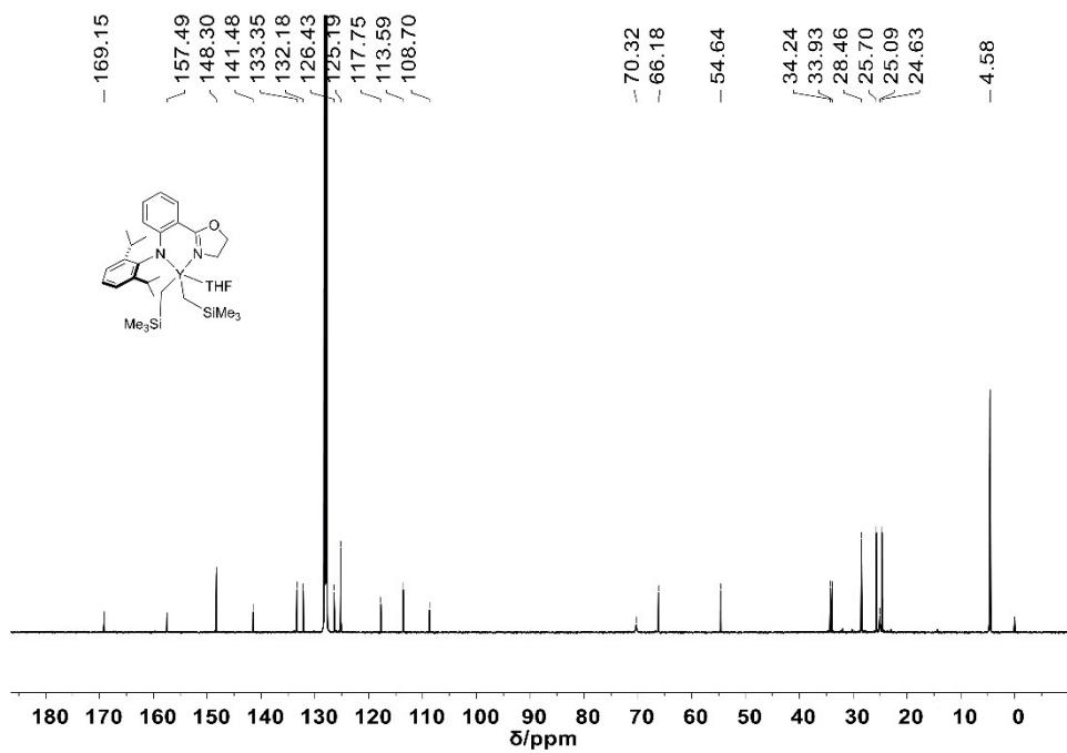
**Fig. S21.**  $^{13}\text{C}$  NMR spectrum (125 MHz,  $\text{C}_6\text{D}_6$ , 25°C) of  $\text{L}^4\text{Y}(\text{CH}_2\text{SiMe}_3)_2\text{THF}$  (**6**).
