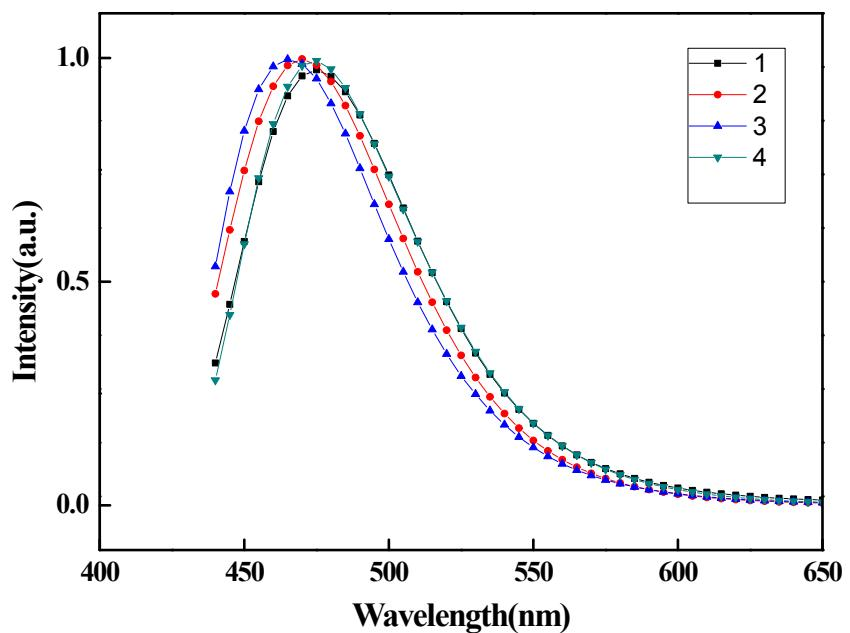
**Fig. S5.** Fluorescence emission spectra of complexes **1–4** at 25 °C in hexane.
