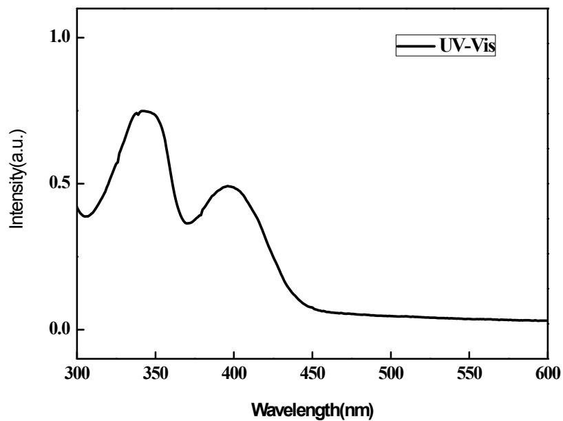
**Fig. S1.** UV-Vis spectrum of  $L^1\text{Sc}(\text{CH}_2\text{SiMe}_3)_2\text{THF}$  (**1**) at 25 °C in hexane.
