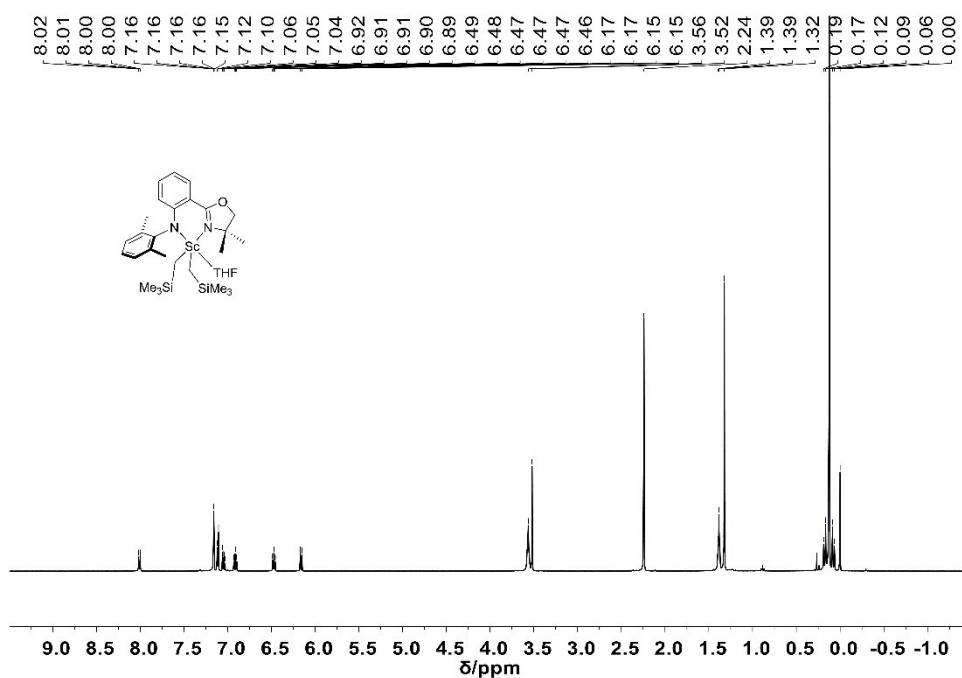
**Fig. S10.**  $^1\text{H}$  NMR spectrum (500 MHz,  $\text{C}_6\text{D}_6$ , 25°C) of  $\text{L}^1\text{Sc}(\text{CH}_2\text{SiMe}_3)_2\text{THF}$  (**1**).
