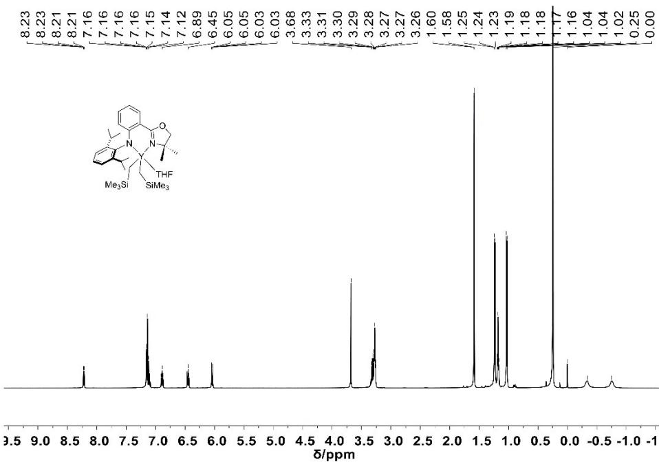
**Fig. S13.** <sup>1</sup>H NMR spectrum (500 MHz, C<sub>6</sub>D<sub>6</sub>, 25°C) of L<sup>2</sup>Y(CH<sub>2</sub>SiMe<sub>3</sub>)<sub>2</sub>THF (**4**).
