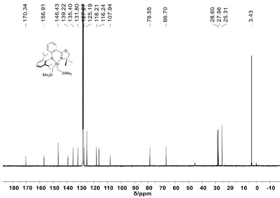
**Fig. S17.**  $^{13}\text{C}$  NMR spectrum (125 MHz,  $\text{C}_6\text{D}_6$ , 25°C) of  $\text{L}^2\text{Sc}(\text{CH}_2\text{SiMe}_3)_2$  (**2**).
