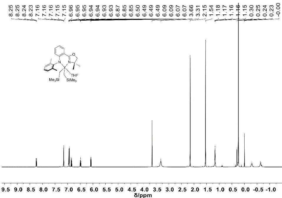
**Fig. S12.** <sup>1</sup>H NMR spectrum (500 MHz, C<sub>6</sub>D<sub>6</sub>, 25°C) of L<sup>1</sup>Y(CH<sub>2</sub>SiMe<sub>3</sub>)<sub>2</sub>THF (**3**).
