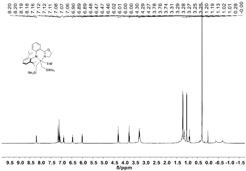
**Fig. S15.** <sup>1</sup>H NMR spectrum (500 MHz, C<sub>6</sub>D<sub>6</sub>, 25°C) of L<sup>4</sup>Y(CH<sub>2</sub>SiMe<sub>3</sub>)<sub>2</sub>THF (6).
