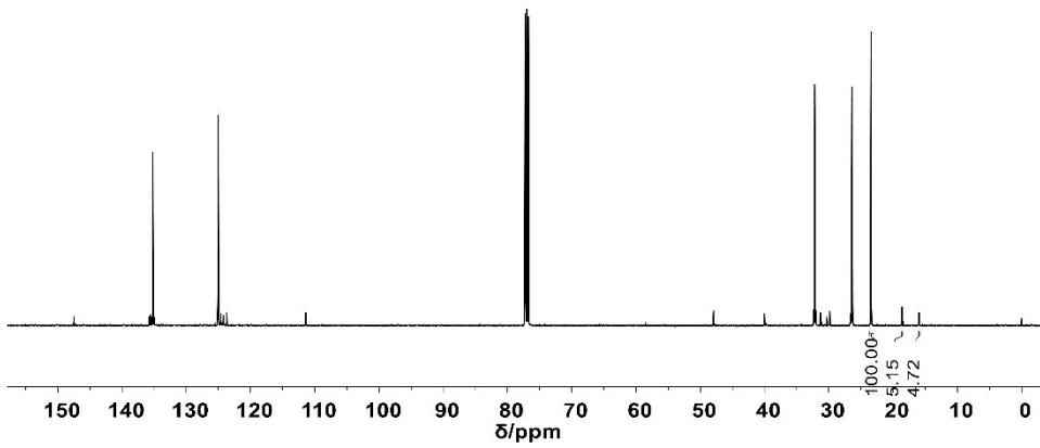
**Fig. S27.**  $^{13}\text{C}$  NMR spectrum (125 MHz,  $\text{CDCl}_3$ , 25°C) of the resultant PIP (Table 4, run 10).
