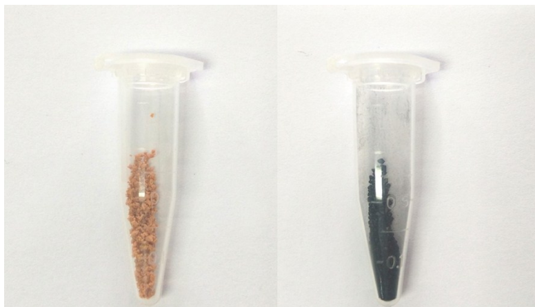
Figure S1 Digital photos of the Co-MOF (left) and corresponding Co@NC-P(3-1) catalyst (right).
