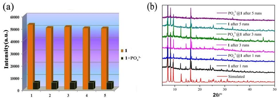
**Fig. S9** (a) Recovery test of **1** in aqueous solution. The orange columns represent the initial relative luminescent intensity and the black columns represent the relative intensity on addition of  $\text{PO}_4^{3-}$ , (b) PXRD patterns of  $\text{PO}_4^{3-}@\mathbf{1}$  after 5 runs.
