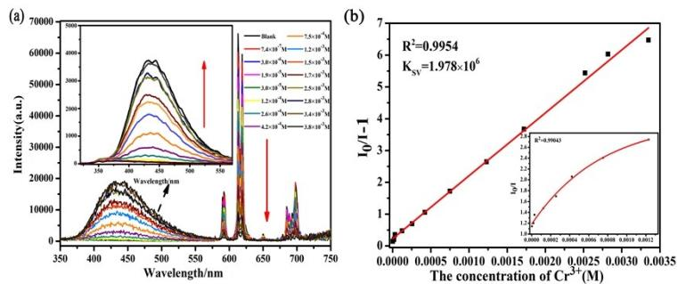
**Fig. S5** (a) Emission spectra of **1** dispersed in the various concentrations of  $\text{Cr}^{3+}$  ions at the excitation of 314nm. (b) Linear Stern-Volmer curves in low concentration range of  $\text{Cr}^{3+}$  ions. (Inset: Nonlinear Stern-Volmer curves of  $\text{Cr}^{3+}$  ions)
