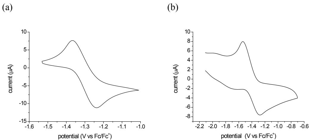
**Figure S2.** Cyclic voltammogram of 3 mM THF solution of (a)  $[(\text{MeO})_2\text{Fe}(\text{NO})_2]^-$  (**2**) and (b)  $[(\text{PhO})_2\text{Fe}(\text{NO})_2]^-$  (**6**) with 0.1 M  $[{}^n\text{Bu}_4\text{N}]^+[\text{PF}_6]^-$  as the supporting electrolyte at scan rate of 0.5 V/s.
