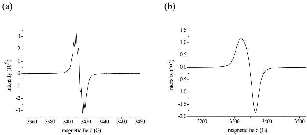
**Figure S1.** EPR spectra of complex **2** in THF (a) at 285 K ( $g_{av} = 2.022$ ,  $a_N = 2.44$  G), and (b) at 77 K ( $g_{av} = 2.023$ ,  $g_1 = 2.04$ ,  $g_2 = 2.02$ , and  $g_3 = 2.01$ ).
