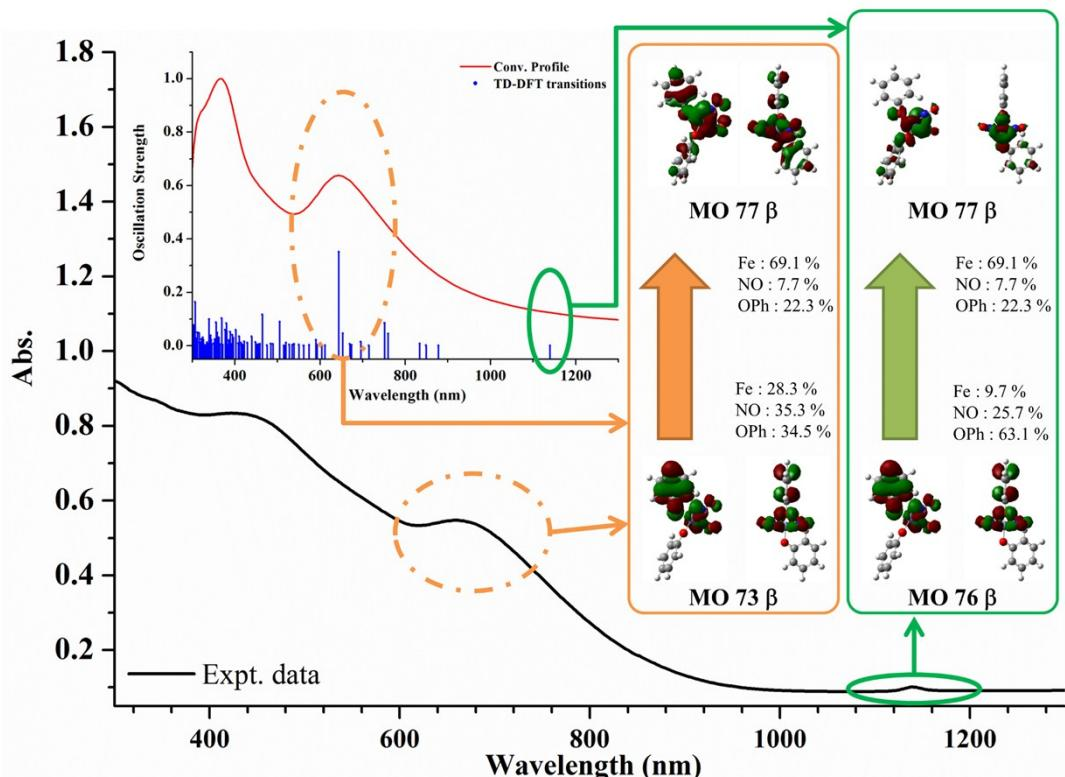
**Figure S5.** Experimental and simulated UV-vis spectra of complex 6.
