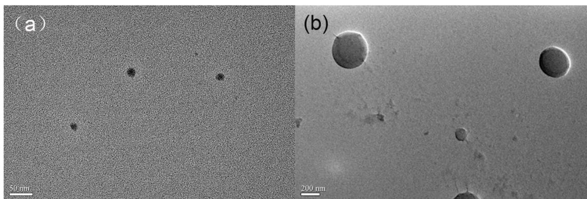
**Fig. S3** TEM image of nanoaggregates of complex **1** formed in DMSO–H<sub>2</sub>O mixtures with 0% (a) and 90% (b) water fraction.
