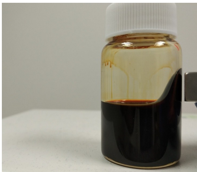
Figure S1: Magnetic colloidal fluid (ferrofluid) composed of oleate-coated USPIOs suspended in chloroform.
