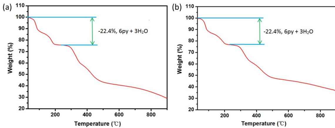
**Figure S1.** Thermogravimetric analysis of **1** (a) and **2** (b). The black solid lines show the loss of solvent molecules.
