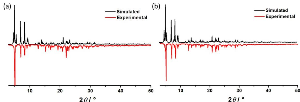
**Fig. S2.** Experimental and simulated powder X-ray diffraction (PXRD) for **1** (a) and **2** (b).
