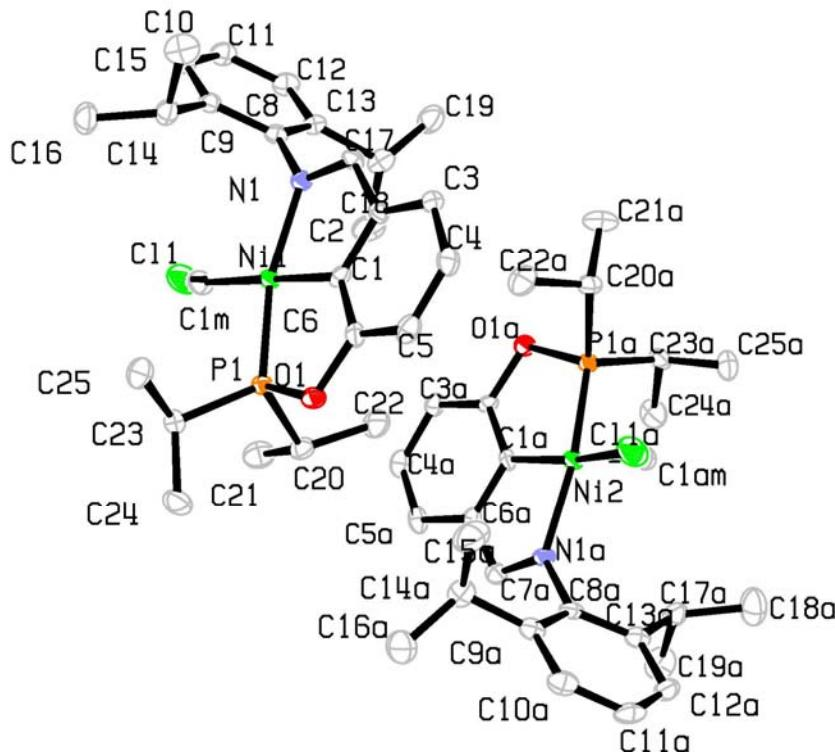
**Figure S10.** The general view of one of the independent molecules of co-crystal of 0.81 **6-Ar** and 0.19 (*i*-PrPOCN<sup>Ar</sup>)NiCl illustrating the superposition of Cl(1) and Me-groups. Atoms are shown by thermal ellipsoids (50% probability level). Hydrogen atoms are omitted for clarity.
