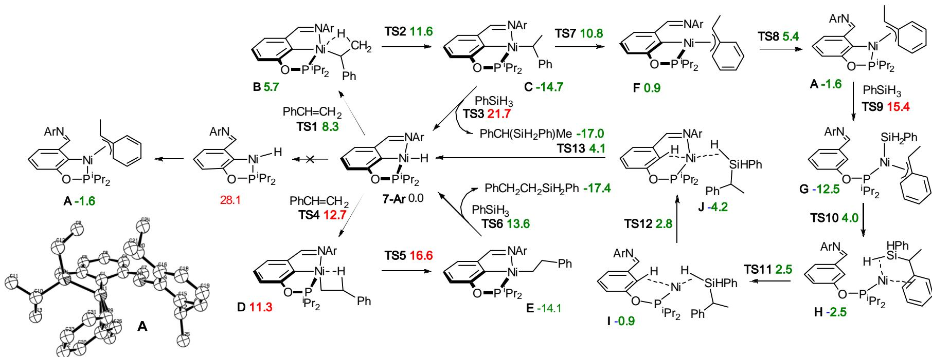
**Figure S14.** DFT-calculated mechanism for **7-Ar**-catalyzed hydrosilylation of styrene with PhSiH<sub>3</sub> at 60 °C (free energies are in kcal·mol<sup>-1</sup>).
