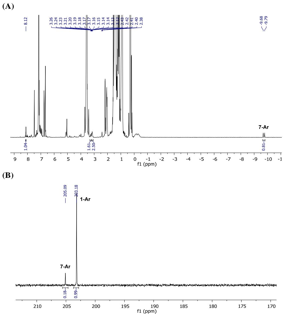
**Figure S1.**  $^1\text{H}$ - (A) and  $^{31}\text{P}\{\text{H}\}$ -NMR (B) spectra from the reaction of **1-Ar** with L-Selectride in  $\text{C}_6\text{D}_6$  taken after 10 min at room temperature, showing 16% conversion (by  $^{31}\text{P}\{\text{H}\}$ -NMR) of **1-Ar** to **7-Ar**.
