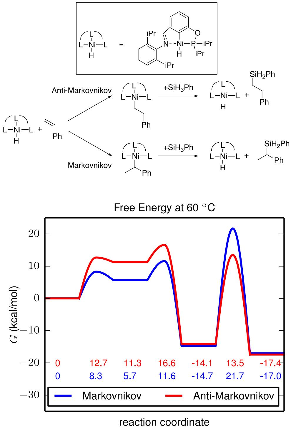
**Figure S11.** Computed mechanism for direct addition of  $\text{PhSiH}_3$  to the alkynickel species
