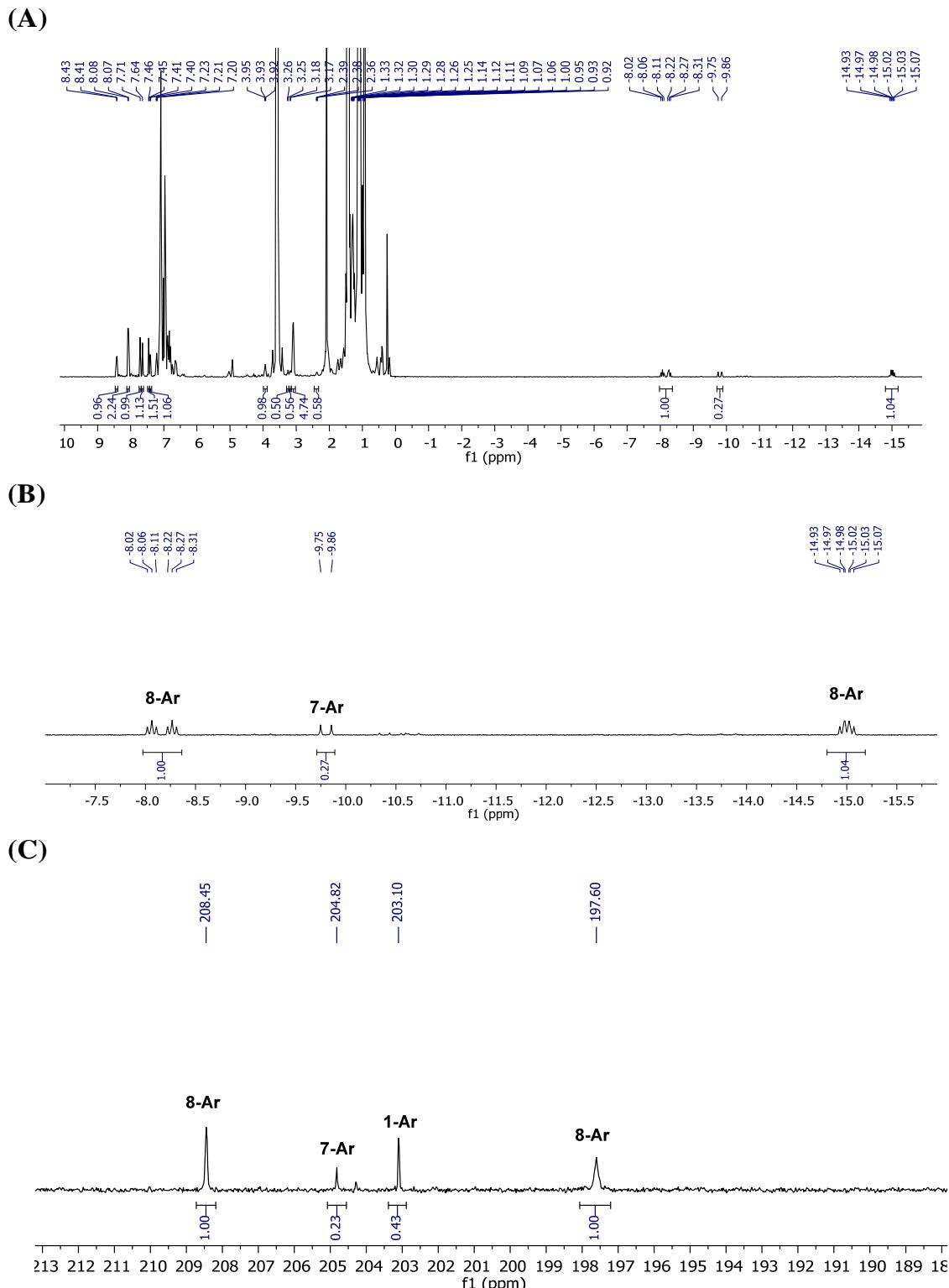
**Figure S2.**  $^1\text{H}$ - (**A**), expanded hydride region (**B**) and  $^{31}\text{P}\{^1\text{H}\}$ -NMR (**C**) spectra from the reaction of **1-Ar** with LiBH<sub>Et</sub><sub>3</sub> in PhMe-d<sub>8</sub> taken after 10 min at room temperature, showing 74% conversion (by  $^{31}\text{P}\{^1\text{H}\}$ -NMR) of **1-Ar** to a mixture of **7-Ar** and **8-Ar** (app. 1:4 ratio by  $^1\text{H}$ -NMR, respectively).
