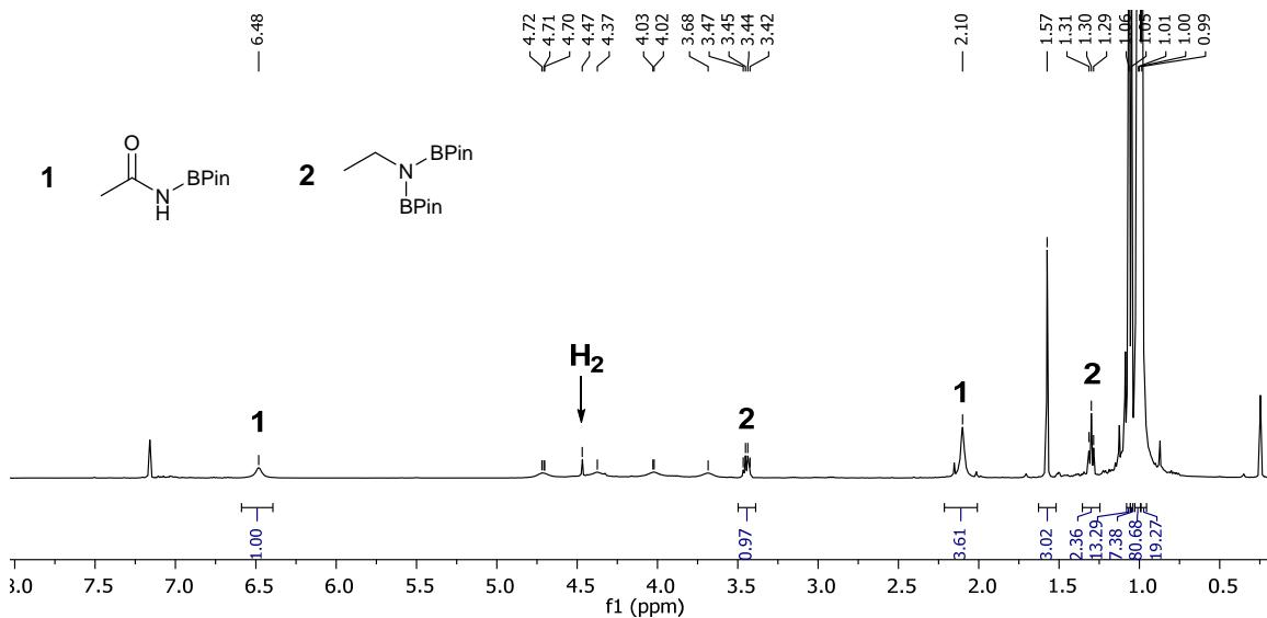
**Figure S5.**  $^1\text{H}$ -NMR spectrum for hydroboration of acetamide with HBPin at 60  $^\circ\text{C}$  in the presence of 5 mol% of **6-Ar**, taken after 5 h and showing formation of a mixture of  $\text{MeC(O)NH(BPin)}$  and  $\text{EtN(BPin)}_2$ .
