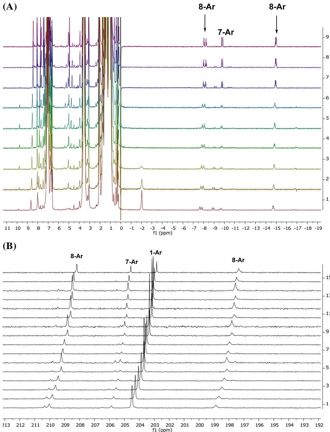
**Figure S3.** Variable temperature NMR analysis (-80 °C to room temperature) of the reaction of **1-Ar** with LiBH<sub>3</sub> in PhMe-d<sub>8</sub>, showing formation of a mixture of **7-Ar** and **8-Ar**:  $^1\text{H}$ -NMR spectra (A) and  $^{31}\text{P}\{\text{H}\}$ -NMR spectra (B).
