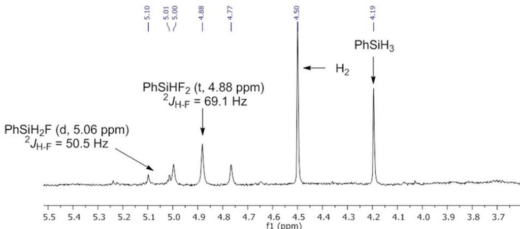
**Figure S4.** A fragment of <sup>1</sup>H-NMR spectrum of the reaction of **3-Ar** with PhSiH<sub>3</sub> in PhMe-d<sub>8</sub> at 0 °C, showing formation of PhSiH<sub>2</sub>F, PhSiHF<sub>2</sub> and H<sub>2</sub>.
