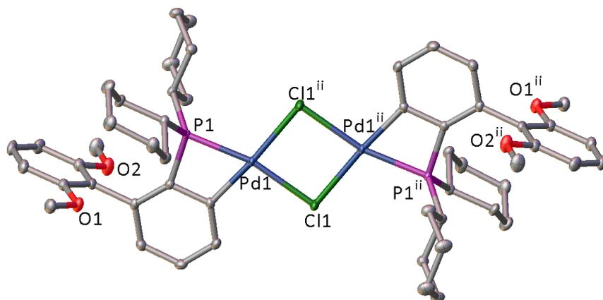
**Figure 5:** Crystal structure of **2**, with hydrogen atoms omitted for clarity. Symmetry code <sup>ii</sup> 1-x, -y, -z.
