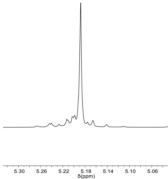
**Fig. S15.**  $^1\text{H}\{^1\text{H}\}$  NMR spectrum ( $\text{CDCl}_3$ , 500 MHz, 298 K) of the poly-*L*-lactide produced using  ${}^{\text{Me}_2}\text{SB}(\text{Cp}^{\text{Me}},\text{I}^*)\text{ZrCl}_2$  (**2**). Polymerisation conditions: 80 °C,  $[\text{LA}]_0/[\text{M}]_0 = 50$ ,  $[\text{LA}]_0 = 0.5 \text{ M}$  and  $\text{CDCl}_3$ .
