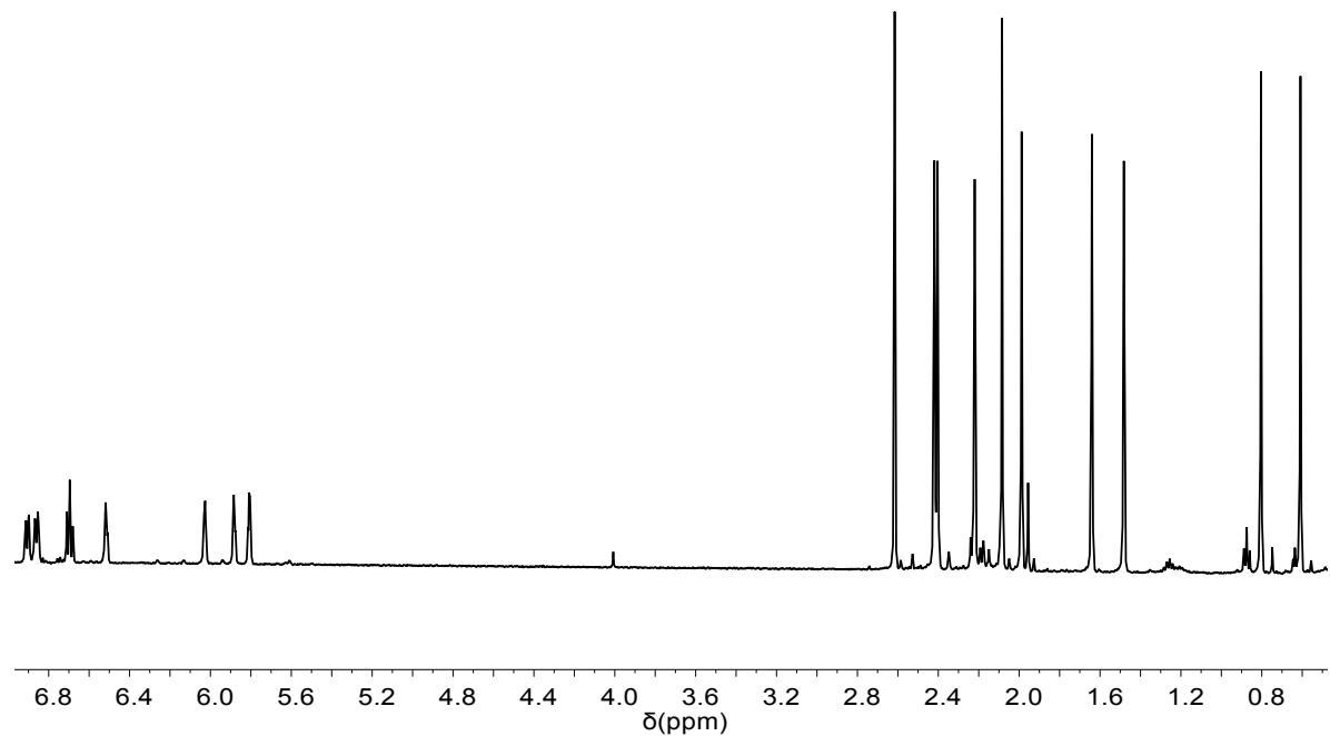
**Fig. S9.**  $^1\text{H}$  NMR spectrum ( $\text{C}_6\text{D}_6$ , 400 MHz, 298 K) of  $Z\text{-Me}_2\text{SB}(\text{Cp},\text{I}^*)\text{ZrCl(O-2,6-Me-C}_6\text{H}_3)$  (**4**).
