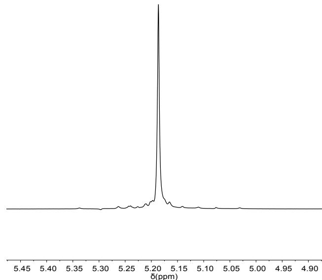
**Fig. S12.**  ${}^1\text{H}\{{}^1\text{H}\}$  NMR spectrum ( $\text{CDCl}_3$ , 500 MHz, 298 K) of the poly-*L*-lactide produced using  ${}^{\text{Me}_2\text{SB}}(\text{Cp},\text{I}^*)\text{ZrCl}_2$  (**1**). Polymerisation conditions: 80 °C,  $[\text{LA}]_0/[\text{M}]_0 = 50$ ,  $[\text{LA}]_0 = 0.5 \text{ M}$  and  $\text{CDCl}_3$ .
