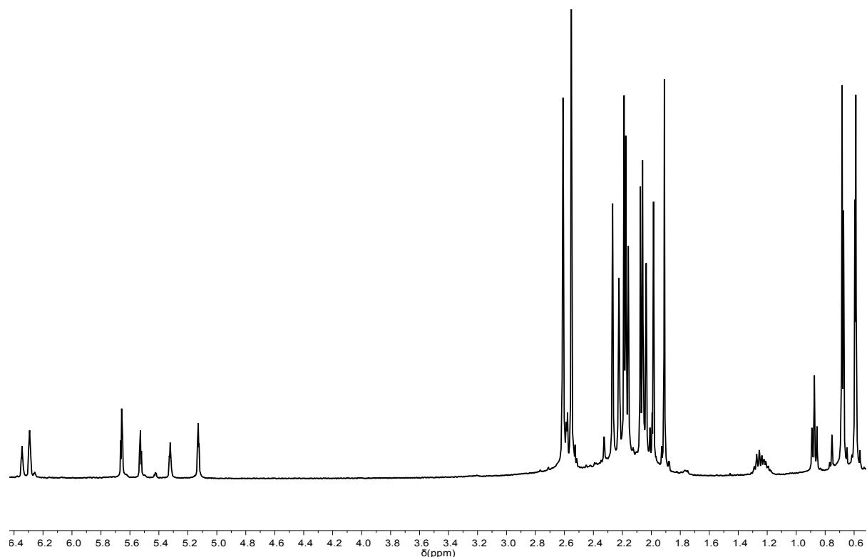
**Fig. S5.**  ${}^1\text{H}$  NMR spectrum ( $\text{C}_6\text{D}_6$ , 400 MHz, 298 K) of  $\text{Me}_2\text{SB}(\text{Cp}^{\text{Me}}, \text{I}^*)\text{ZrCl}_2$  (**2**). Isomers **E-2:Z-2** in 60:40 ratio.
