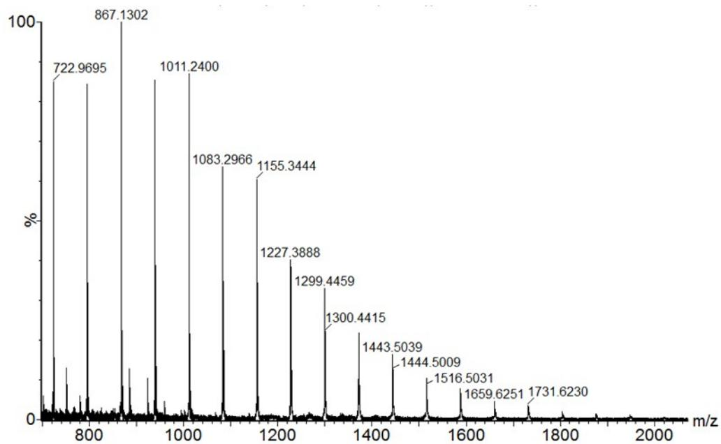
**Fig. S39.** MALDI-TOF mass spectrum recorded in a DCTB + KTFA matrix of the PLA produced from  ${}^{\text{Me}_2}\text{SB}(\text{Cp}^{\text{Me}}, \text{I}^*)\text{ZrCl}_2$  (2) and *L*-lactide. Polymerisation conditions: *L*-lactide (40 mg), 80 °C,  $[\text{LA}]_0/[\text{M}]_0 = 10$ ,  $[\text{LA}]_0 = 0.5$  M and  $\text{CDCl}_3$  (0.56 mL).
