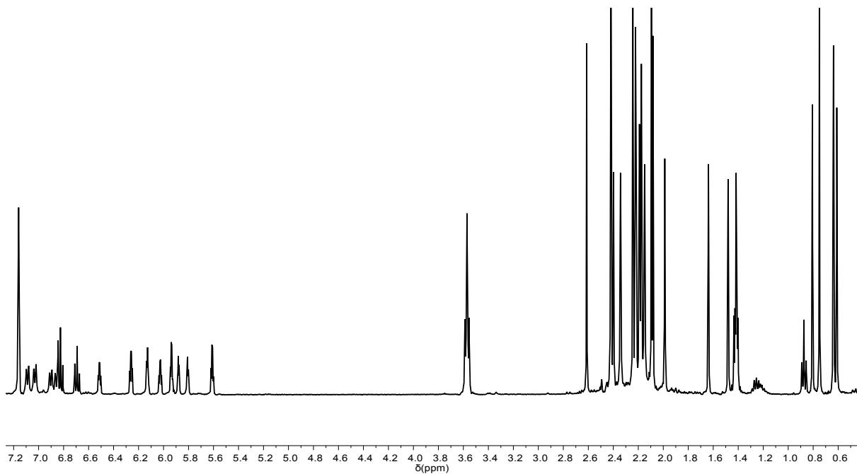
**Fig. S11.** Crude  $^1\text{H}$  NMR spectrum ( $\text{C}_6\text{D}_6$ , 400 MHz, 298 K) of  ${}^{\text{Me}_2\text{S}}\text{B}(\text{Cp},\text{I}^*)\text{ZrCl}(\text{O}-2,6-\text{Me-C}_6\text{H}_3)$  (**4**). Isomers **E-4:Z-4** in 15:85 ratio.
