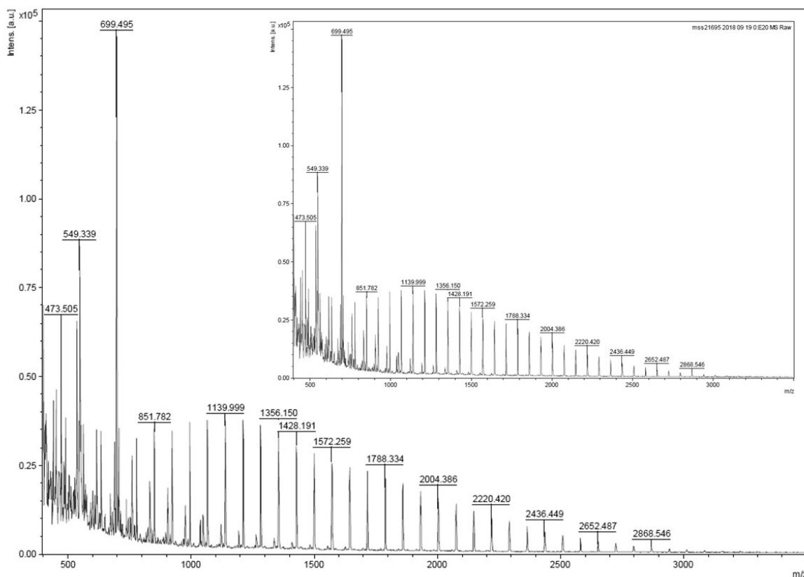
**Fig. S42.** MALDI-TOF mass spectrum recorded in a DHB matrix of PLA produced from  $\text{Me}_2\text{SB}(\text{Cp},\text{I}^*)\text{ZrCl(O-2,6-Me-C}_6\text{H}_3)$  (**4**) and *rac*-lactide. Polymerisation conditions: *rac*-lactide (40 mg), 80 °C,  $[\text{LA}]_0/[\text{M}]_0 = 10$ ,  $[\text{LA}]_0 = 0.5 \text{ M}$  and  $\text{CDCl}_3$  (0.95 mL).
