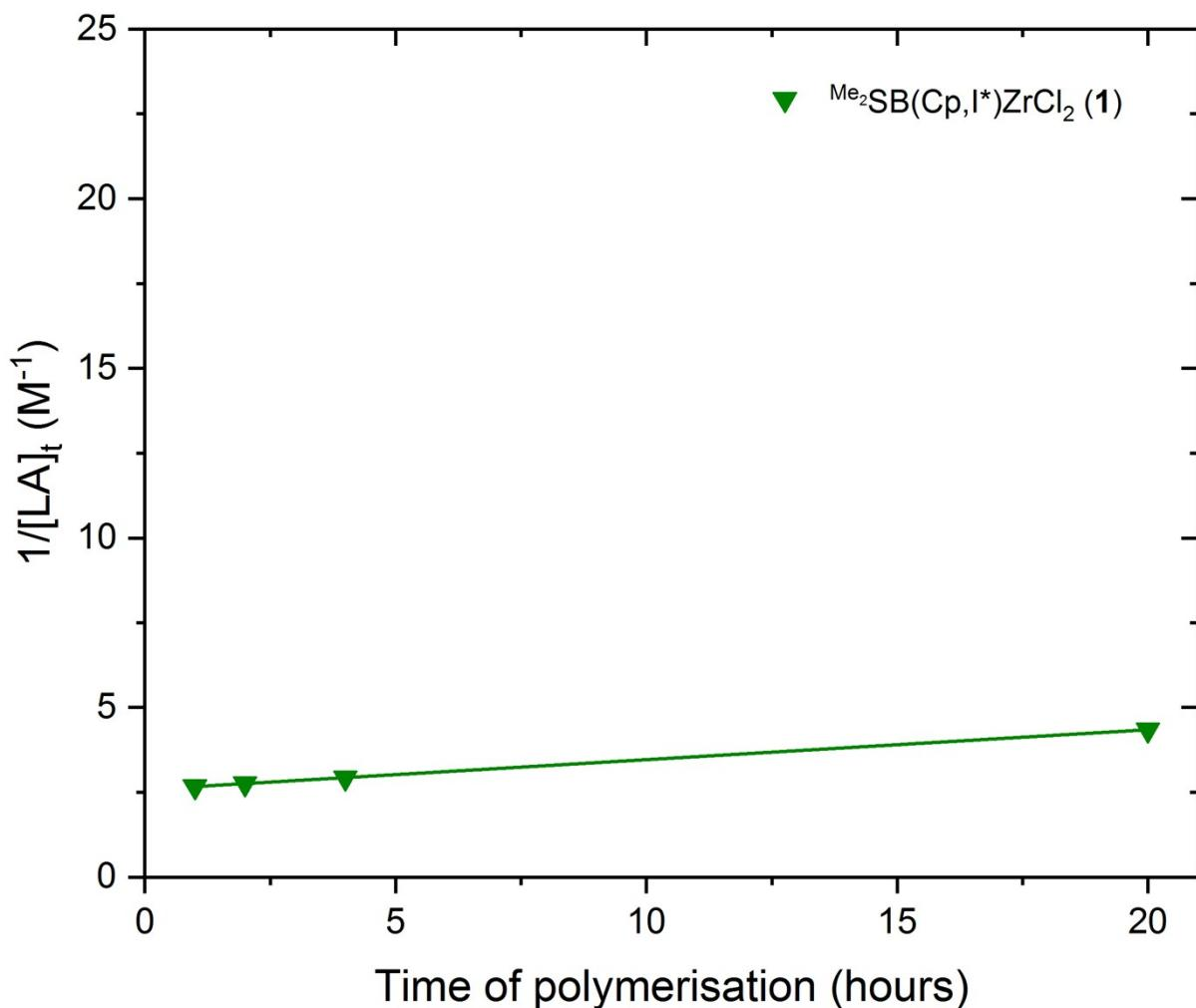
**Fig. S43.** *L*-Lactide polymerisation with  $^{Me_2}SB(Cp,I^*)ZrCl_2$  (**1**) (green down triangle,  $k_{obs} = 0.08 \pm 0.01 M^{-1} h^{-1}$ ). Polymerisation conditions: *L*-lactide (40 mg), 80 °C, toluene (5.5 mL),  $[LA]_0/[M]_0 = 50$ ,  $[LA]_0 = 0.05 M$ , 2 equivalents of benzyl alcohol as co-initiator.
