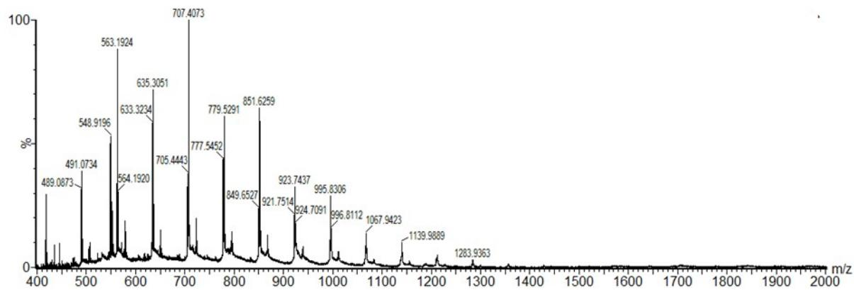
**Fig. S40.** MALDI-TOF mass spectrum recorded in a DHB matrix of PLA produced from  ${}^{\text{Me}_2}\text{SB}(\text{Cp}^{\text{Me}}, \text{I}^*)\text{ZrCl}_2$  (2) and *rac*-lactide. Polymerisation conditions: *rac*-lactide (40 mg) 80 °C,  $[\text{LA}]_0/[\text{M}]_0 = 10$ ,  $[\text{LA}]_0 = 0.5$  M and  $\text{CDCl}_3$  (0.56 mL).
