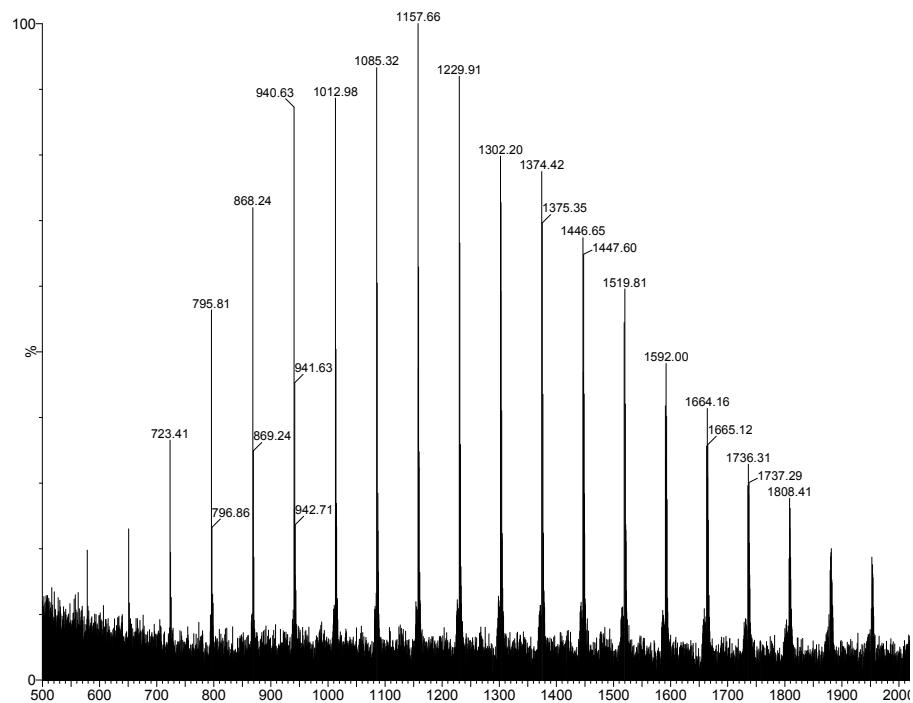
**Fig. S36.** MALDI-TOF mass spectrum recorded in a DCTB + KTFA matrix of the PLA produced from  $^{Me_2}SB(Cp,I^*)ZrCl_2$  (1) and *L*-lactide. Polymerisation conditions: *L*-lactide (40 mg), 80 °C,  $[LA]_0/[M]_0 = 10$ ,  $[LA]_0 = 0.5$  M and  $CDCl_3$  (0.56 mL).
