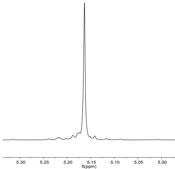
**Fig. S14.**  $^1\text{H}\{^1\text{H}\}$  NMR spectrum ( $\text{CDCl}_3$ , 500 MHz, 298 K) of the poly-*D*-lactide produced using  ${}^{\text{Me}_2}\text{SB}(\text{Cp},\text{I}^*)\text{ZrCl}_2$  (**1**). Polymerisation conditions: 80 °C,  $[\text{LA}]_0/[\text{M}]_0 = 50$ ,  $[\text{LA}]_0 = 0.5 \text{ M}$  and  $\text{CDCl}_3$ .
