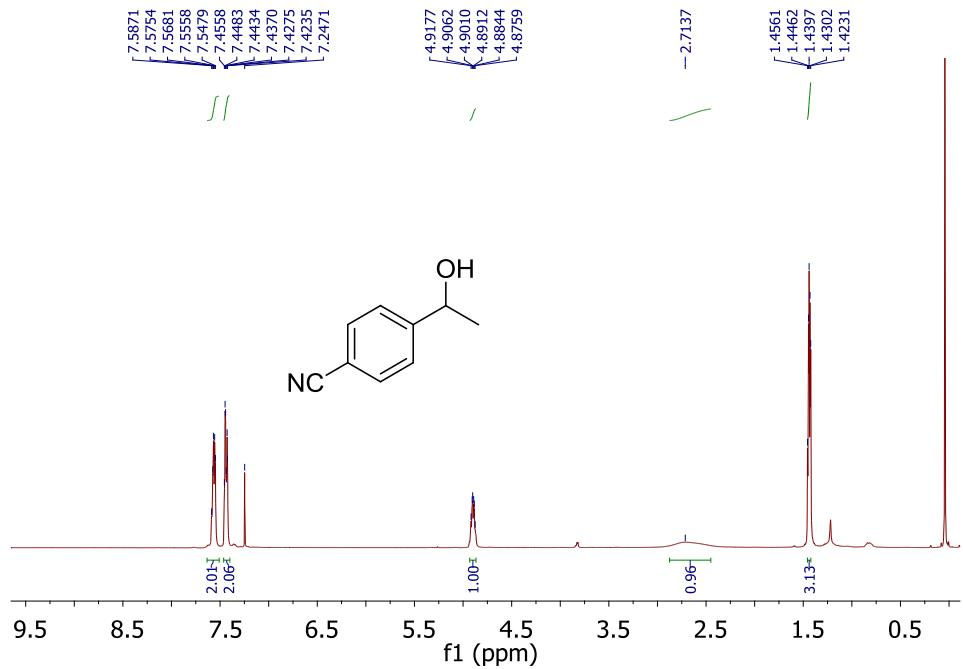
**Fig. S45**  $^1\text{H}$  NMR Spectrum of **5k** in  $\text{CDCl}_3$  (400 MHz).
