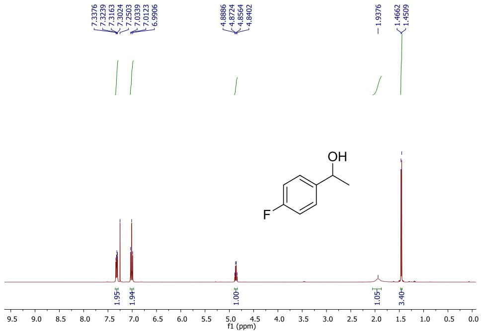
**Fig. S41** <sup>1</sup>H NMR Spectrum of **5g** in CDCl<sub>3</sub> (400 MHz).
