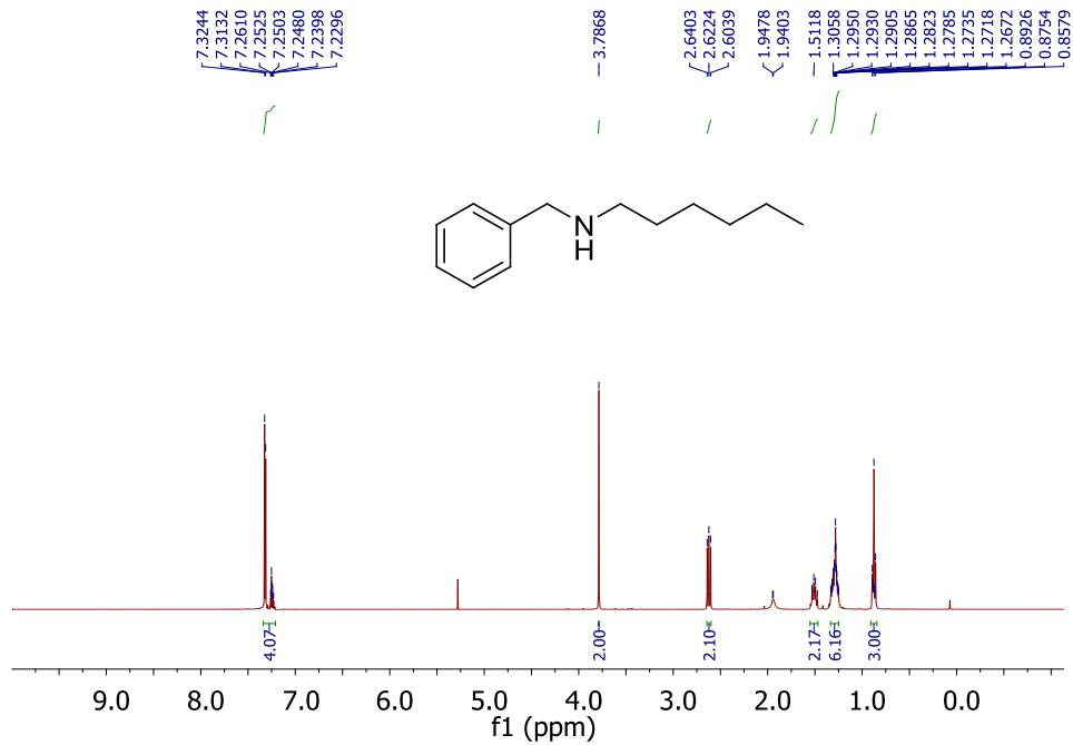
**Fig. S89**  $^1\text{H}$  NMR Spectrum of **8j** in  $\text{CDCl}_3$  (400 MHz).
