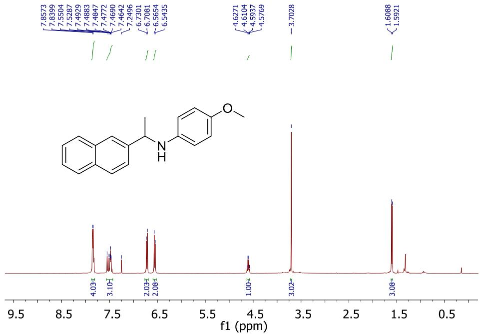
**Fig. S83**  $^1\text{H}$  NMR Spectrum of **8g** in  $\text{CDCl}_3$  (400 MHz).
