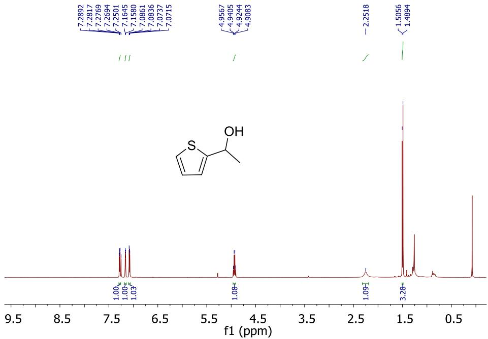
**Fig. S53**  $^1\text{H}$  NMR Spectrum of **5r** in  $\text{CDCl}_3$  (400 MHz).
