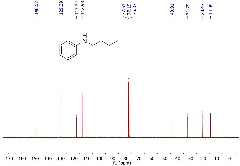
**Fig. S88**  $^{13}\text{C}$  NMR Spectrum of **8i** in  $\text{CDCl}_3$  (100 MHz).
