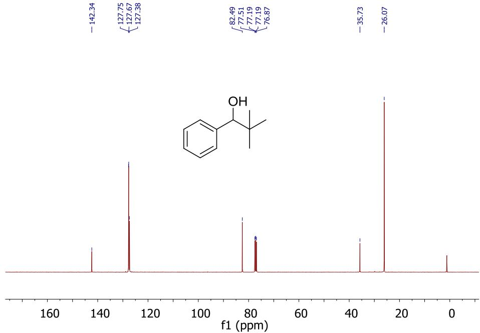
**Fig. S52** <sup>13</sup>C NMR Spectrum of **5o** in CDCl<sub>3</sub> (100 MHz).
