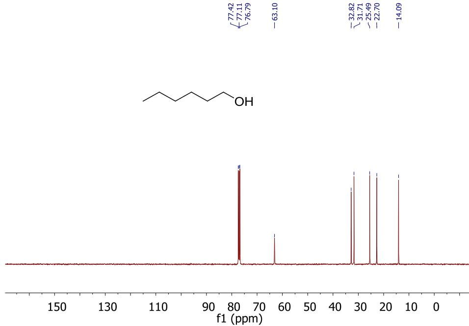
**Fig. S70**  $^{13}\text{C}$  NMR Spectrum of **7h** in  $\text{CDCl}_3$  (100 MHz).
