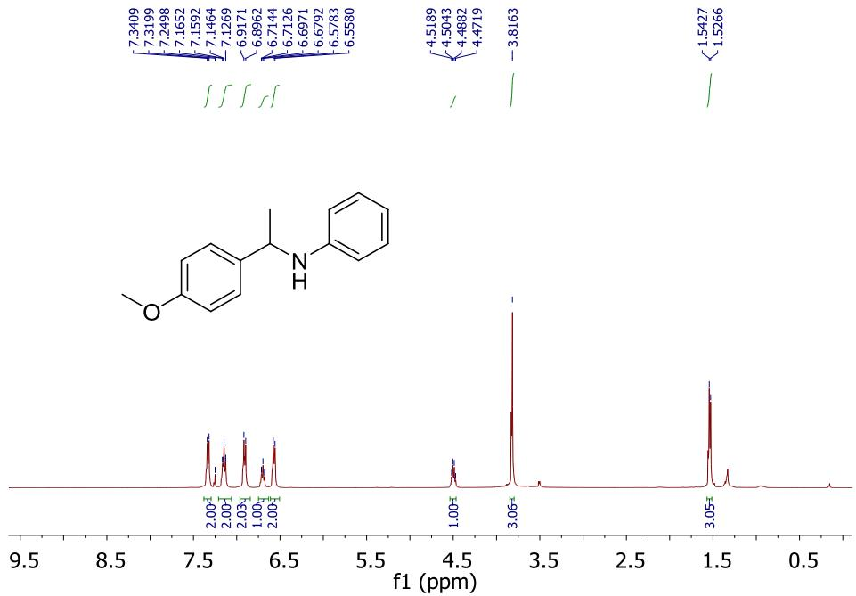
**Fig. S81**  $^1\text{H}$  NMR Spectrum of **8f** in  $\text{CDCl}_3$  (400 MHz).
