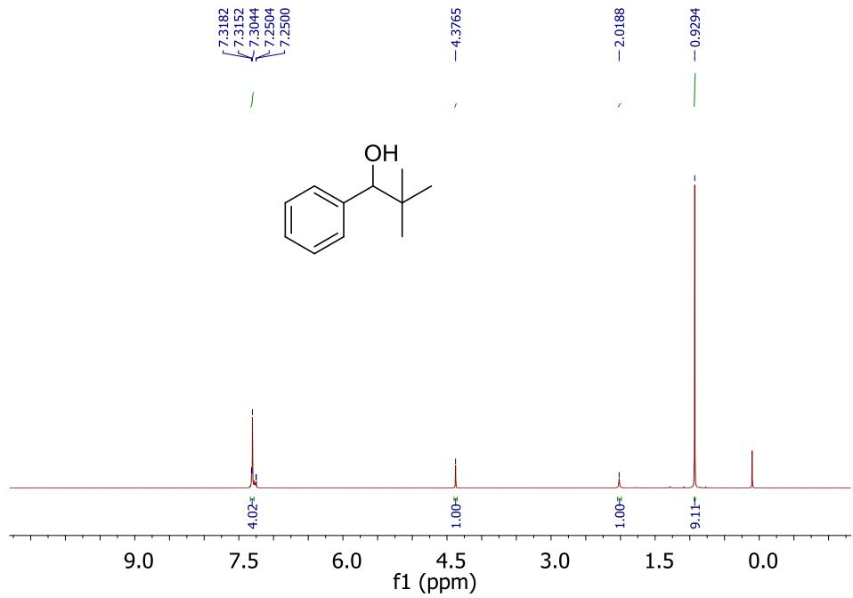
**Fig. S51** <sup>1</sup>H NMR Spectrum of **5o** in CDCl<sub>3</sub> (400 MHz).
