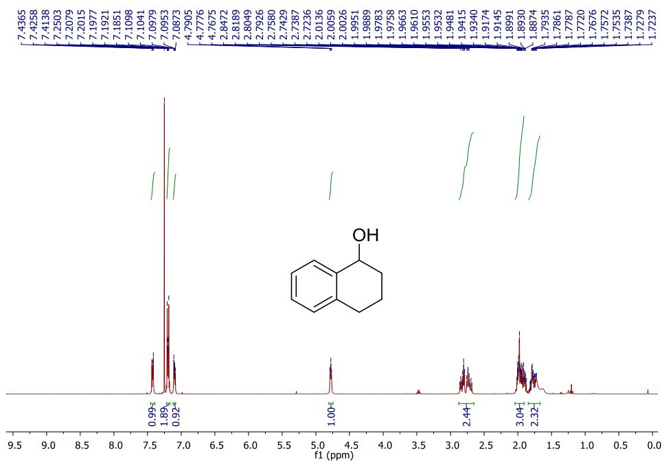
**Fig. S57** <sup>1</sup>H NMR Spectrum of **6a** in CDCl<sub>3</sub> (400 MHz).
