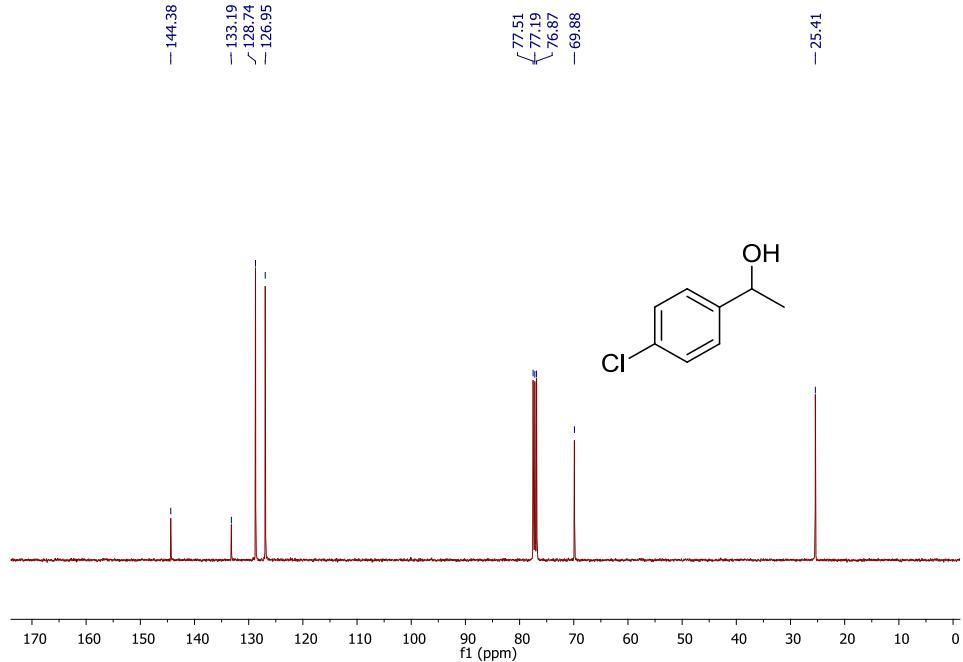
**Fig. S44** <sup>13</sup>C NMR Spectrum of **5h** in CDCl<sub>3</sub> (100 MHz).
