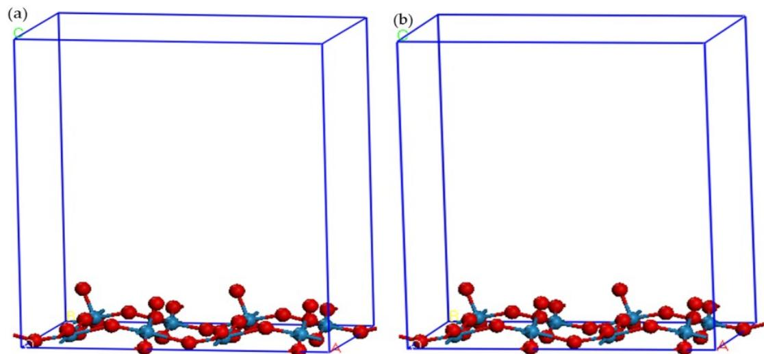
**Fig. S4.** Schematic drawing of supercell model for  $\text{WO}_3(020)$  surface: (a) before relaxation, (b) after relaxation.
