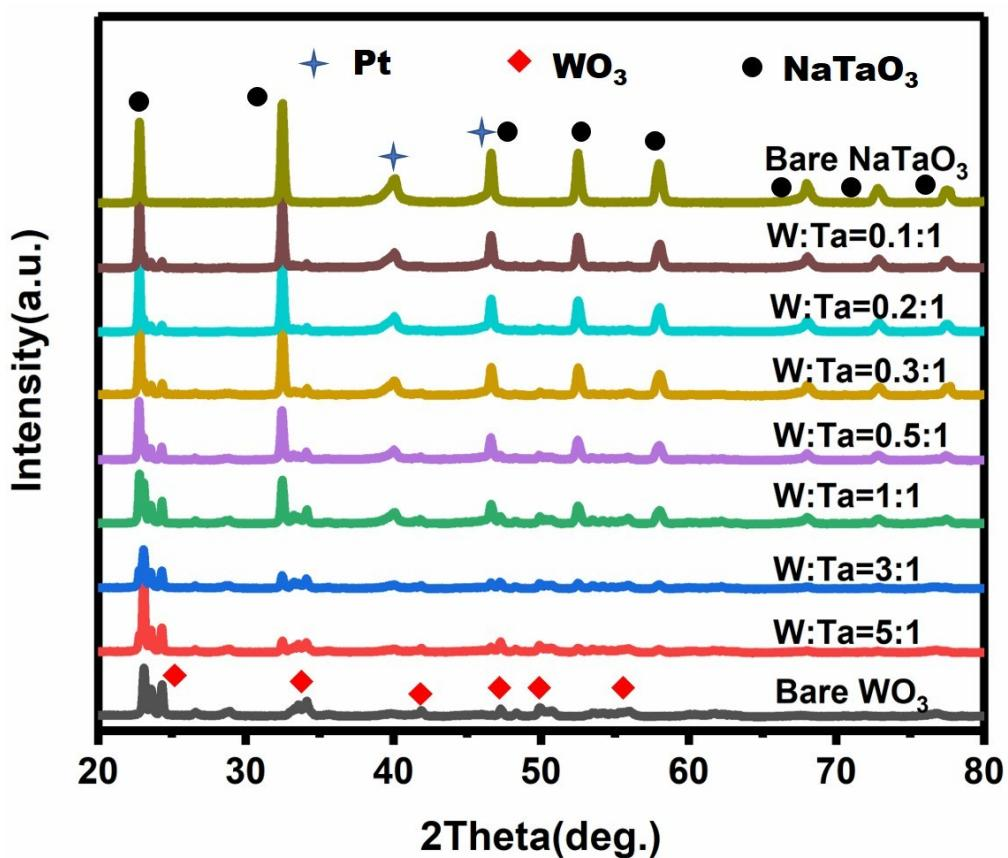
**Fig. S1.** XRD patterns of Pt/ $\text{WO}_3$ , Pt/ $\text{NaTaO}_3$ , and Pt/ $\text{WO}_3$ - $\text{NaTaO}_3$  composites with different molar ratio (W:Ta = 5:1, 3:1, 1:1, 0.5:1, 0.3:1, 0.2:1, 0.1:1).
