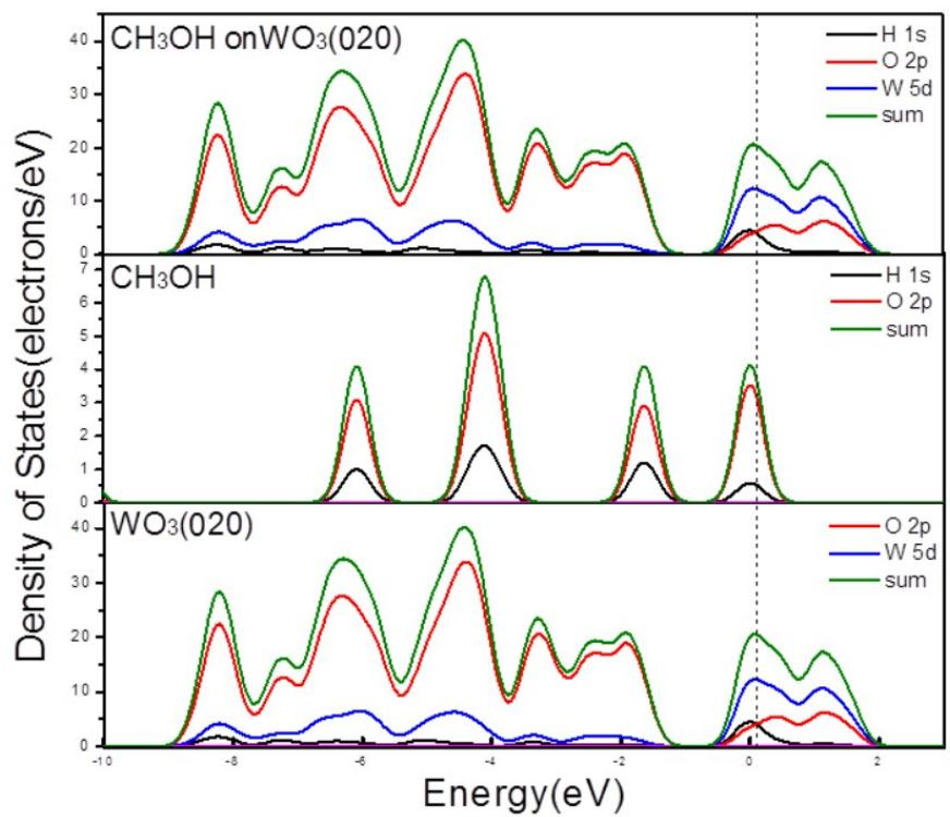
**Fig. S5.** Density of state for  $\text{CH}_3\text{OH}$  molecule adsorbed on W-top site of  $\text{WO}_3(020)$ .
