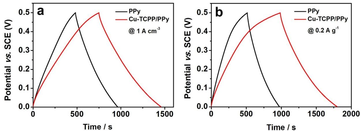
**Fig. S3** GCD curves of Cu-TCPP/PPy (The electrophoretic deposition time of Cu-TCPP is 30 s. The Electrochemical polymerization time is 600 s.) and PPy films at a current density of 1 mA cm<sup>-3</sup> (a) and 0.2 A g<sup>-1</sup> (b).
