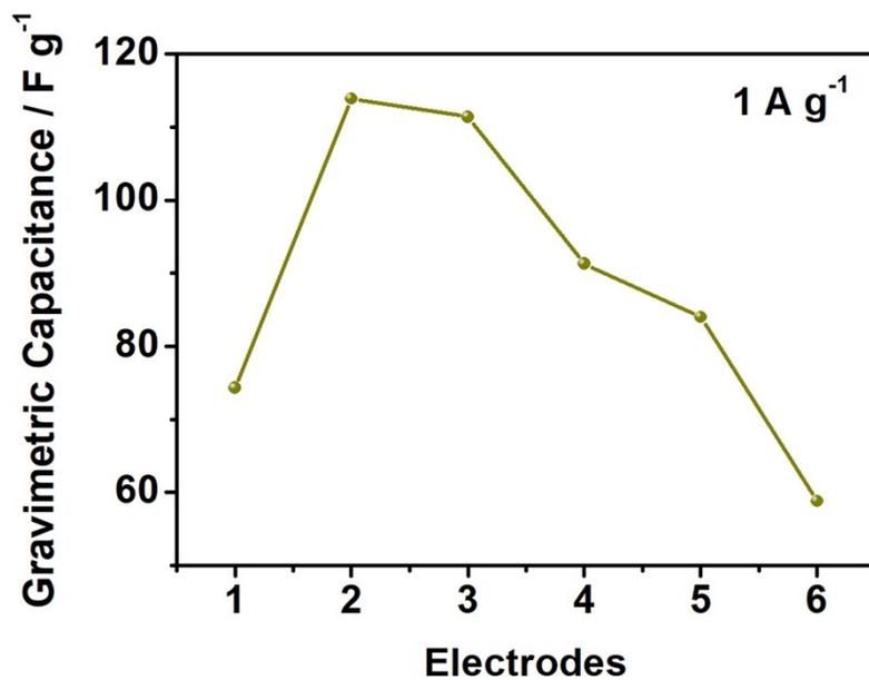
**Fig. S5** Gravimetric capacitance of different Cu-TCPP/PPy electrodes through the electrophoretic deposition of wrinkled ultrathin 2D Cu-TCPP nanosheets for a certain time of 0 s (1), 30 s (2), 1 min (3), 3 min (4), 5 min (5) and 10 min (6) and electrochemical polymerization of PPy at 0.8 V versus Ag/AgCl for 600 s. Current density:  $1 A g^{-1}$ .
