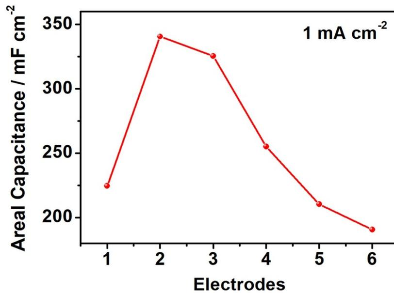
**Fig. S4** Areal capacitance of different Cu-TCPP/PPy electrodes through the electrophoretic deposition of wrinkled ultrathin 2D Cu-TCPP nanosheets for a certain time of 0 s (1), 30 s (2), 1 min (3), 3 min (4), 5 min (5) and 10 min (6) and electrochemical polymerization of PPy at 0.8 V versus Ag/AgCl for 600 s. Current density: 1 mA cm<sup>-2</sup>.
