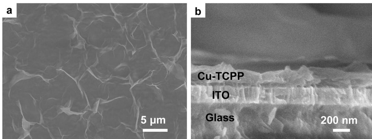
**Fig. S1** SEM images of the flat ultrathin 2D Cu-TCPP film through the electrophoretic deposition of the flat ultrathin 2D Cu-TCPP nanosheets onto the surface of ITO-coated glass for 30 s. (a) The top-view SEM image. There are no macroporous structure existing in the film. (b) The cross-sectional SEM image. It shows that the flat ultrathin Cu-TCPP nanosheets tightly stack.
