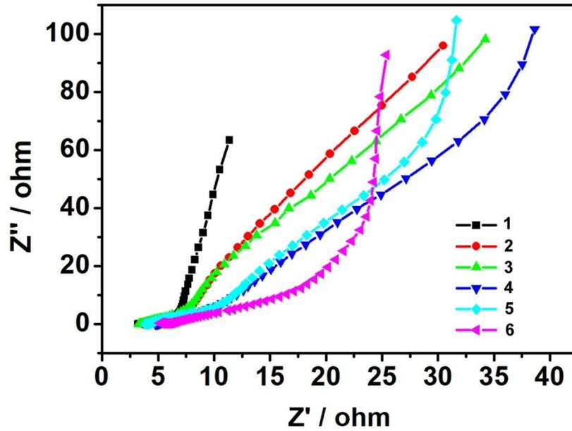
**Fig. S6** Electrochemical impedance spectroscopy of different Cu-TCPP/PPy electrodes through the electrophoretic deposition of wrinkled 2D ultrathin Cu-TCPP nanosheets for a certain time of 0 s (1), 30 s (2), 1 min (3), 3 min (4), 5 min (5) and 10 min (6) and electrochemical polymerization of PPy at 0.8 V versus Ag/AgCl for 600 s. Frequency range: 0.01 Hz~10 kHz. Electrolyte: 0.5 M H<sub>2</sub>SO<sub>4</sub>.
