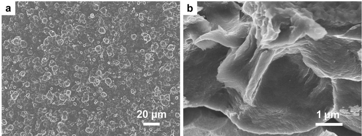
**Fig. S8** (a) The top-view SEM image and (b) cross-sectional SEM image of the Cu-TCP/PPy film after cycling test.
