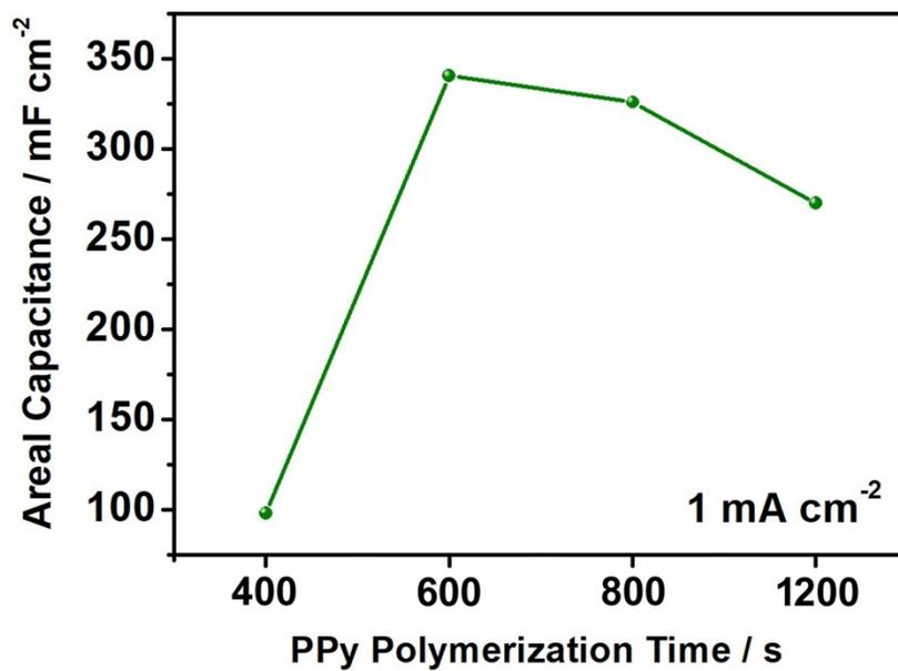
**Fig. S7** Areal capacitance of different Cu-TCPP/PPy electrodes through the electrophoretic deposition of wrinkled ultrathin 2D Cu-TCPP nanosheets for 30 s and electrochemical polymerization of PPy at 0.8 V versus Ag/AgCl for a certain time of 400 s, 600 s, 900 s and 1200 s. Current density:  $1 \text{ mA cm}^{-2}$ .
