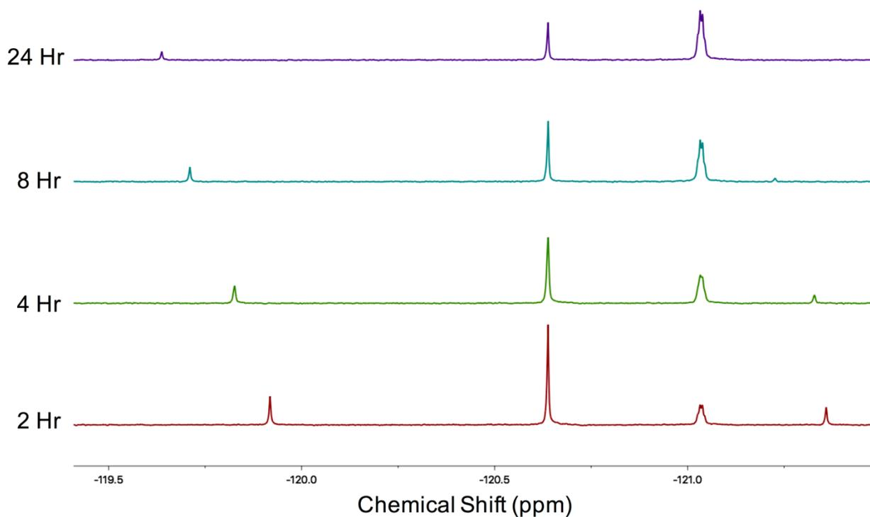
**Figure S5.** A time series of  $^{19}\text{F}\{^1\text{H}\}$  NMR spectra when complex [1] is incubated with N-Ac-Cys-OMe (2 mM Ru, 3 eq. amino acid, 310 K).
