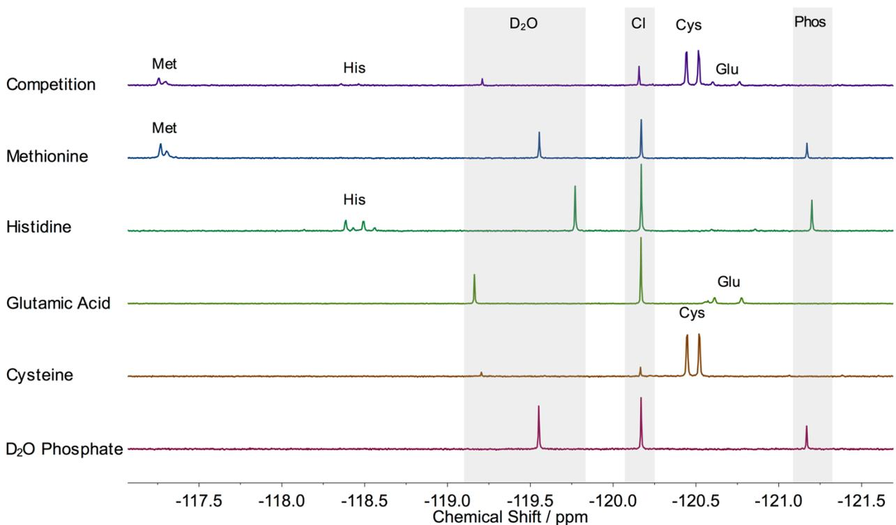
**Figure S8.** A series of  $^{19}\text{F}\{^1\text{H}\}$  NMR spectra when complex [3] is incubated with the protected amino acids, N-Ac-Cys-OMe, N-Z-Glu-OMe, N-Bz-His-OMe, N-Ac-Met-OMe, and a mixture of all amino acids together, (2 mM Ru, 3 eq. amino acid, 24 hr, 310 K).
