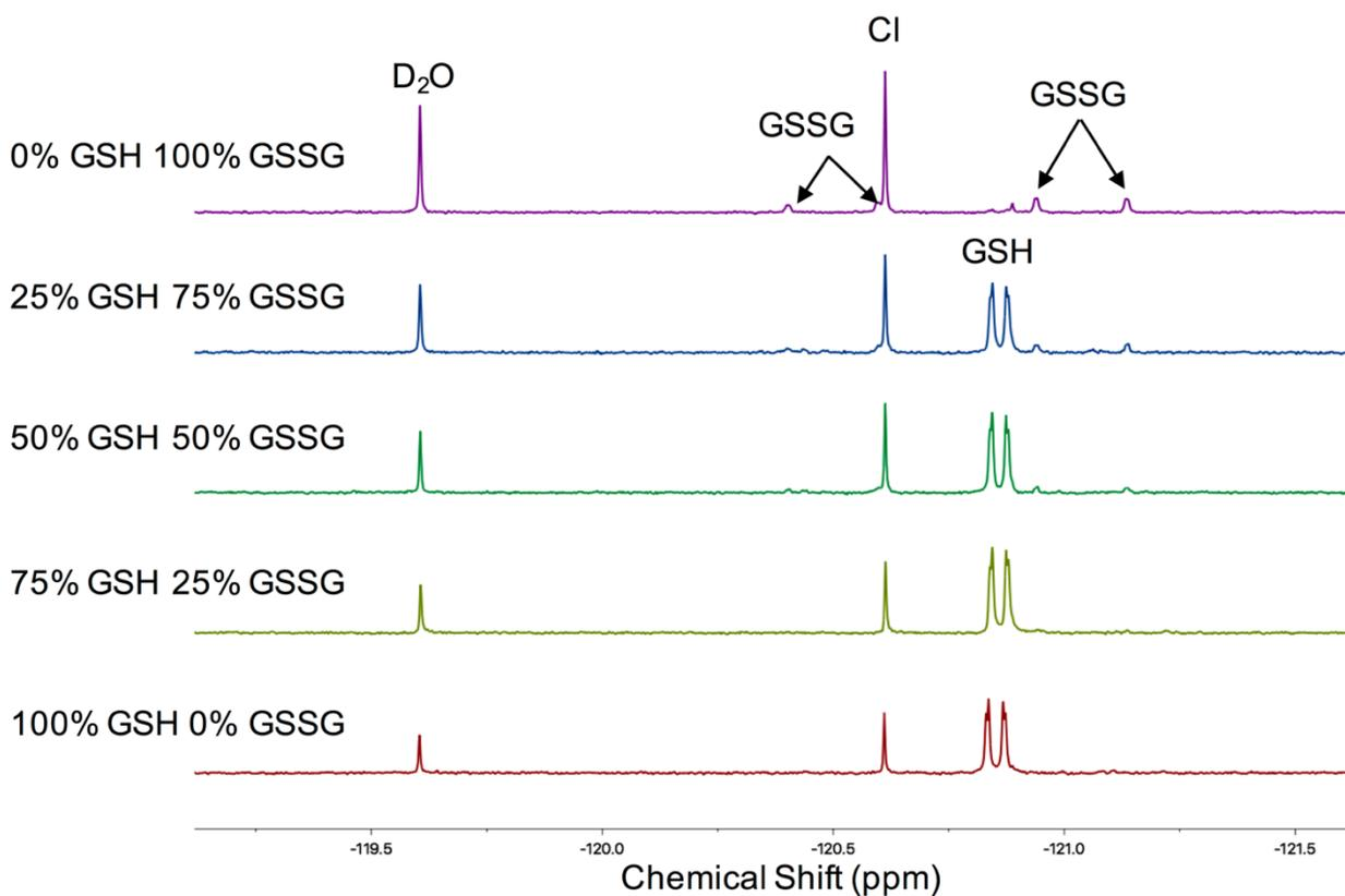
**Figure S11.** A series of  $^{19}\text{F}\{^1\text{H}\}$  NMR spectra when complex [2] is incubated with defined mixtures of reduced and oxidised glutathione (2 mM Ru, 3 eq. glutathione, 24 hr, 310 K).
