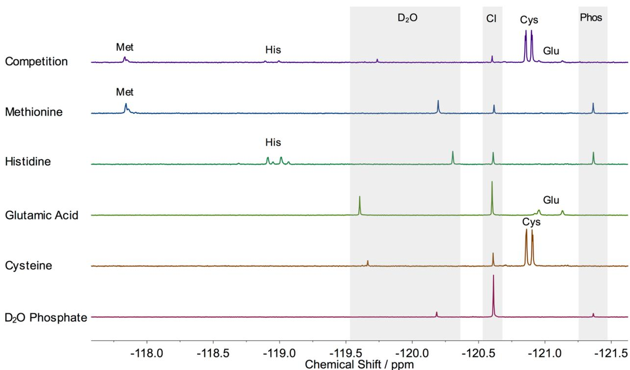
**Figure S7.** A series of  $^{19}\text{F}\{^1\text{H}\}$  NMR spectra when complex [2] is incubated with the protected amino acids, N-Ac-Cys-OMe, N-Z-Glu-OMe, N-Bz-His-OMe, N-Ac-Met-OMe, and a mixture of all amino acids together, (2 mM Ru, 3 eq. amino acid, 24 hr, 310 K).
