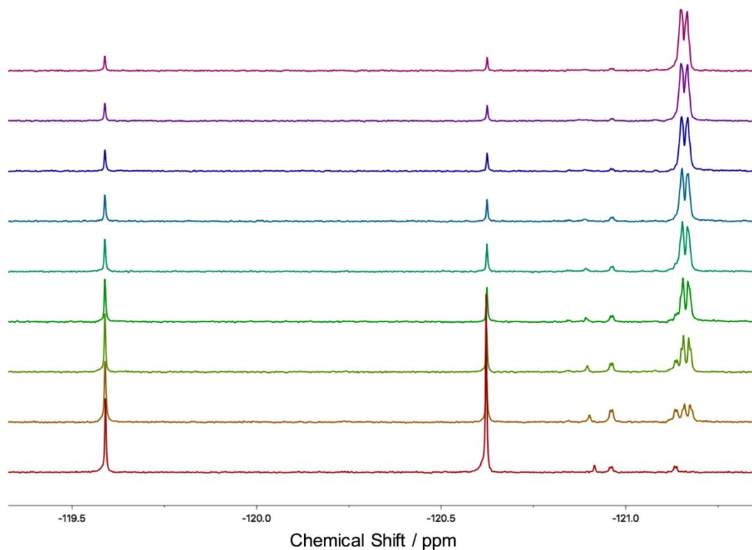
**Figure S10.** A time series of  $^{19}\text{F}\{^1\text{H}\}$  NMR spectra when complex [1] is incubated with N-Ac-Cys-OOH (2 mM Ru, 3 eq. amino acid, 310 K, 0 – 24 hr).
