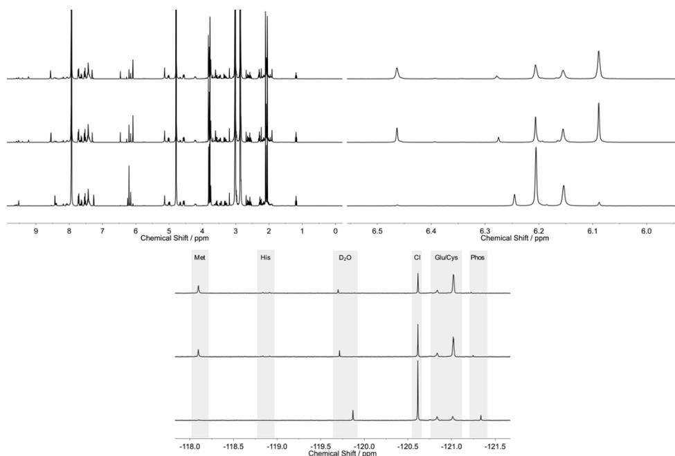
**Figure S6.** A comparison of  $^{19}\text{F}\{^1\text{H}\}$  NMR (bottom) and  $^1\text{H}$  spectra (top) when complex [1] is incubated with a mixture protected amino acids, N-Ac-Cys-OMe, N-Z-Glu-OMe, N-Bz-His-OMe, N-Ac-Met-OMe, and a mixture of all amino acids together, (4 mM Ru, 1.5 eq. each amino acid, 310 K).
