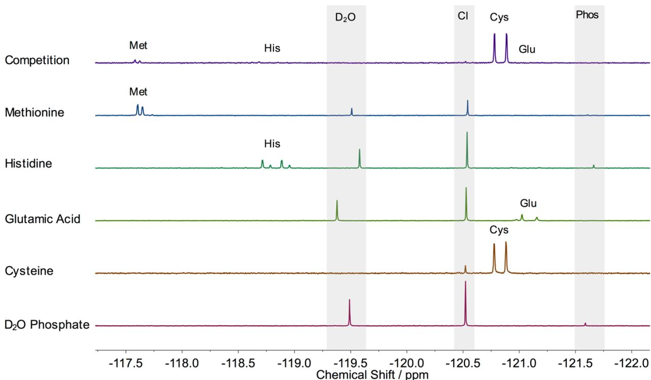
**Figure S9.** A series of  $^{19}\text{F}\{^1\text{H}\}$  NMR spectra when complex [4] is incubated with the protected amino acids, N-Ac-Cys-OMe, N-Z-Glu-OMe, N-Bz-His-OMe, N-Ac-Met-OMe, and a mixture of all amino acids together, (2 mM Ru, 3 eq. amino acid, 24 hr, 310 K).
