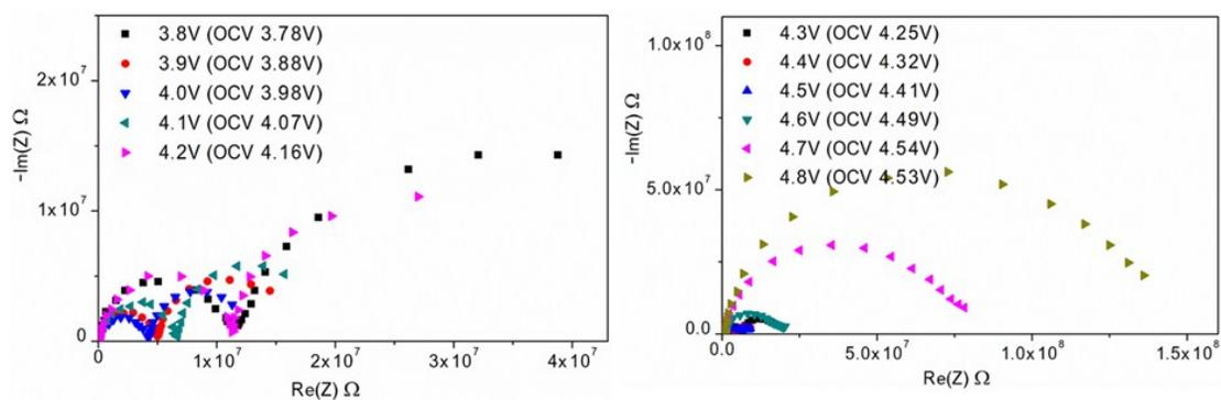
**Fig. S6.** The EIS spectra of a PVdF-coated NCA particle vary with specific charge voltage from 3.8V to 4.8V.
