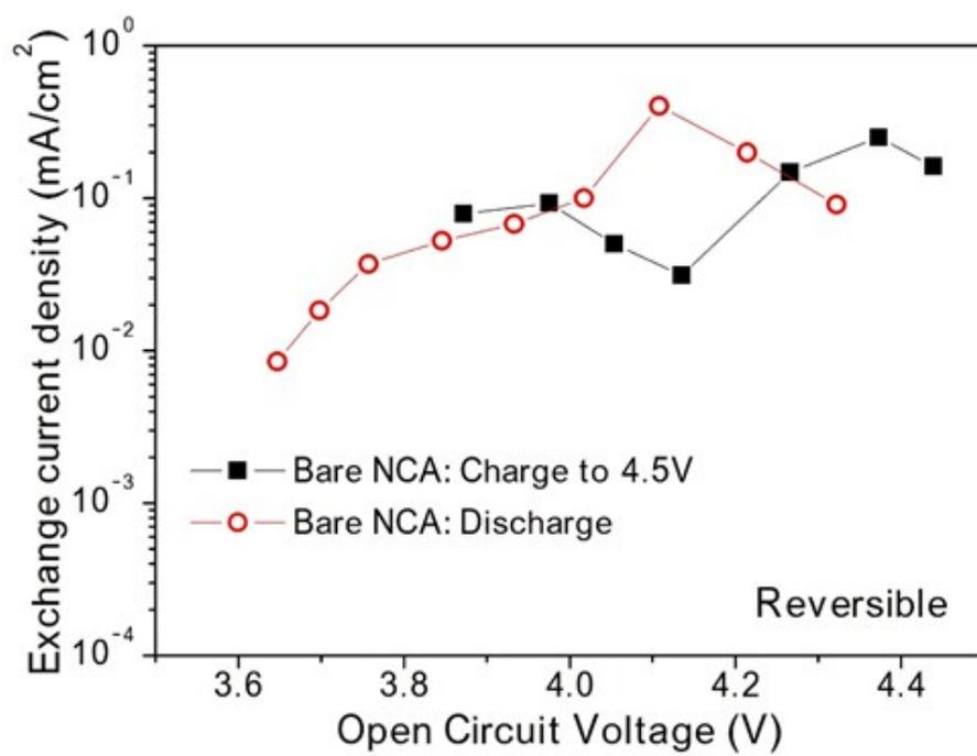
**Fig. S4.** Reversibility is observed in  $j_0$  between charge and discharge for bare NCA charged to the lower voltage (4.5V).
