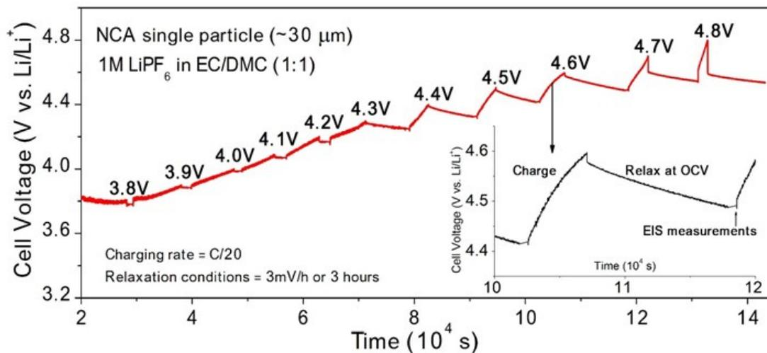
**Fig. S2.** Voltage vs. time during galvanostatic step-charging at C/20 rate of a single NCA ( $\text{Li}_{1-x}\text{Ni}_{0.8}\text{Co}_{0.15}\text{Al}_{0.05}\text{O}_2$ ) particle. Each galvanostatic step is followed by voltage relaxation under open circuit conditions.
