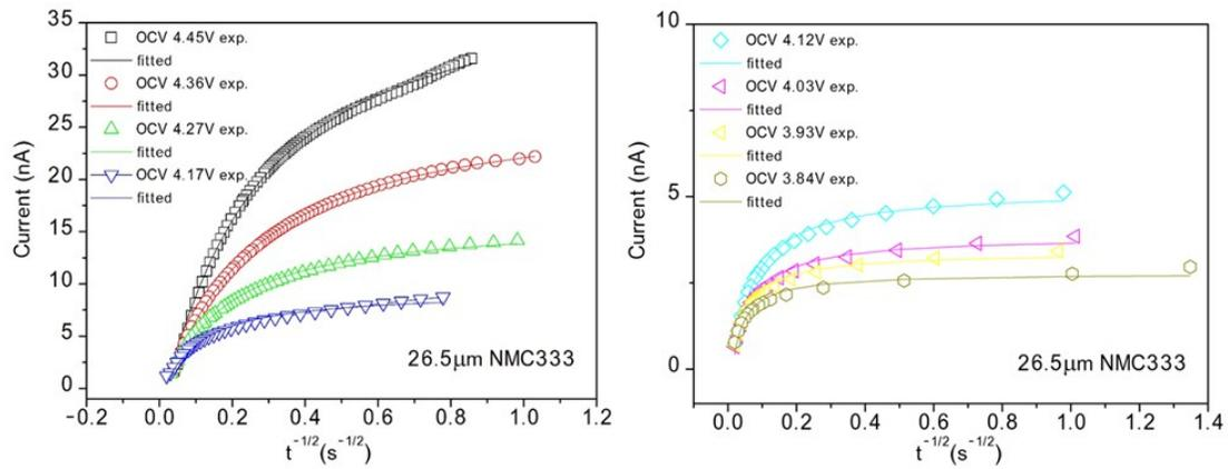
**Fig. S5.** PITT current vs time data, and corresponding least-squares fit from which kinetic parameters are obtained, for an NMC333 particle of 26.5 μm diameter, measured for a +15 mV voltage step from various relaxed OCV.
