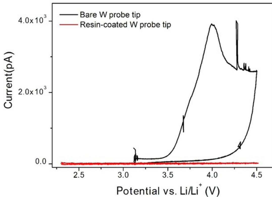
**Fig. S1.** Cyclic voltammogram for tungsten probe with and without coating by amorphous fluoropolymer (CYTOP), showing suppression of tungsten oxidation side-reaction for the coated probe.
