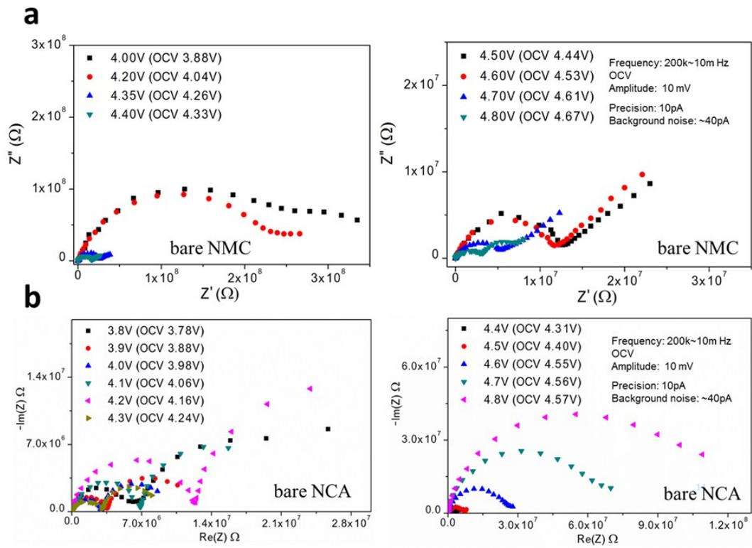
**Fig. S3.** The EIS spectra of (a) bare NMC and (b) bare NCA vary with specific charge voltage from 3.8V to 4.8V
