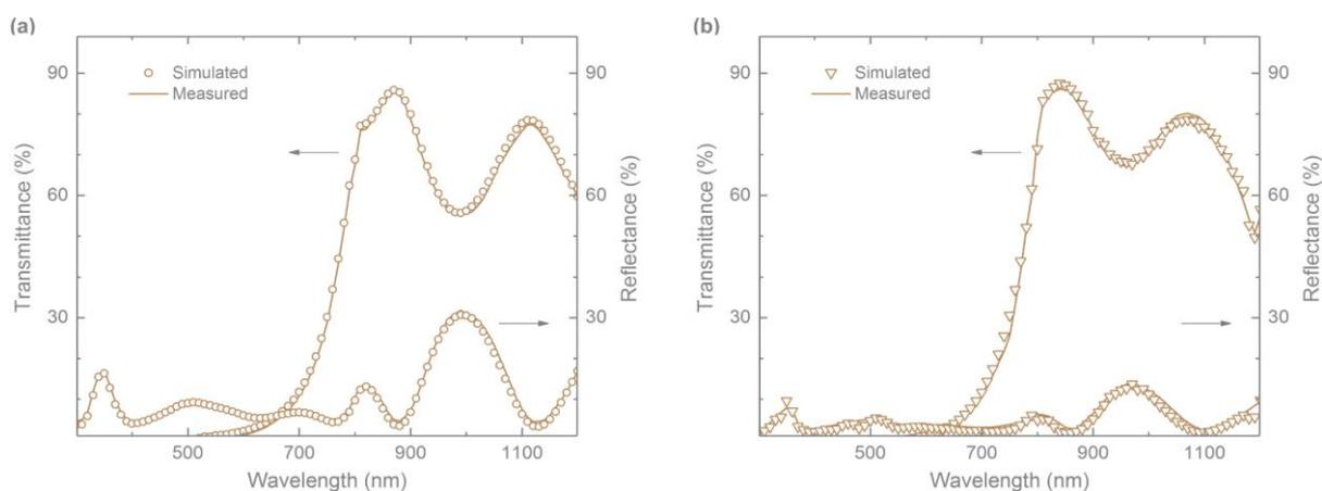
**Figure S1:** Simulated and measured transmittance, reflectance spectra of semi-transparent perovskite solar cell (a) without textured film and (b) with textured film. The spectra of solar cells and solar modules are identical.
