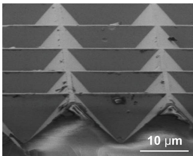
**Figure S2:** Scanning electron microscopy image of the textured film with inverted pyramids.
