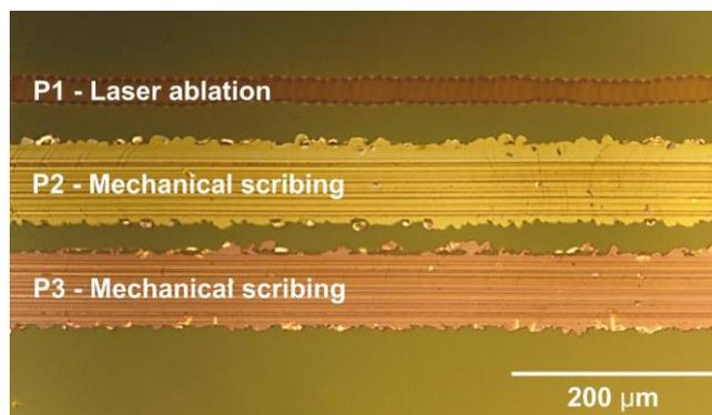
**Figure S9:** Optical microscopy image of P1, P2, and P3 scribes of the perovskite solar module.
