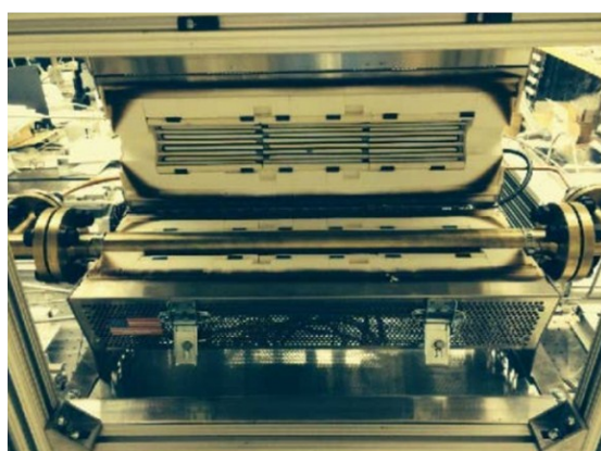
Figure S5. CO catalytic bed reactor: Photographs of the a) rear view of the reactor assembly, b) recuperative heat exchanger, c) furnace and data acquisition system, and d) furnace opened with the view of the reactor chamber.
