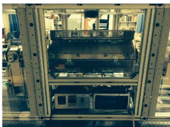
Figure S5. CO catalytic bed reactor: Photographs of the a) rear view of the reactor assembly, b) recuperative heat exchanger, c) furnace and data acquisition system, and d) furnace opened with the view of the reactor chamber.
