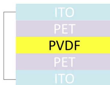
Figure S1. Sample used for piezo-regime tests to measure current and voltage where PVDF film is sandwiched between insulative PET layers. Conductive ITO electrode layers are below PET. Piezo-regime tests are used to demonstrate that the electrostatic induction can be driven by piezoelectric charges.
