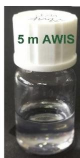
**Figure S13.** Photographs showing the state of 5 m AWIS electrolyte at -50 °C.
