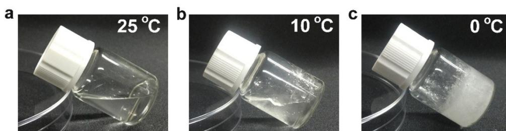
**Figure S12.** Photographs showing the state of 21 m WIS electrolyte at different temperatures.
