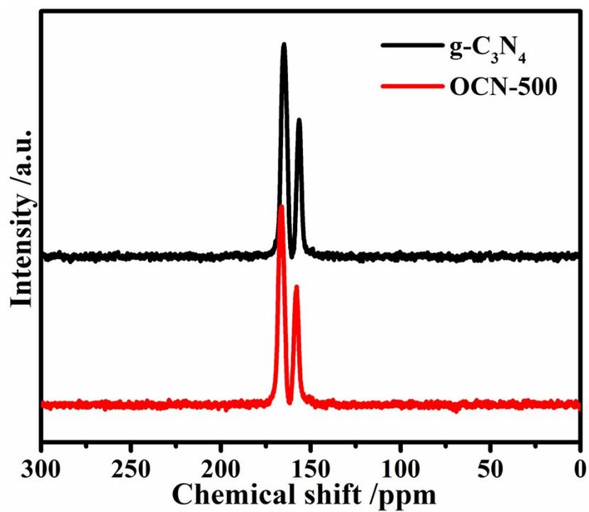
Fig. S14 Solid-state <sup>13</sup>C CP-MAS NMR of g-C<sub>3</sub>N<sub>4</sub> and OCN-500.
