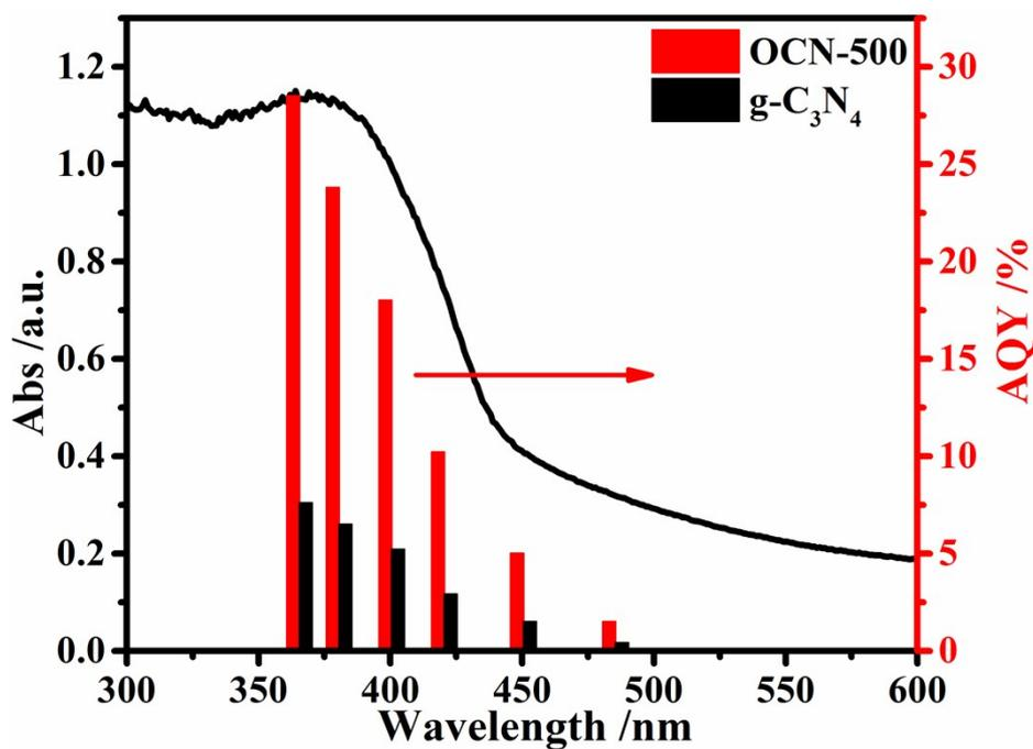
Fig. S23 Diffuse reflectance absorption spectra (left axis) of OCN-500 and apparent quantum yield (AQY, right axis) of g-C<sub>3</sub>N<sub>4</sub> and OCN-500 photocatalytic H<sub>2</sub>O<sub>2</sub> production with monochromatic light irradiation. The experimental conditions were as follows: 1 g/L of photocatalyst, 10 vol % of isopropyl alcohol, and O<sub>2</sub>-saturated.
