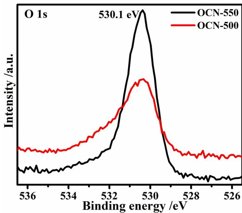
Fig. S16 O 1s high-resolution XPS spectra of OCN-500 and OCN-550.
