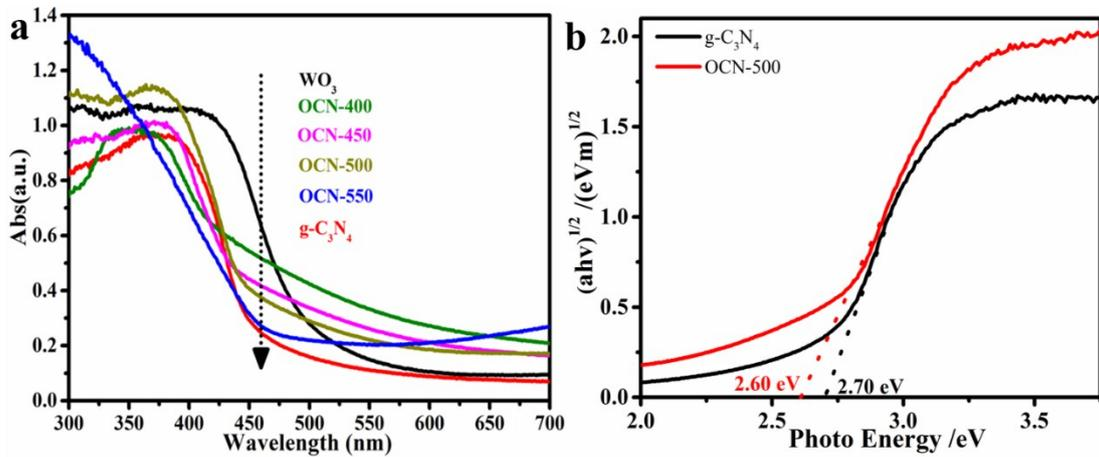
Fig. S11 (a) Diffuse reflectance absorption spectra of the samples; (b) gap energies of g-C<sub>3</sub>N<sub>4</sub> and OCN-500.
