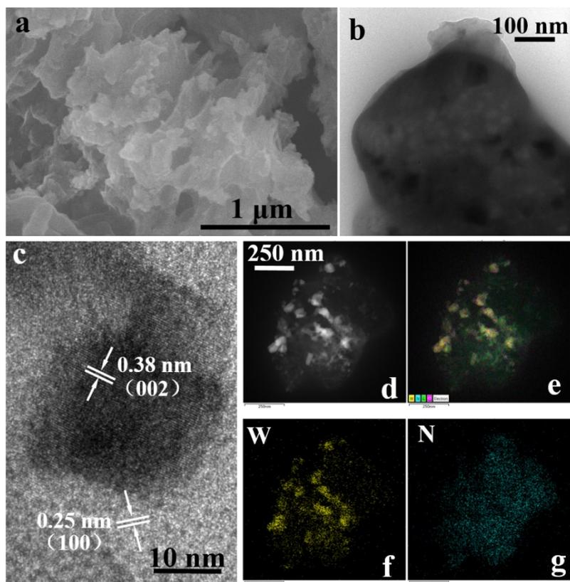
Fig. S7 (a) FE-SEM images of OCN-500; (b) TEM images of OCN-500; (c) HR-TEM images of OCN-500; (d) HAADF-STEM images of OCN-500, EDS mapping results W (f) and N (g) and overlay of HAADF-STEM of W (yellow) and N (blue) elements of OCN-500 (e).
