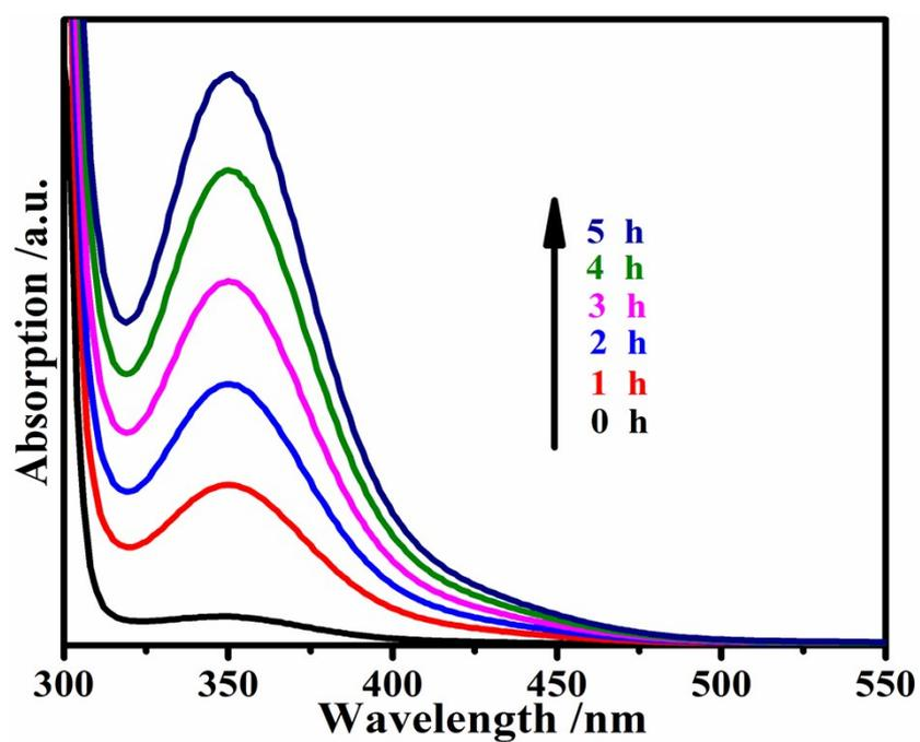
Fig. S18 UV-vis absorption spectrum changes of H<sub>2</sub>O<sub>2</sub> generation of OCN-500 in isopropyl alcohol under visible light irradiation.
