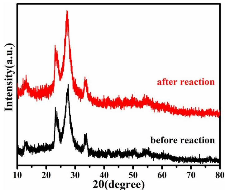
Fig. S21 XRD patterns of OCN-500 after 4 cycles of the photocatalytic generation of H<sub>2</sub>O<sub>2</sub> with 10% isopropyl alcohol under visible light irradiation.
