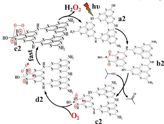
Fig. S2 The mechanism of OCN model (-OH) photocatalytic O<sub>2</sub> reduction to synthesis H<sub>2</sub>O<sub>2</sub>.
