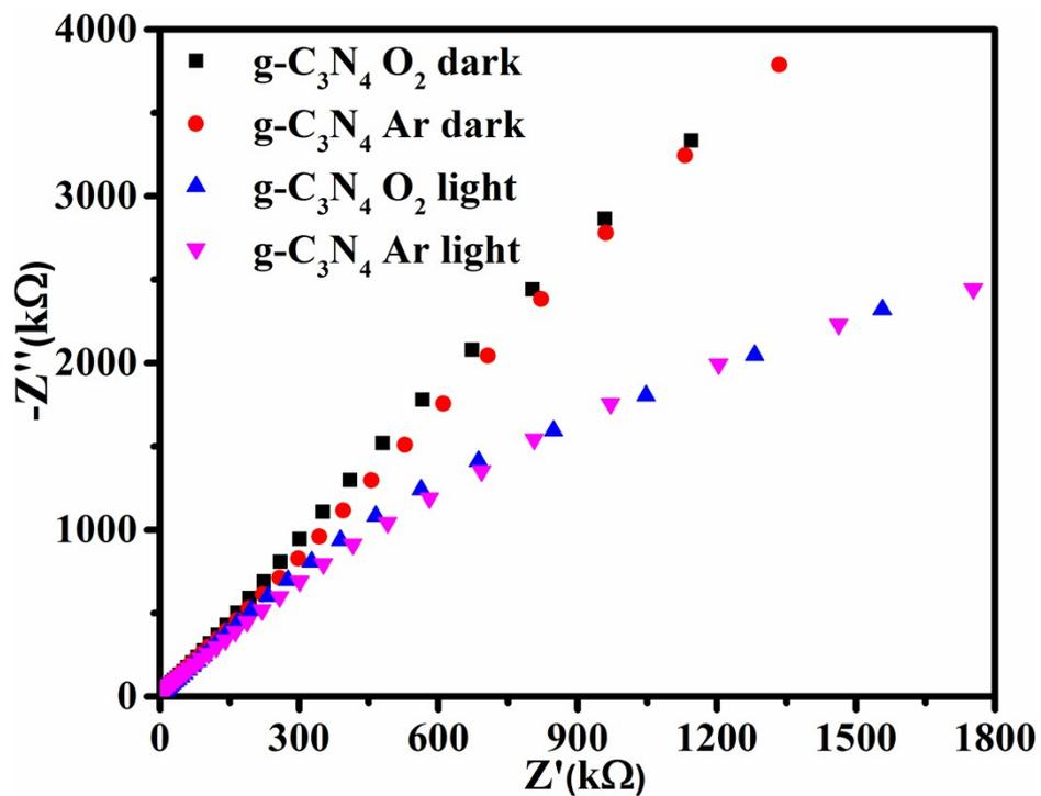
Fig. S24 Electrochemical impedance spectroscopy Nyquist plots of  $g\text{-C}_3\text{N}_4$  with saturated Ar or  $\text{O}_2$  atmosphere.
