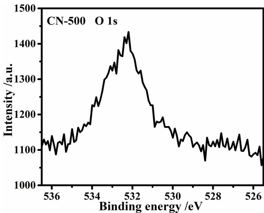
Fig. S15 O 1s high-resolution XPS spectra of g-C<sub>3</sub>N<sub>4</sub>.
