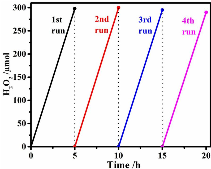
Fig. S20 The photocatalytic generation of H<sub>2</sub>O<sub>2</sub> by OCN-500 for four times with 10% isopropyl alcohol under visible light irradiation.
