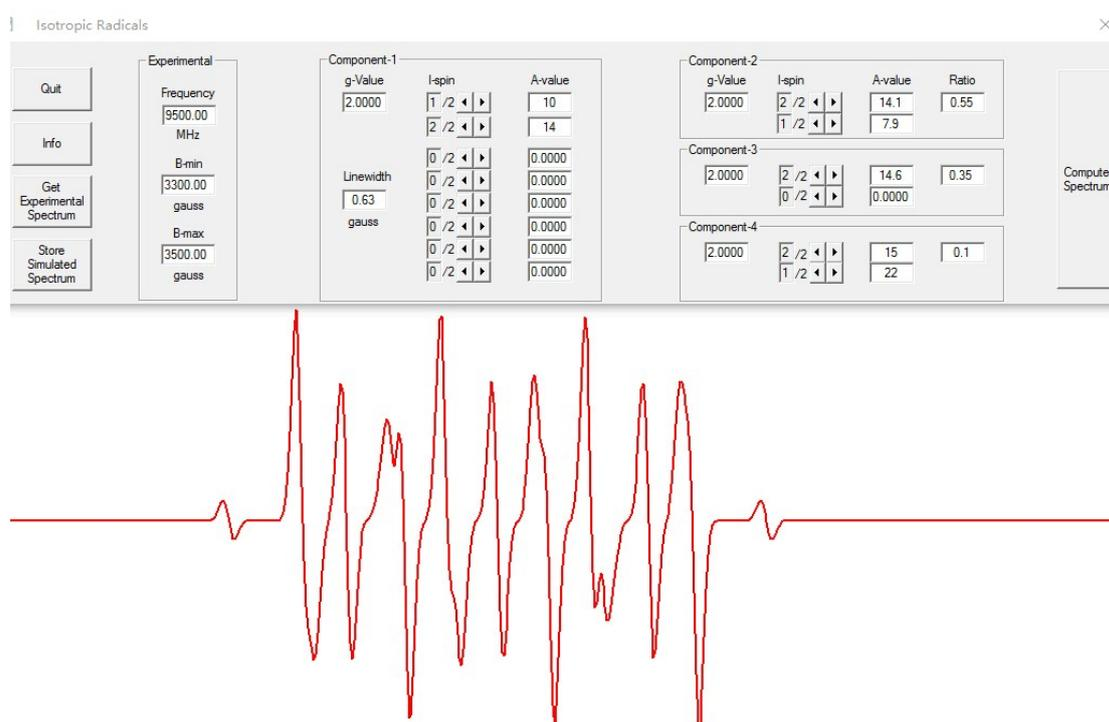
Fig. S29. The simulation ESR spectra of OCN-500 under visible light irradiation by the “Isotropic Radicals” software.
