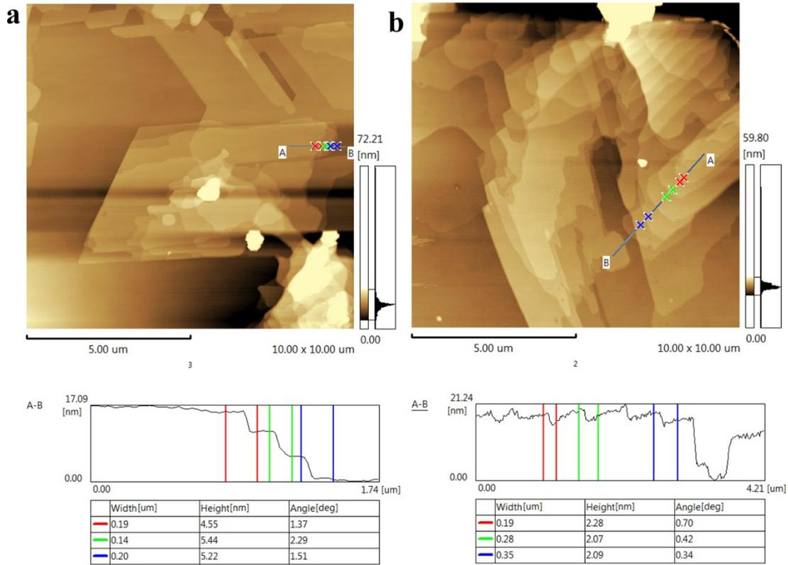
Fig. S10 AFM images of g-C<sub>3</sub>N<sub>4</sub> (a) and OCN-500 (b).
