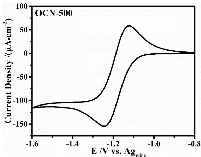
Fig. 28 Cyclic voltammetry for OCN-500 in acetonitrile solution. Experiment conditions: 0.1 M TBAP (tetra-*n*-butylammonium perchlorate), scan rates 10 mV/s, A silver wire was used as a reference electrode. All solutions were thoroughly degassed with  $\text{N}_2$  before each experiment, and an inert atmosphere was maintained during the experiments.
