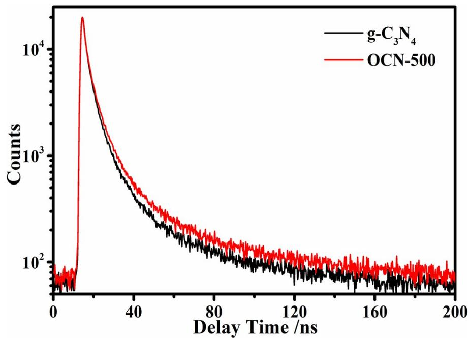
Fig. S25. Room temperature time-resolved transient photoluminescence decays spectroscopy for OCN-500 and  $g\text{-C}_3\text{N}_4$ , excited at 360 nm.
