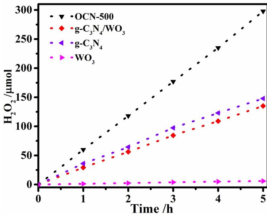
Fig. S26. The photocatalytic generation of H<sub>2</sub>O<sub>2</sub> with 10% isopropyl alcohol under visible light irradiation. (g-C<sub>3</sub>N<sub>4</sub>/WO<sub>3</sub>: g-C<sub>3</sub>N<sub>4</sub> and WO<sub>3</sub> are ground and mixed according to the ratio of carbon nitride and tungsten in OCN-500)
