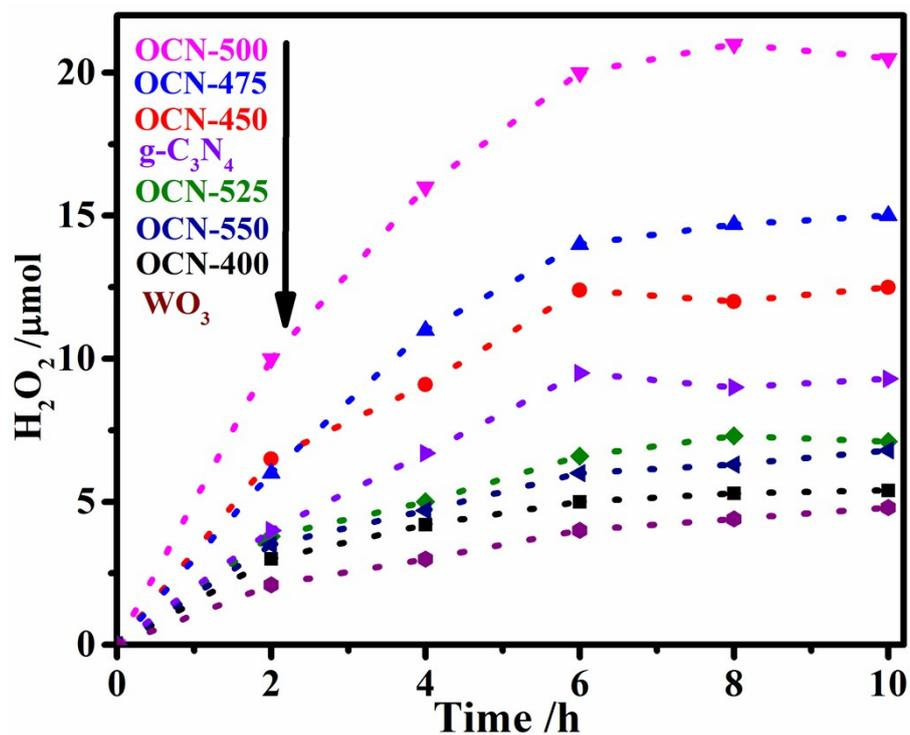
Fig. S17 The photocatalytic generation of H<sub>2</sub>O<sub>2</sub> in pure water under visible light irradiation with air atmosphere.
