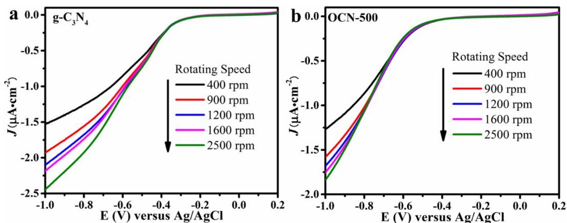
Fig. S27. LSV curves of  $g\text{-C}_3\text{N}_4$  (a) and OCN-500 (b) measured on RDE analysis at different rotating speeds.
