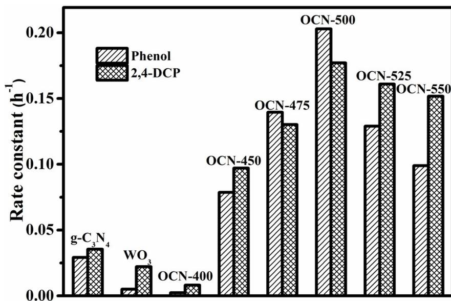
Fig. S22 Photocatalytic degradation of phenol and 2,4-DCP by different samples under visible light irradiation.
