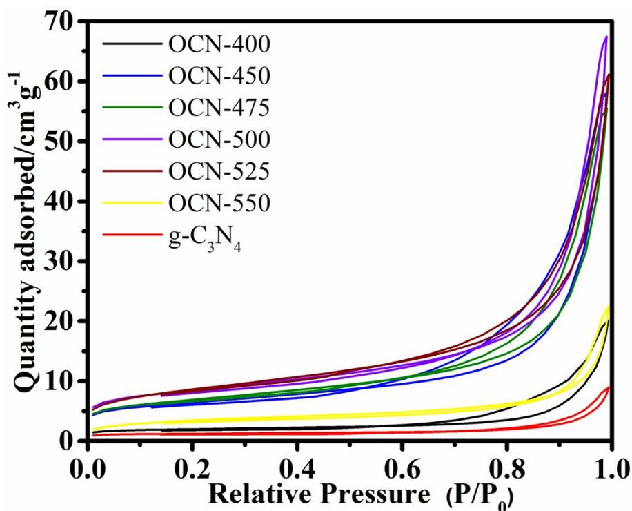
Fig. S5 N<sub>2</sub> adsorption–desorption isotherms of different samples.
