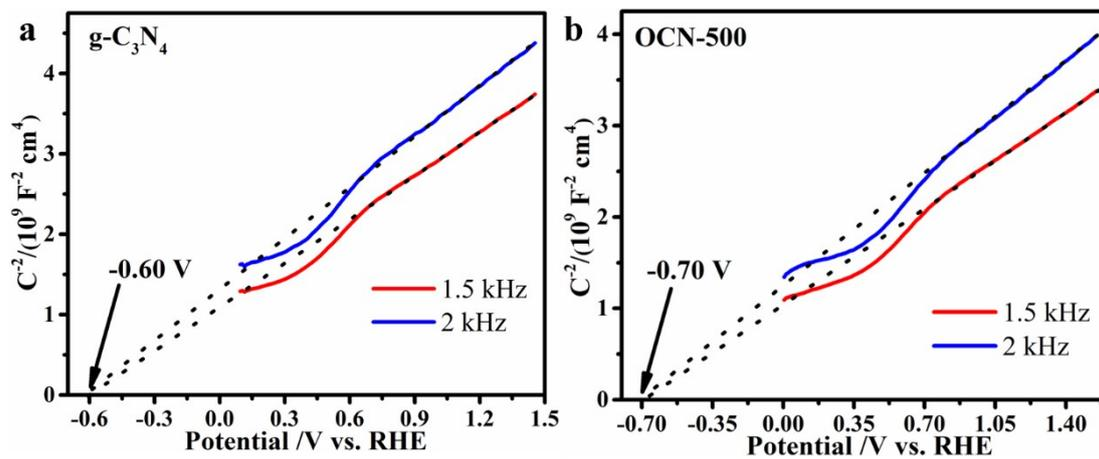
Fig. S12 Electrochemical Mott-Schottky curves of  $g\text{-C}_3\text{N}_4$  (a) and OCN-500 (b).
