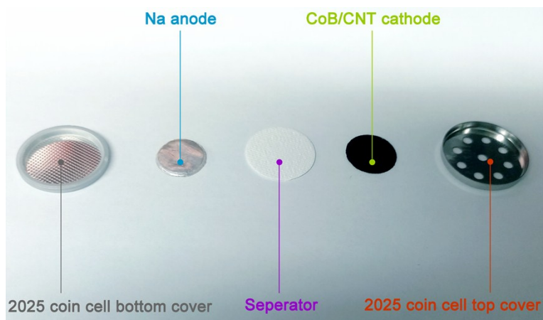
Fig. S22 Photograph of modified 2025-type coin cell used in Na-O 2 batteries.
