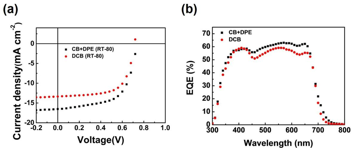
**Figure S1.** *J-V* characteristics of PPDT2FBT:PC<sub>71</sub>BM-based inverted PSCs with different solvents at a head temperature of 25 °C and substrate temperature of 80 °C (H25-S80).
