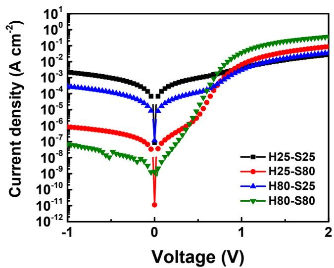
**Figure S5.** Dark  $J$ - $V$  characteristics of devices processed at various temperature combination conditions.
