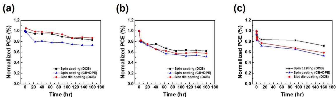
**Figure S2.** (a) long-term device stabilities in air, (b) thermal stabilities at 120 °C in N<sub>2</sub> filled glove box and (c) photo stabilities under AM 1.5G illumination in air. The photoactive layer of PSCs were spin-coated with and without additives, and also slot die coated for comparisons of devices durability. The devices used for stability testing were encapsulated in glass.
