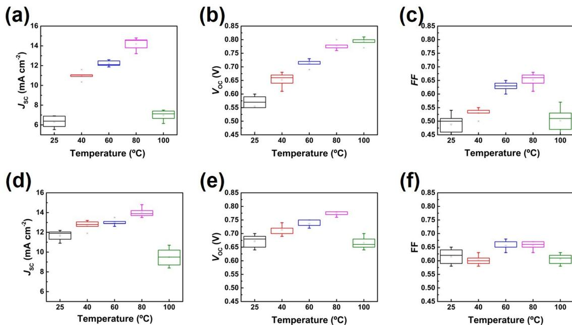
**Figure S3.** (a-c)  $J_{sc}$ ,  $V_{oc}$  and FF, respectively, of devices processed at different substrate temperatures at a fixed slot head temperature of 80 °C. (d-f)  $J_{sc}$ ,  $V_{oc}$  and FF, respectively, of devices processed at different slot head temperatures at a fixed substrate temperature of 80 °C. Each data point and the associated error bars represent the mean value and standard deviation, respectively.
