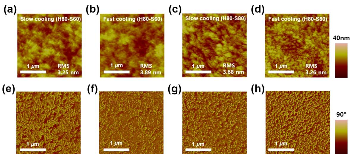
**Figure S8.** AFM topography (a-d) and corresponding phase images (e-h) for comparison of film morphologies dried by fast and slow cooling after slot die coating at H80-S60 and H80-S80.
