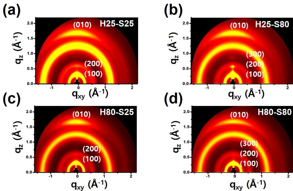
**Figure S6.** Two-dimensional GIWAXS data for films processed at (a) H25-S25, (b) H25-S80, (c) H80-S25 and (d) H80-S80 conditions, respectively.
