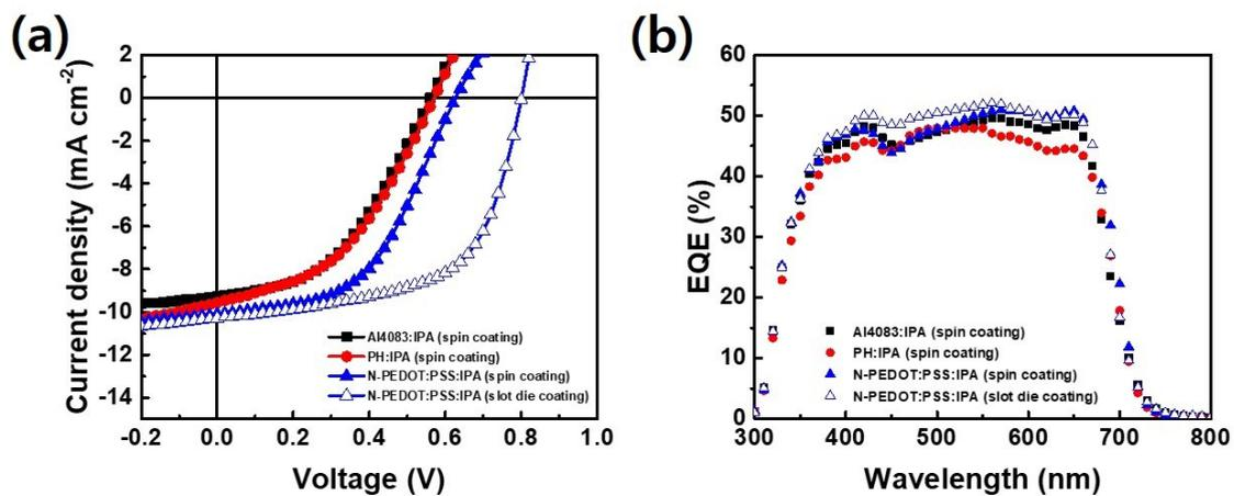
**Figure S11.** *J-V* characteristics and EQE results of PSCs fabricated by slot die-based all-solution process except electrodes.
