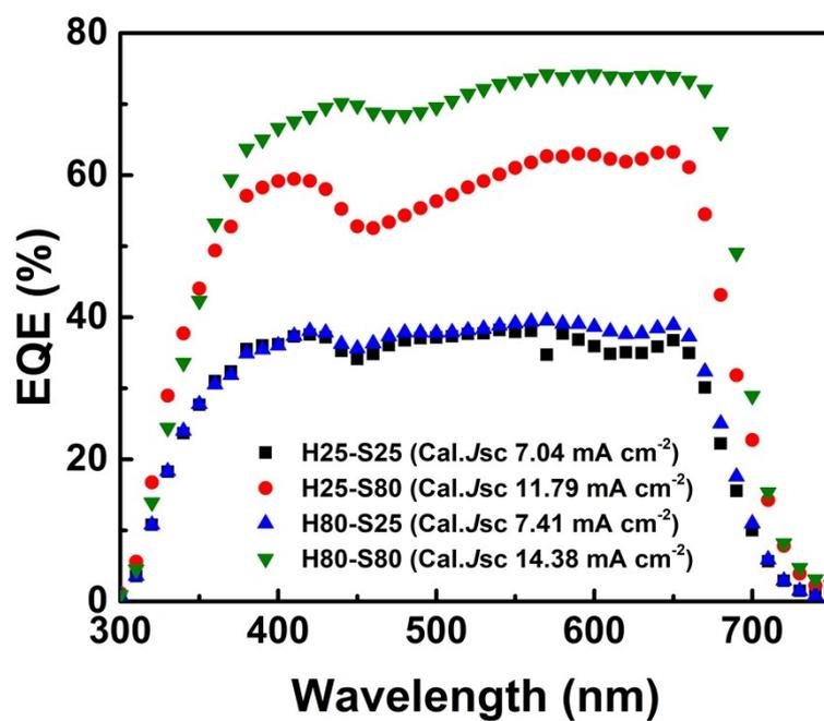
**Figure S4.** EQE spectra with varying thermal treatment conditions.
