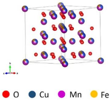
**Figure S9:**  $\text{CuMn}_{1.5}\text{Fe}_{0.5}\text{O}_4$  spinel structure.
