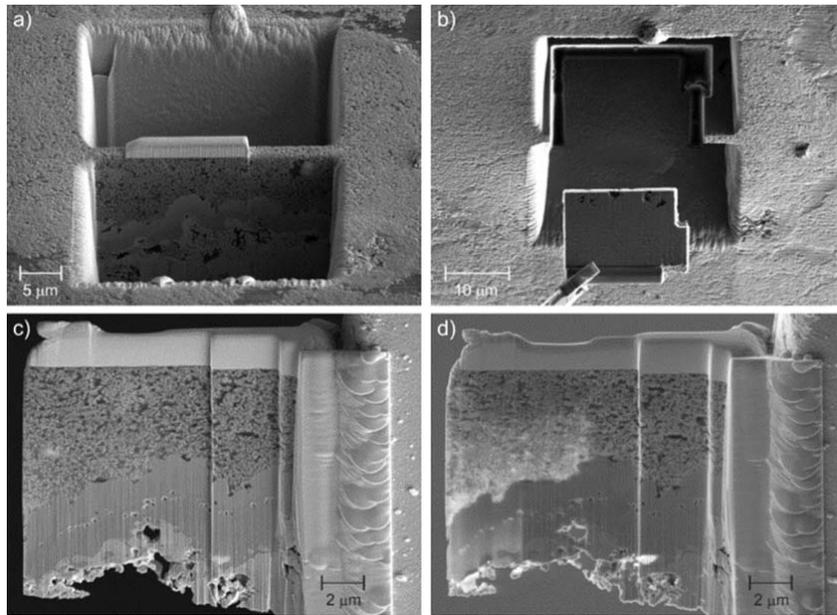
**Figure S6:** FIB lamella TEM sample preparation: a) FIB lamella bulk milling, b) rough lamella lift out, c) sequential lamella thinning using high-energy focused ion beam, d) thinned lamella polishing using low-energy focused ion beam.
