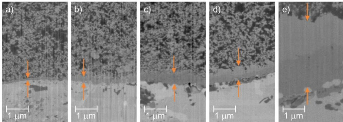
**Figure S5:** FIB-SEM cross-sectional image of oxide-layer formation on Inconel support material for the case of: a) Initial sample B444 [average 110 nm], b) sample b1  $\Delta T_1$ /12 weeks (620 cycles) [average 320 nm], c) sample b1  $\Delta T_1$ /24 weeks (1142 cycles) [average 590 nm], d) sample 750/2 weeks [average 670 nm], e) sample 770/14 weeks [average 3,1  $\mu\text{m}$ ].
