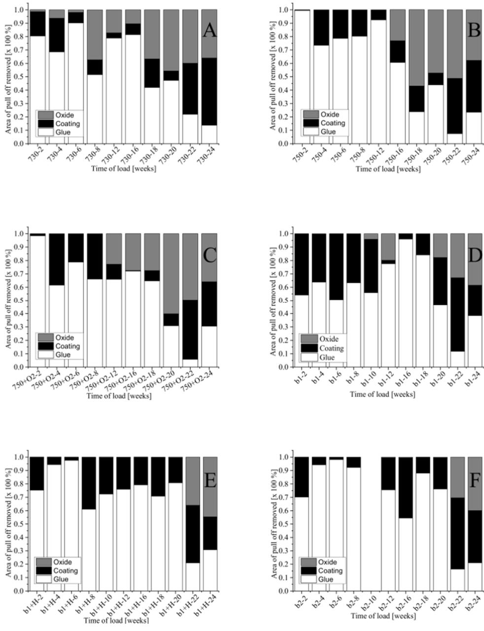
**Figure S3:** Ratio of areas for three different species (oxide, coating, glue) after pull-off testing vs. isothermal loading time at 730 °C (A), 750 °C (B), 750 °C + O<sub>2</sub> (C), b1 ΔT<sub>1</sub> (D), b1+H ΔT<sub>1</sub> (E) and b2 ΔT<sub>1</sub> (F).
