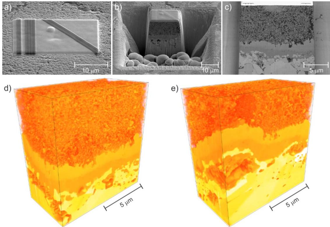
**Figure S7:** FIB 3D analysis of sample 770-14W: a) fabrication of Pt protective layer with embedded reference markers, b) U-Shaped region of interest preparation by FIB milling, c) Z-contrast cross-sectional SEM image of the first acquired slice-image, d) three-dimensional sample visualization using volume rendering (front view), e) three-dimensional sample visualization using volume rendering (back view).
