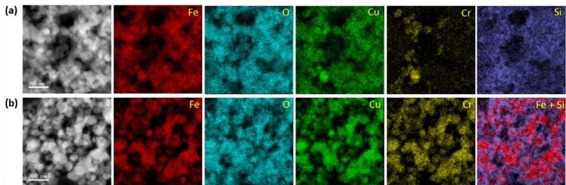
**Figure S8:** (a) EDX elemental maps acquired from the mid-section of the B444 coating, where Cr segregation is observed: only some particles imaged on the mapped area show a Cr signal. (b) EDX elemental maps acquired from a section of the B444 coating located very close to the interface with the oxide layer. The Cr signal, in this case, is uniformly distributed along the particles. To visualize the Si coating on the particles, a compositional map of Fe and Si is displayed as well .
