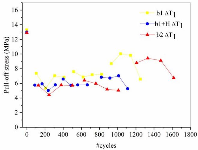
**Figure S4:** Pull-off stress as a function of the loading time for a cyclic load.
