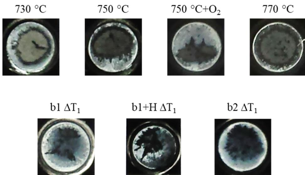
**Figure S1:** Photograph of the testing surface by pull-off test after 18 weeks of different thermal loads.
