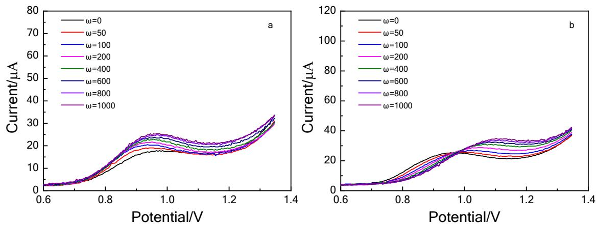
Fig. S2. Linear sweep curves of different blank water matrixes on GC RDE. a) Lake Water; b) Secondary Effluent. Background electrolyte: 0.01 M phosphate buffer, pH=7; scan rate: 100 mV s<sup>-1</sup>.
