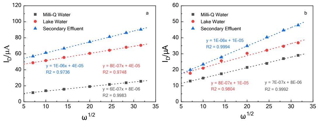
Fig. S3. Linear fitting plot of  $I_D-\omega^{1/2}$  of  $10^{-4}$  M CPX in different water matrixes on GC RDE. a) without deducting of blank values; b) blank values deducted. Background electrolyte: 0.01 M phosphate buffer, pH=7; scan rate:  $100 \text{ mV s}^{-1}$ .
