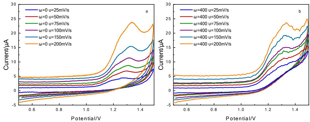
Fig.S4. Cyclic voltammetry curves of CPX at various scan rates on GC RDE with rotating speed of a) 0 and b) 400, respectively. CPX concentration: 10  $\mu$ M; background solution: 0.01 M phosphate buffer, pH=2.
